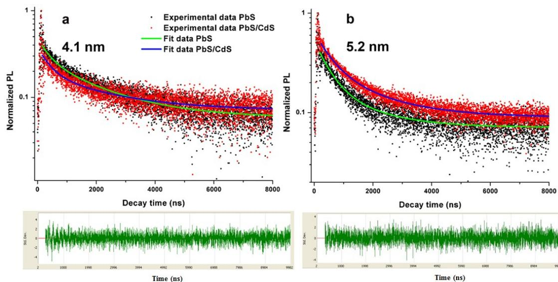
Figure S5. Typical PL decay curves of PbS and PbS/CdS QDs of different size (a: 4.1 nm, b: 5.2 nm) and corresponding residuals of the fittings for PbS/CdS QDs.
