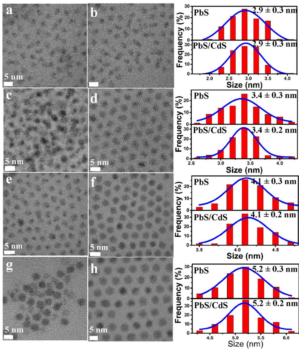
Figure S2. TEM images of differently sized PbS (a:  $2.9 \pm 0.3$  nm, c:  $3.4 \pm 0.3$  nm, e:  $4.1 \pm 0.3$  nm, g:  $5.2 \pm 0.3$  nm) and PbS/CdS (b:  $2.9 \pm 0.3$ , d:  $3.4 \pm 0.2$  nm, f:  $4.1 \pm 0.2$  nm, h:  $5.2 \pm 0.2$  nm) QDs and their corresponding histograms (right).
