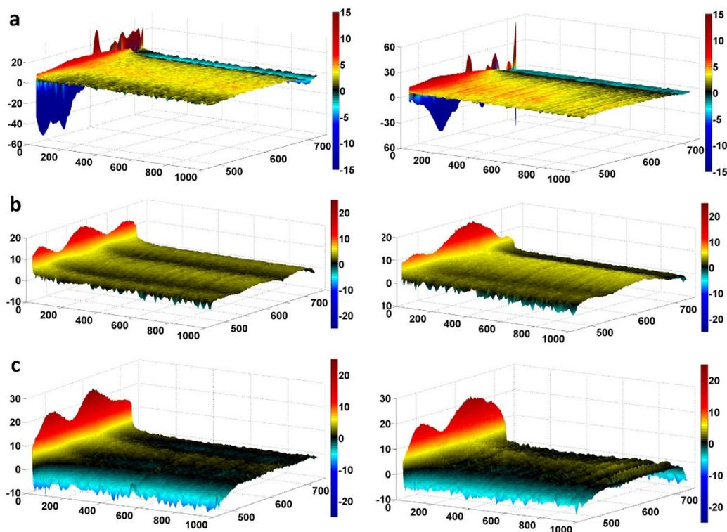
Figure S7. 3D transient absorption difference absorption spectra of PbS (left) and PbS/CdS (right) of different particle size a: 2.9 nm, b: 4.4 nm, c: 6 nm at probe wavelengths spanning 480 – 720 nm after 750 nm, 2.5  $\mu\text{J}$ /pulse excitation.
