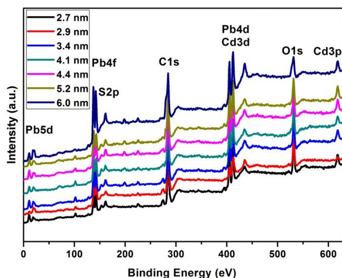
Figure S1. XPS survey spectrum of PbS/CdS core/shell QDs.
