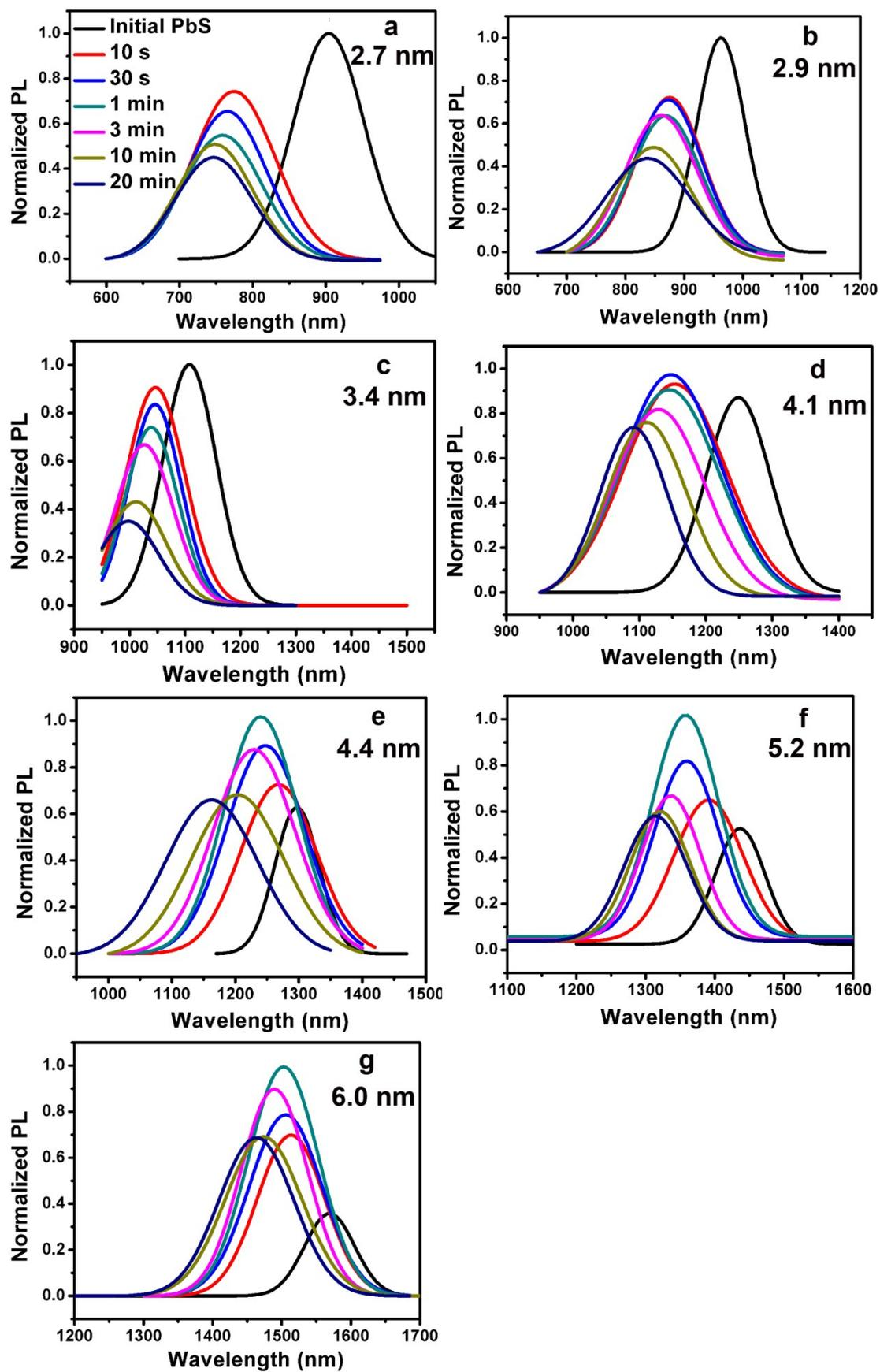
Figure S3. PL spectra of differently sized PbS QDs and PbS/CdS core/shell QDs synthesized by microwave-assisted cation exchange at different reaction time.
