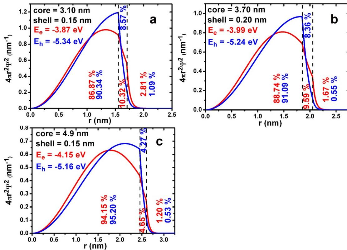
Figure S6. The energies for electrons and holes of differently sized PbS/CdS QDs (a: 3.4 nm, b: 4.1 nm, c: 5.2 nm) and the probability of finding them in each of the 3 regions (core, shell, outside).
