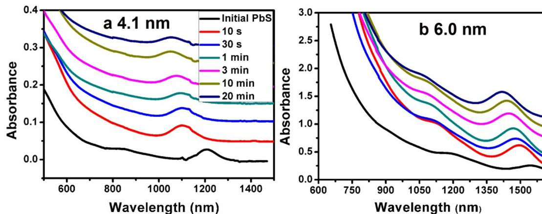
Figure S4. Typical absorption spectra evolution of QDs during microwave-assisted cation exchange (a: 4.1 nm, b: 6 nm).
