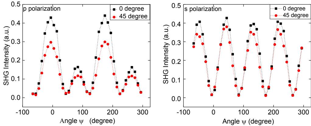
**Figure S1 (a):**  $p$ - and  $s$ - polarization data from a FF-MNT at  $45^\circ$  and  $0^\circ$  degree. There is a slight change in the SHG intensity due to the Fresnel coefficients of fundamental and SHG waves.
