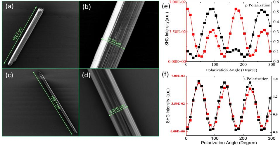
**Figure S3:** (a) and (b) are the SEM images from a FF-MNT with O.D. = 13.2  $\mu\text{m}$ . (c) and (d) are SEM images from a FF-MNT with O.D. = 5.8  $\mu\text{m}$ . (e) and (f) p-polarization and s-polarization SHG from the two tubes. The red curve represents the FF-NT with O.D. = 5.8  $\mu\text{m}$  and the black curve represents the FF-MNT with O.D. = 13.2  $\mu\text{m}$
