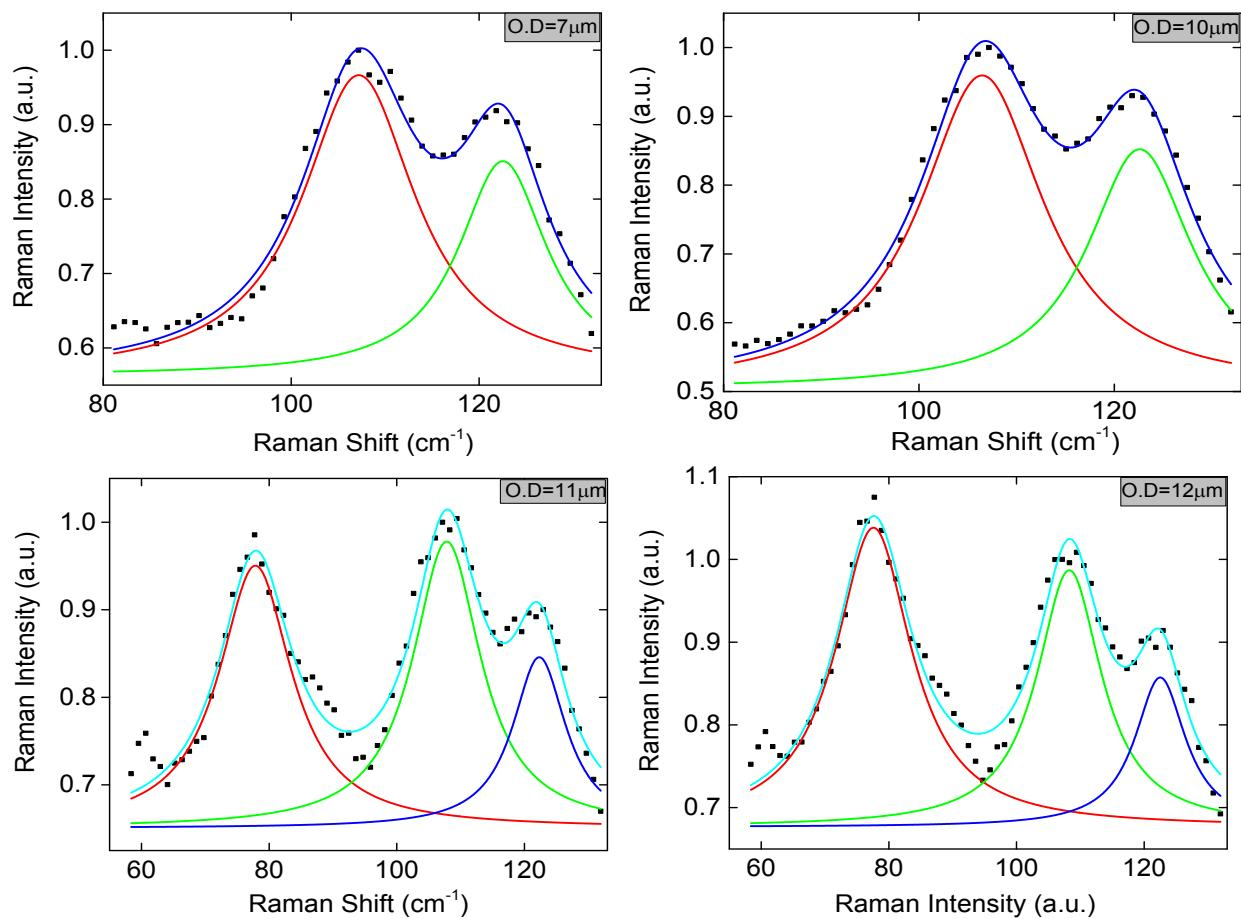
**Figure S6:** Peak fit of Raman scattering from individual FF-MNTs with varying O.D.s.
