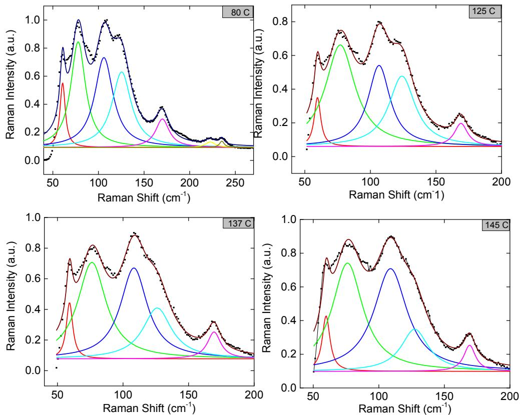
**Figure S6:** Peak fit of Raman spectra from FF-MNT (O.D. = 11  $\mu\text{m}$ ) at different annealing temperatures. Annealing the tube beyond 145 °C results in the orthorhombic phase.
