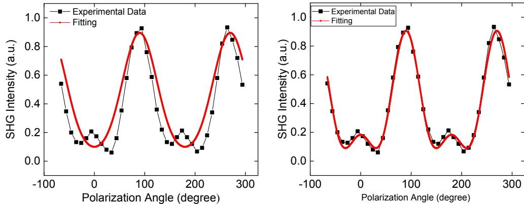
**Figure S1 (b):**  $p$ -polarization data at  $0^\circ$  degree fit with  $d_{31}$  and  $d_{33}$  having the same sign (left) and opposite sign (right).
