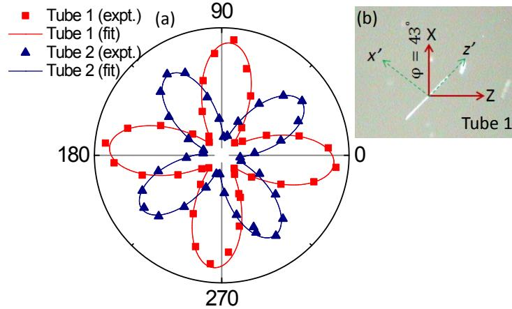
**Figure S2.** (a) Symbols are the experimental  $s$  polarization SHG data for two tube orientation. The solid lines are a fit to the square of Eq. (3 a). (b) Optical image of FF-MNT (Tube 1) (in white) where the angle was measured as  $43^\circ$  with respect to the laboratory frame of reference. For tube 2, the measured angle was  $169^\circ$ .
