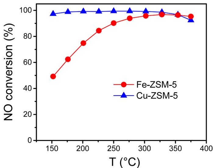
Fig. S8 Measured conversion of NO in the  $\text{NH}_3$ -SCR tests over Fe-ZSM-5 and Cu-ZSM-5. The Testing conditions: 0.5 g catalyst; a total flow rate of  $1 \text{ L min}^{-1}$ ; 500 ppm  $\text{NH}_3$ , 500 ppm NO, 10%  $\text{O}_2$ , 2%  $\text{H}_2\text{O}$ .
