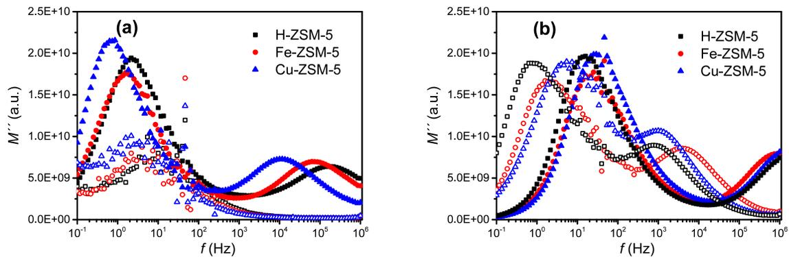
Fig. S3 Modulus plots of the *in situ* IS results in pure N<sub>2</sub> (empty symbols) and 100 ppm NH<sub>3</sub> in N<sub>2</sub> (solid symbols) at 100 °C (a) and 250 °C (b). H-ZSM-5: black squares; Fe-ZSM-5: red circles; Cu-ZSM-5: blue triangles.
