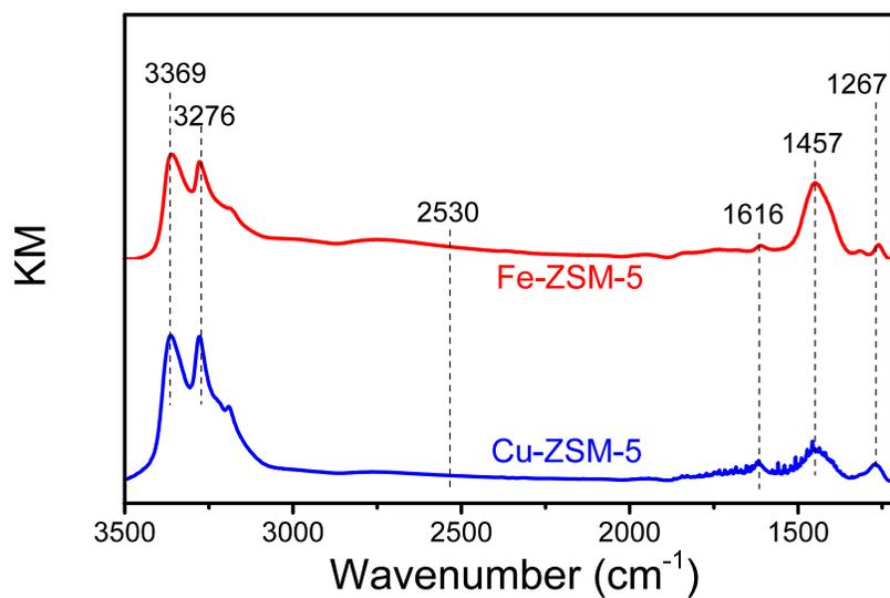
Fig. S6 DRIFT spectra taken over zeolites after  $\text{NH}_3$  saturation at 250 °C.
