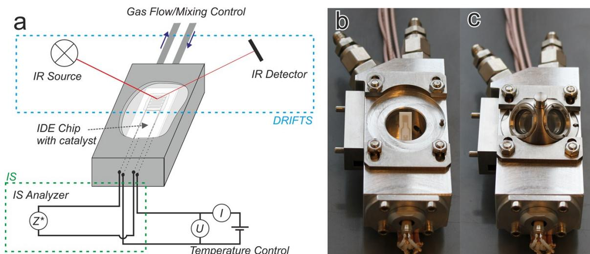
**Fig. S1** Simultaneous *in situ* IS-DRIFTS measurements on the same catalyst film. (a) Scheme of the chamber and measurement configuration; (b) Photograph of open chamber; (c) Photograph of chamber with dome. Adapted from Ref 3.
