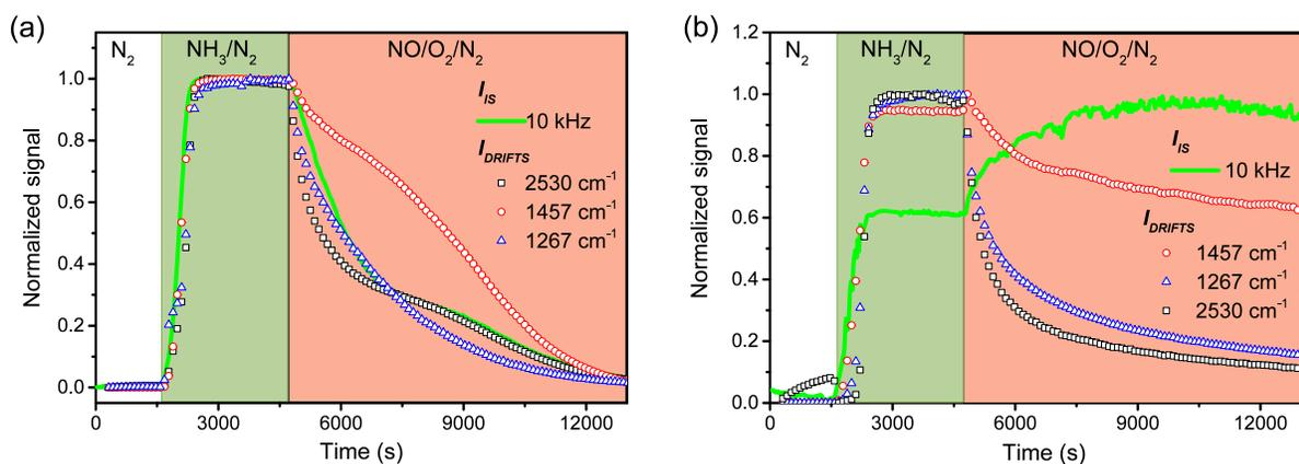
Fig. S9 Time-course of normalized  $I_{IS}$  and  $I_{DRIFTS}$  signals (normalized by setting the smallest value to 0 and the highest value to 1) for Fe-ZSM-5 (a) and Cu-ZSM-5 (b) during exposure to the indicated atmospheres at  $100 \text{ }^\circ\text{C}$ . Fig. S9b is part of a submitted manuscript.
