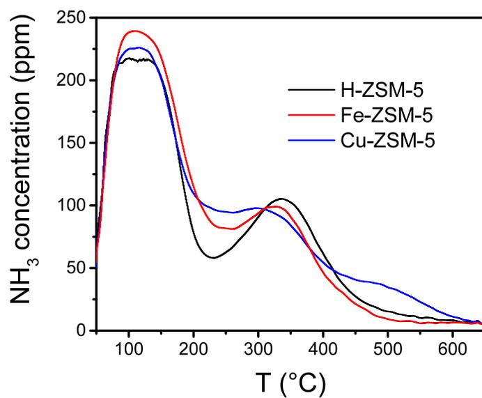
Fig. S2 NH<sub>3</sub> desorption profiles of the zeolite catalysts in NH<sub>3</sub>-TPD at a heating ramp of 2 °C min<sup>-1</sup>.
