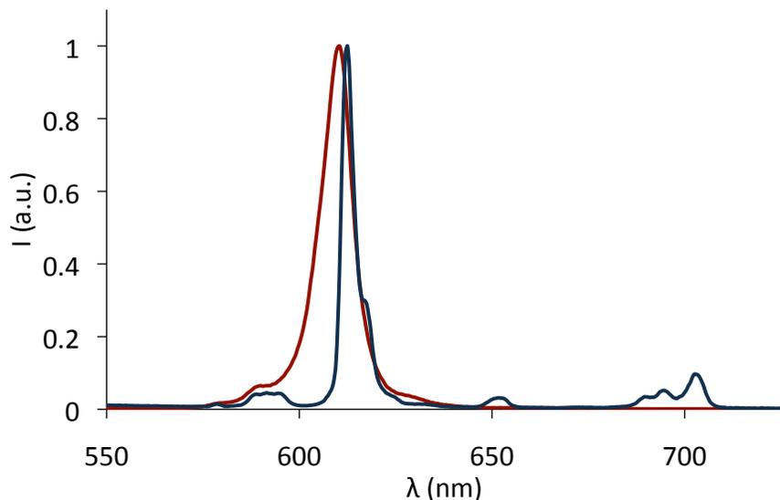
**Figure S1.** Normalized steady-state emission spectra ( $\lambda_{\text{exc}} = 345 \text{ nm}$ ) of  $\text{Eu}^{\text{III}}$  (blue) and  $\text{Cm}^{\text{III}}$  (red) complexes formed in situ with **2**, in 0.1 M HEPES buffer (pH 7.4, 25°C,  $[\text{M}^{\text{III}}] = [\mathbf{2}] = 10 \mu\text{M}$ ).
