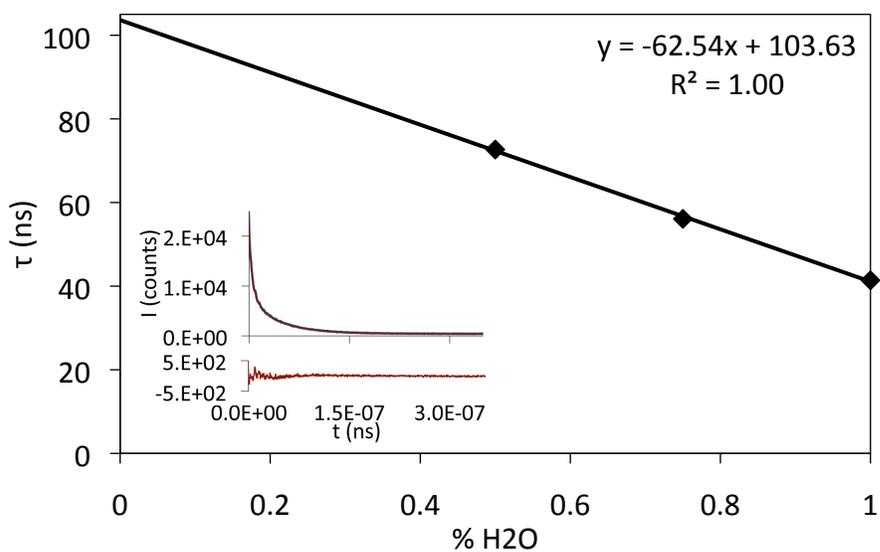
**Figure S2.**  $\text{Am}^{\text{III}}$  luminescence lifetime determination as a function of % $\text{H}_2\text{O}$  content in  $\text{D}_2\text{O}:\text{H}_2\text{O}$  mixtures for  $[\text{Am}^{\text{III}}(\mathbf{1})]^-$  (10  $\mu\text{M}$  in 0.1 M HEPES, pH 7.4, 25°C). **Inset:** Luminescence decay of  $[\text{Am}^{\text{III}}(\mathbf{1})]^-$  (blue) in  $\text{H}_2\text{O}$  with the fitted curve (red) and its residual.
