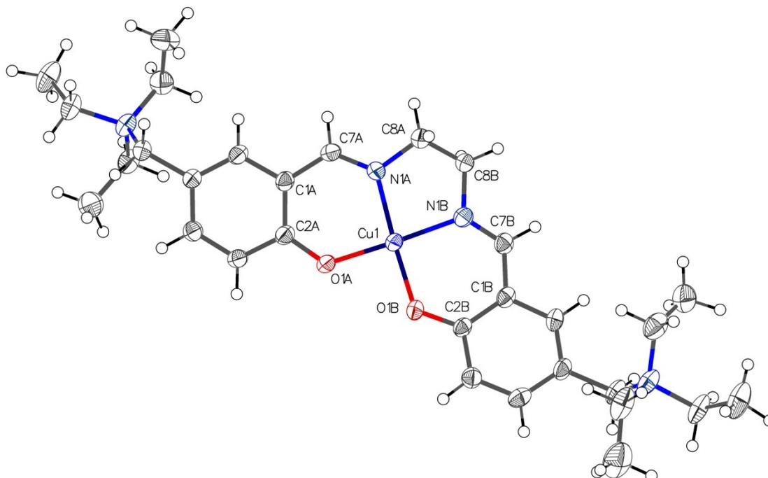
**Figure S3.** Asymmetric Unit of **2**, drawn with 50% displacement ellipsoids. Perchlorate omitted for clarity. The single bond between C8A C8B is arranged as “gauche” conformer (44.053(7)°). It was necessary to mask (by Olex2) one void because no adequate solution could be found. The volume of this void is 179.6 [Å<sup>3</sup>] and the number of excluded electrons is 29.4. Both hkl-Files (original and masked) are uploaded to the CCDC.
