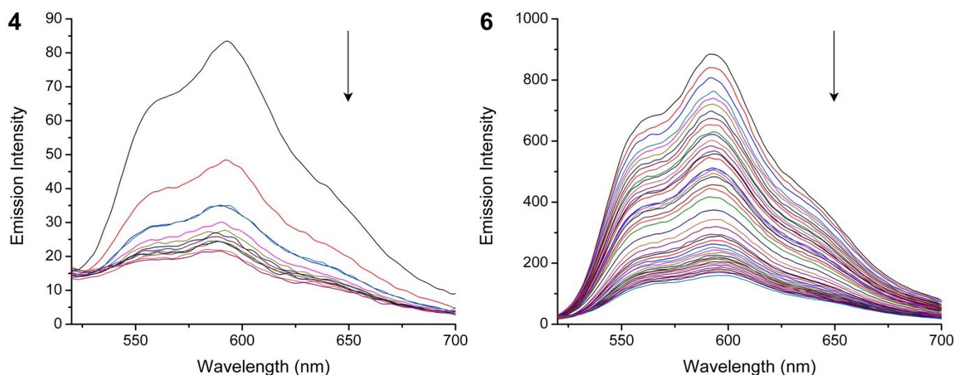
**Figure 2.** Emission spectra (510-700 nm) of **4** at 0.7  $\mu\text{M}$  and **6** at 2.8  $\mu\text{M}$  in PBS buffer (10 mM, pH 7.48) with NaCl (50 mM). The initial fluorescence is quenched upon incremental addition of ctDNA.
