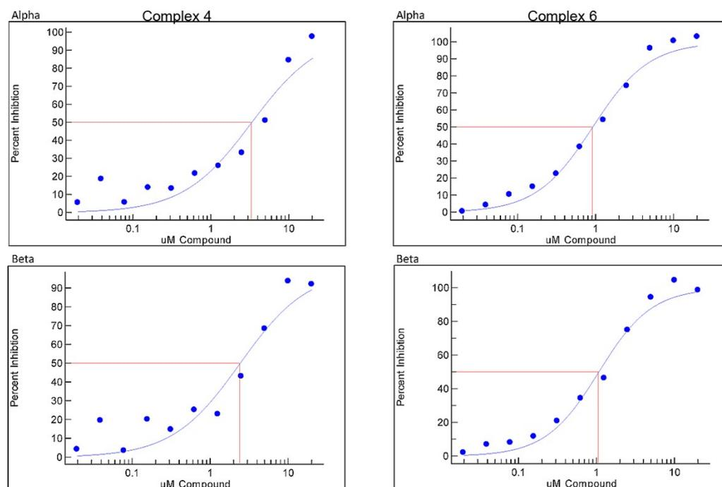
**Figure 4.** Concentration-dependent inhibition of hTOPOII  $\alpha$  and  $\beta$  by complexes 4 (left) and 6 (right). Blue dots represent measured values according to equation (5), the blue line represents a non-linear least squares fit to equation (6) and the red drop-lines indicate the  $IC_{50}$  values.
