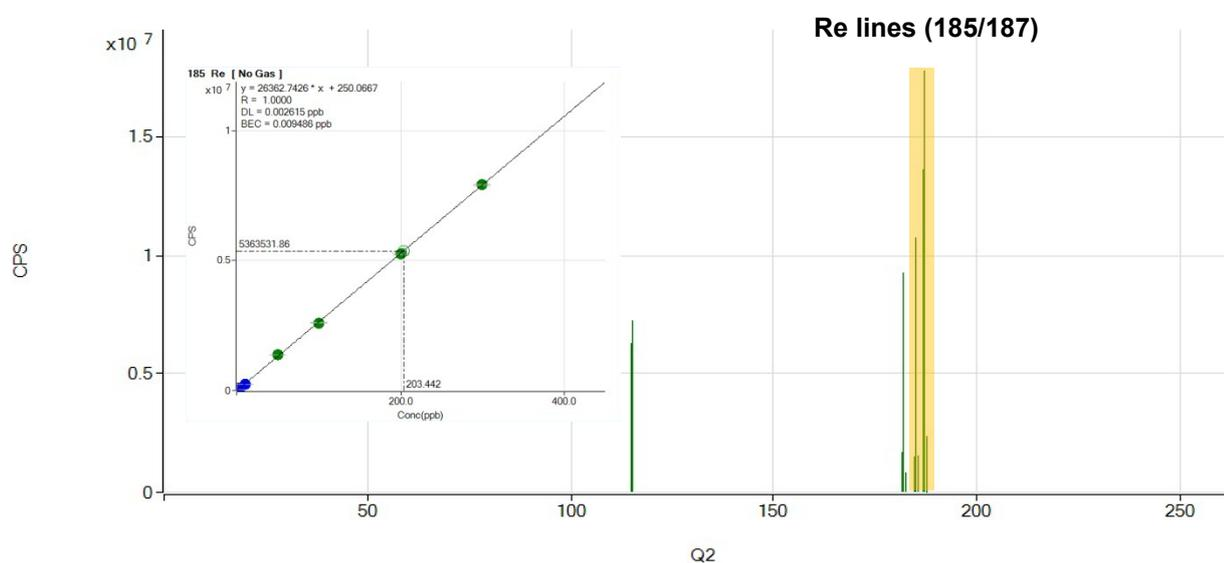
**Figure 1.** Example of the rhenium lines observed during ICP-MS measurements. Inset: Calibration curve of the actual measurements. Detection limit (DL): 2.6 ppt, background equivalent concentration (BEC): 9.4 ppt.
