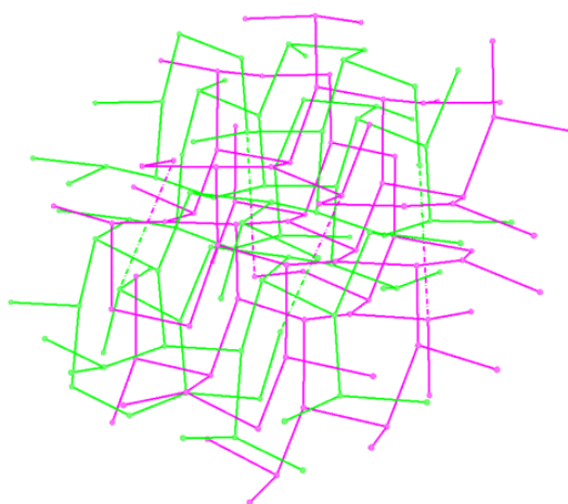
Figure S20 The underlying net of the three-dimensional coordination polymer 13 . Interpenetrating utp nets are shown in green and fuchsia, and the connections by Ag(2) atoms are depicted with dashed lines.
