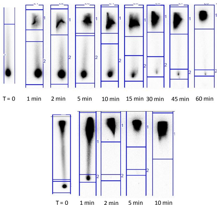
**Figure S2.** TLC analyses of  $^{89}\text{ZrL}^{1'}$  (top) and  $^{89}\text{ZrMe-AHA}$  (bottom) incubated in EDTA (10 mM, pH = 6) from 0 to 60 min, using EDTA (10 mM, pH = 6) as eluent.
