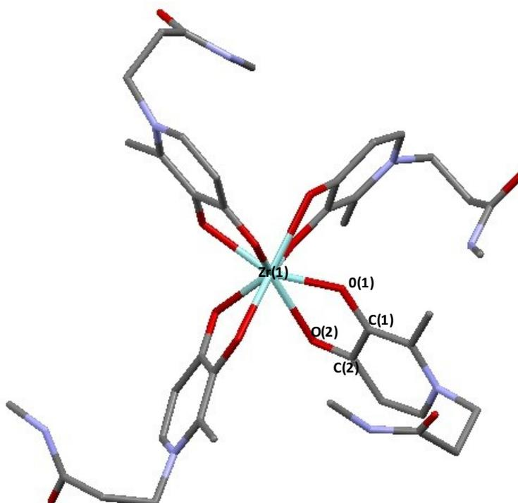
**Figure S4.** Calculated structure of  $\text{Zr}(\text{L}^3)_4$  in the reaction field of water at 298.15 K. Selected bond lengths ( $\text{\AA}$ ) and angles ( $^\circ$ ):  $\text{Zr1-O1}$ , 2.187;  $\text{Zr1-O2}$ , 2.335;  $\text{O1-Zr1-O1}$ , 69.98;  $\text{C1-O1-Zr1}$ , 120.29;  $\text{C2-O2-Zr1}$ , 115.75. Hydrogen atoms omitted for clarity.
