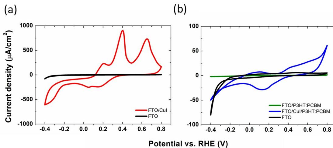
**Fig. S4.** Cyclic voltammety measurements on CuI deposited on top of FTO substrates and directly exposed to the electrolyte solution (panel a, red line), as compared to FTO/CuI/P3HT:PCBM samples (panel b, blue line). Control bare FTO and FTO/P3HT:PCBM devices (black and green solid lines, respectively) show almost no electrochemical activity within the considered potential range. Scan rate, 200 mV/s.
