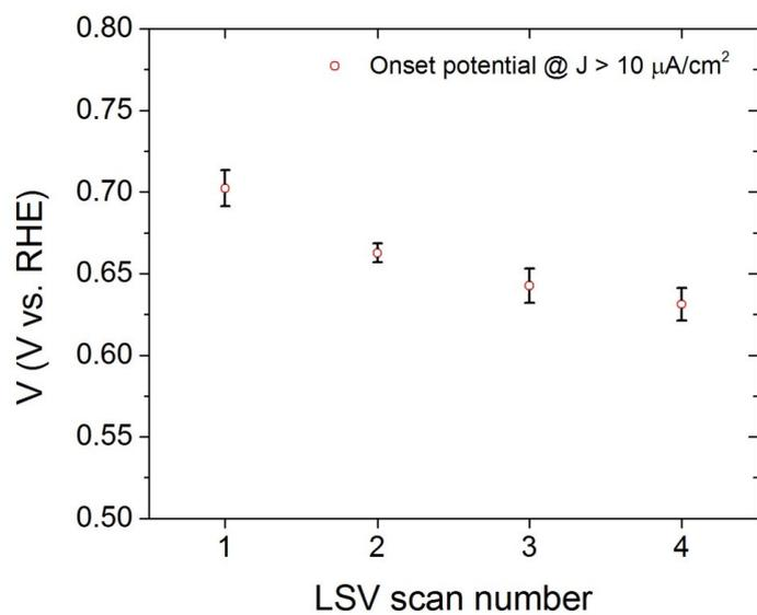
**Fig. S6.** Onset potentials (OP) for cathodic photocurrents higher than 10 μA/cm<sup>2</sup> during subsequent LSV scans of hybrid photocathodes at pH 1 and 1 sun illumination. Error bars represent the standard deviation of measurements over six different devices.
