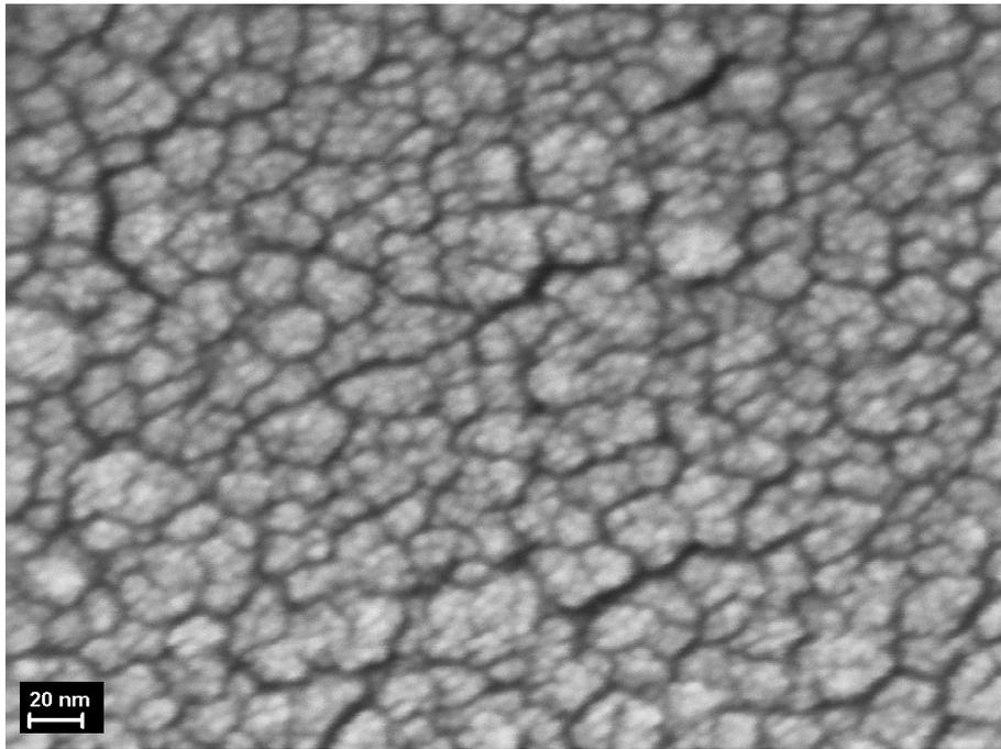
**Fig. S9.** HR-SEM of the surface (capping Pt layer on top of the nanostructured TiO<sub>2</sub>) of a hybrid photocathode after thermal annealing. The granular morphology at the top of TiO<sub>2</sub> layer are clearly visible (scale bar 20 nm).
