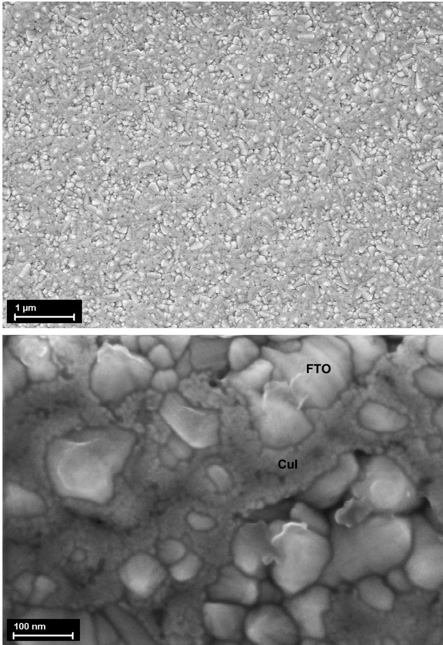
**Fig. S2.** SEM micrographs of a CuI layer (darker gray) deposited over the rough FTO substrate (brighter big crystals). Top: Long scale view of the surface (scale bar, 1  $\mu\text{m}$ ). Bottom: High resolution image showing a granular morphology with nanoparticles around 10 nm in size (scale bar, 100 nm).
