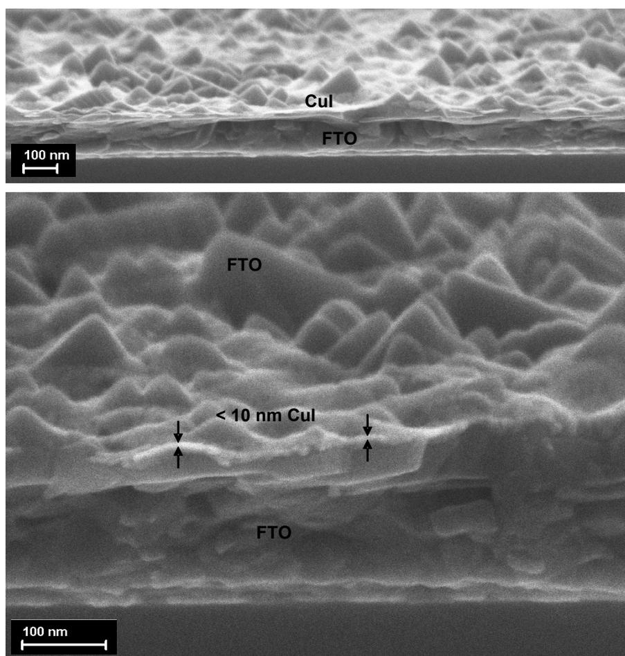
**Fig. S1.** Cross-sectional SEM of a CuI layer deposited over the rough FTO substrate. Top: Long scale view (scale bar, 100 nm). Bottom: High resolution image showing the thin layer of CuI (thickness around or below 10 nm) and the big FTO crystals (scale bar, 100 nm).
