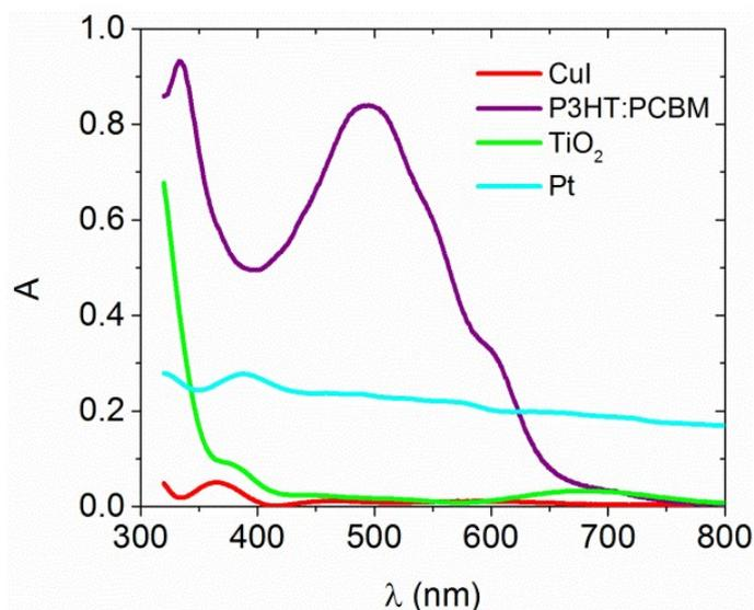
**Fig. S3.** Neat UV-visible absorption spectra of every layer present in the hybrid photocathode according to the architecture FTO/CuI/P3HT:PCBM/TiO<sub>2</sub>/Pt.
