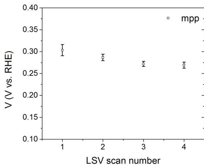
**Fig. S7.** Maximum power points (mpp) during subsequent LSV scans of hybrid photocathodes at pH 1 and 1 sun illumination. Error bars represent the standard deviation of measurements over six different devices.
