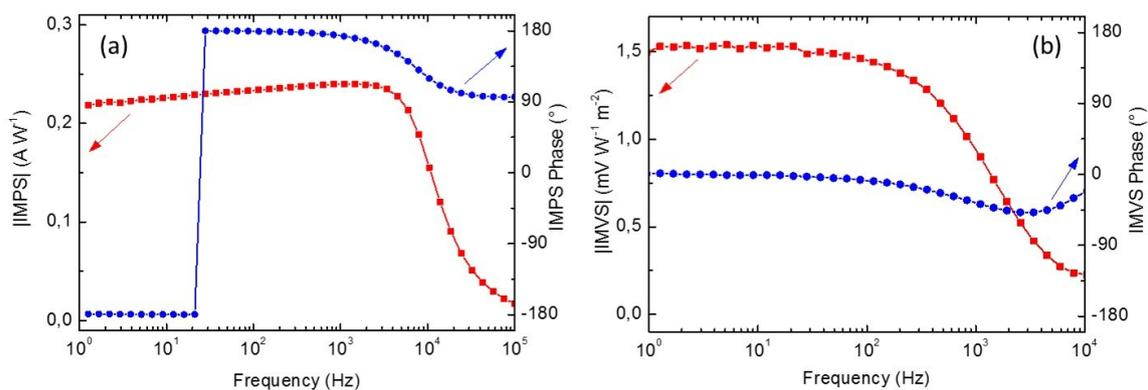
**Fig. S5** IMPS (a) and IMVS (b) Bode diagrams recorded at 0 V vs. RHE and at open circuit condition, respectively. A red and blue color traces represent module and phase, respectively.
