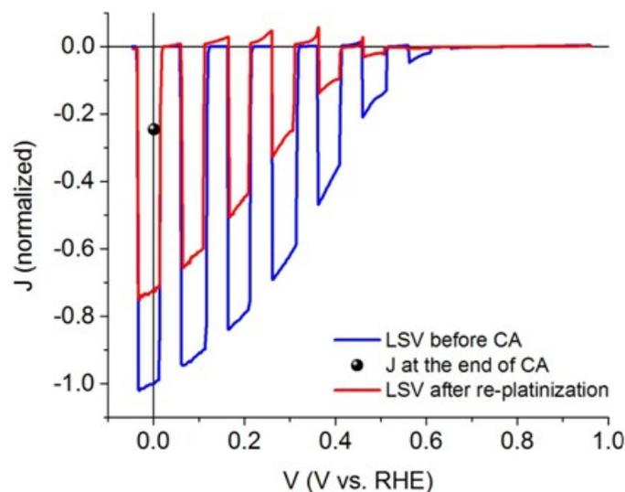
**Fig. S10.** Comparison between LSV scans before and after a second platinum deposition, on a photocathode undergoing one hour operation at 0 V and pH 1 electrolyte. The final photocurrent value at the end of the CA is identified by the black dot.
