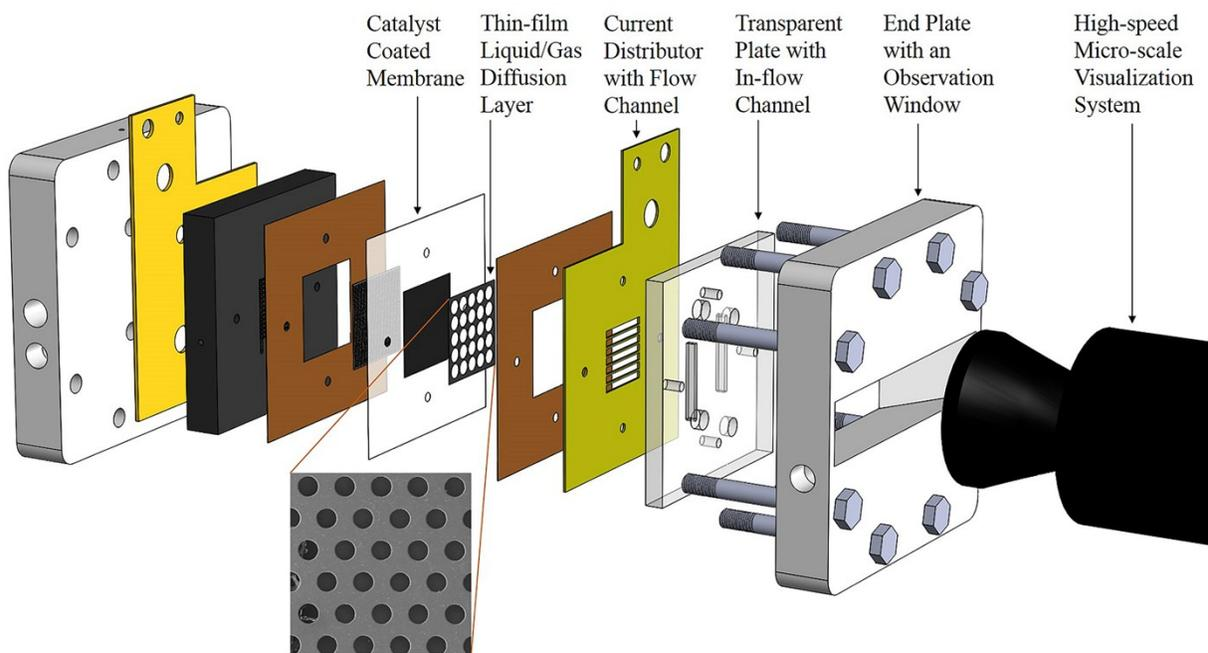
**Fig. S2** Schematic of high-speed micro-scale visualization system (HMVS) and transparent PEMEC with thin film/well tunable LGDL
