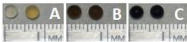
Figure S6. Chitosan hydrogel beads prepared in this study. (A) CS-PAA, (B) GO1 and (C) GO5 hydrogel beads have an average diameter of 3 mm.
