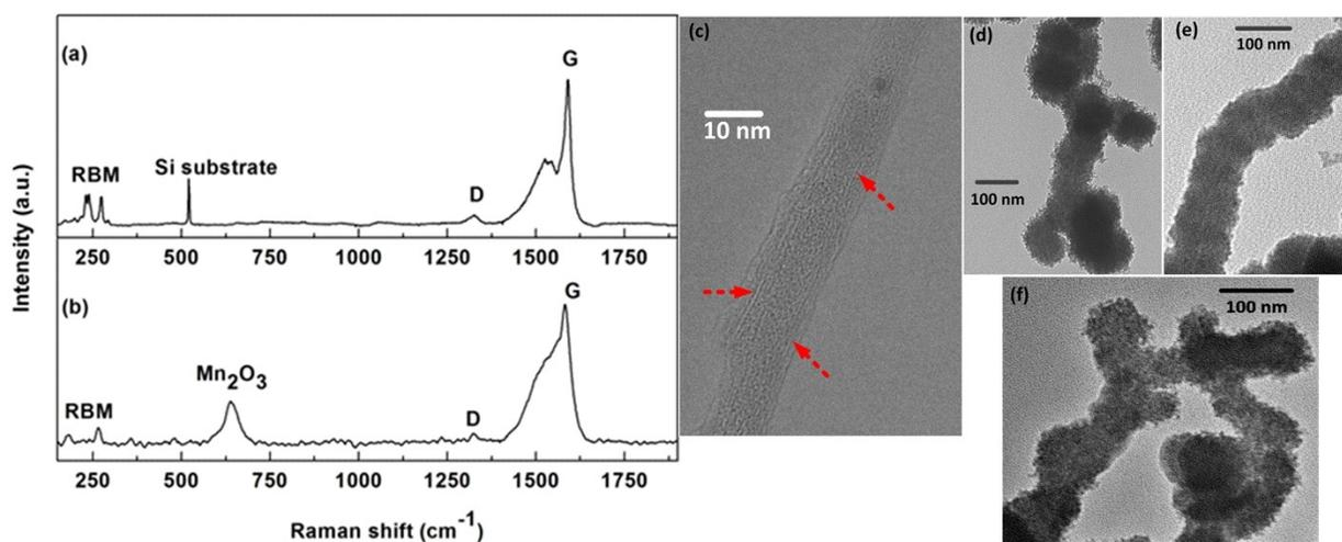
**Figure S1:** Raman spectra obtained from M13 virus-SWCNT complex on Si substrates (a) before and (b) after the mineralization. The spectra show the radial breathing modes (RBM), D-band, G-band confirming the presence of SWCNT in the material. TEM image of (c) M13-SWCNT complex (red arrow showing SWCNT on the virus), and the grown  $\text{MnO}_x$  on (d)&(e) M13 virus and (f) M13-SWCNT complex comparing the morphology of the material with and without SWCNT.
