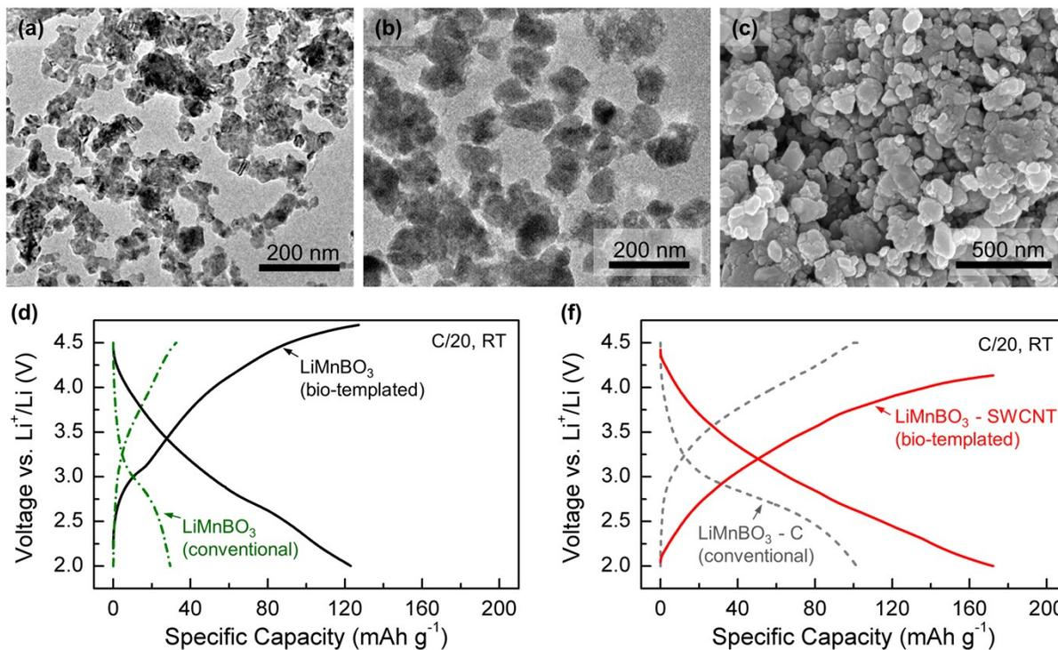
**Figure S2:** TEM images obtained from (a) bio-templated, also shown in Fig. 1g, and (b) conventionally synthesized  $LiMnBO_3$ , (c) an SEM image of conventionally synthesized  $LiMnBO_3$ , and voltage vs. specific capacity profiles of bio-templated and conventionally synthesized  $LiMnBO_3$  (d) without and (e) with conductive phase attachment at C/20.
