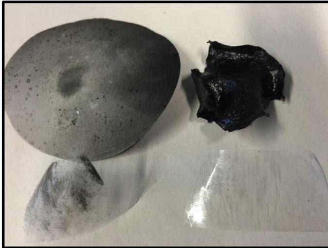
**Figure S3: Adhesion by Tape Test (a) Polypyrrole grafted on laboratory filter paper, (b) Film 4**
