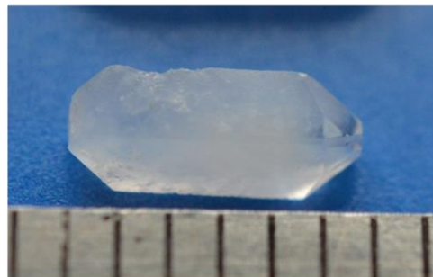
Test 6 average size, ca. 6.0 \times 2.0 \times 2.0 \text{ mm}^3
