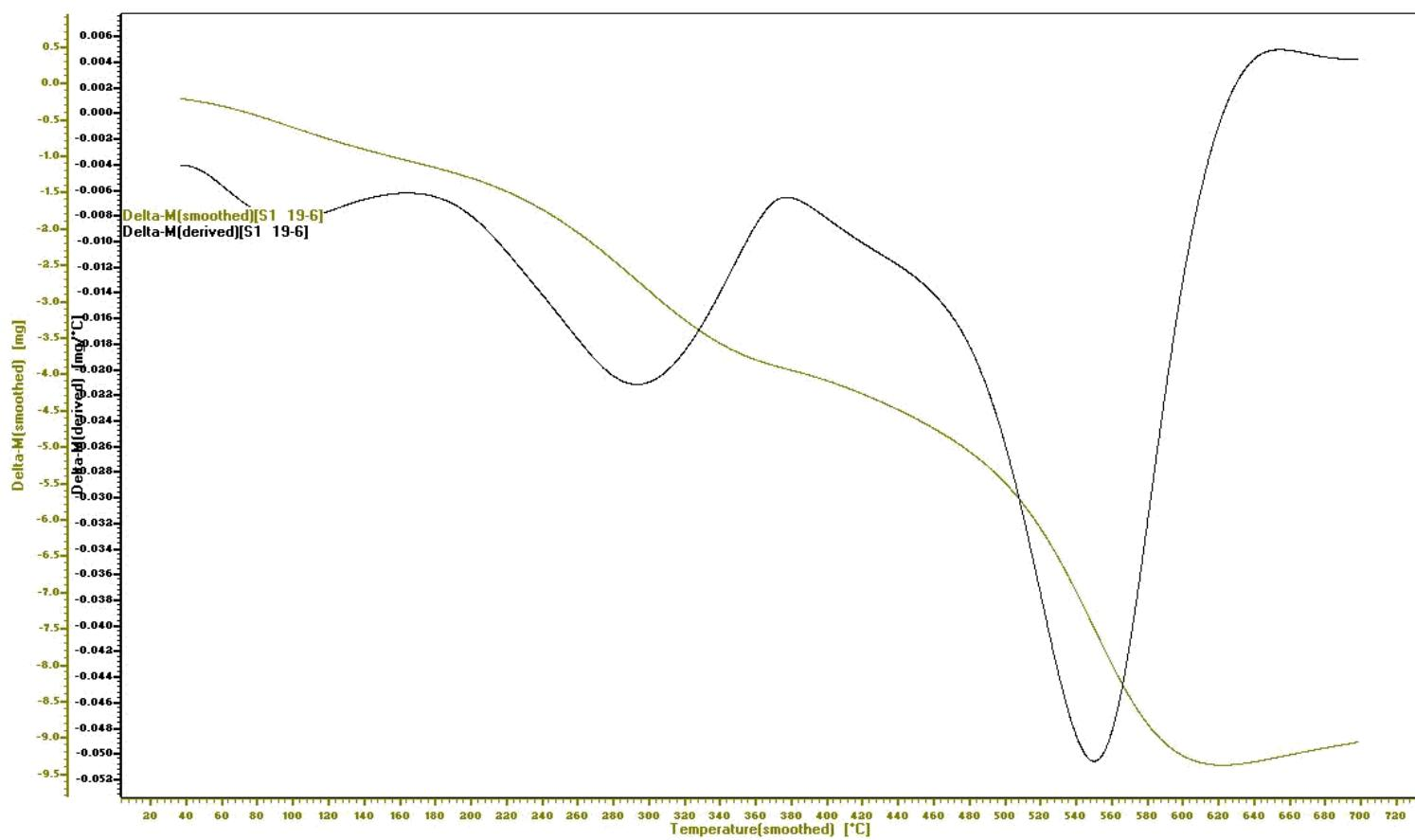
**Figure 120:** TGA/DTG of poly[2-(2-(4-aminophenylamino)-2-oxoethylamino)-6-(piperidin-1-yl)-1,3,5-triazin-2-ylamino]acetic acid **45**.
