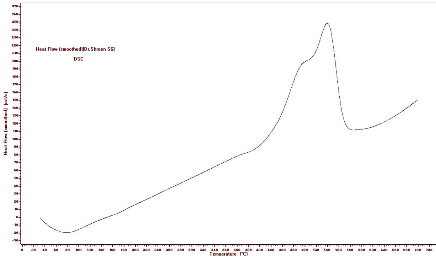
**Figure 72:** DSC of poly[2-(4-(2-(4'-aminobiphenyl-4-ylamino)-2-oxoethylamino)-6-(phenylamino)-1,3,5-triazin-2-ylamino)acetic acid] **35.**
