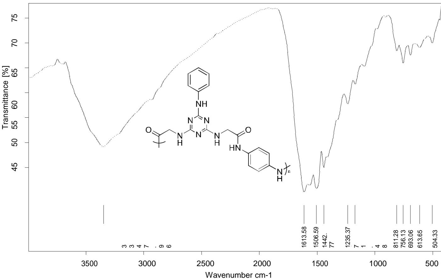
**Figure 128:** IR (KBr) of poly[2-(4-(2-(4-aminophenylamino)-2-oxoethylamino)-6-(phenylamino)-1,3,5-triazin-2-ylamino)acetic acid]
