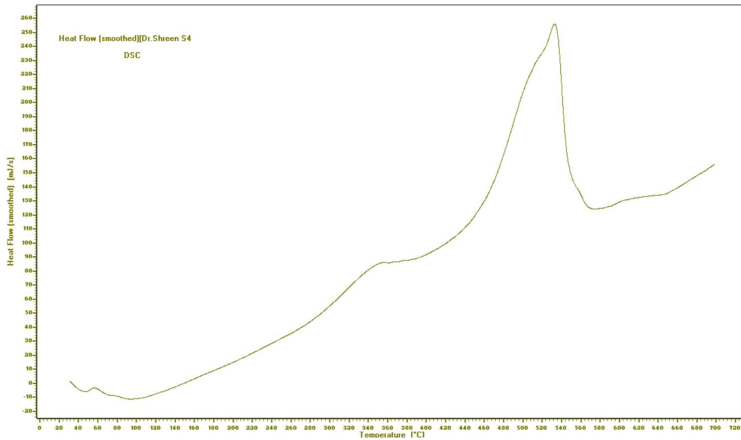
**Figure 62:** DSC of poly[2-(4-(2-(4'-aminobiphenyl-4-ylamino)-2-oxoethylamino)-6-(piperidin-1-yl)-1,3,5-triazin-2-ylamino)acetic acid] **33**.
