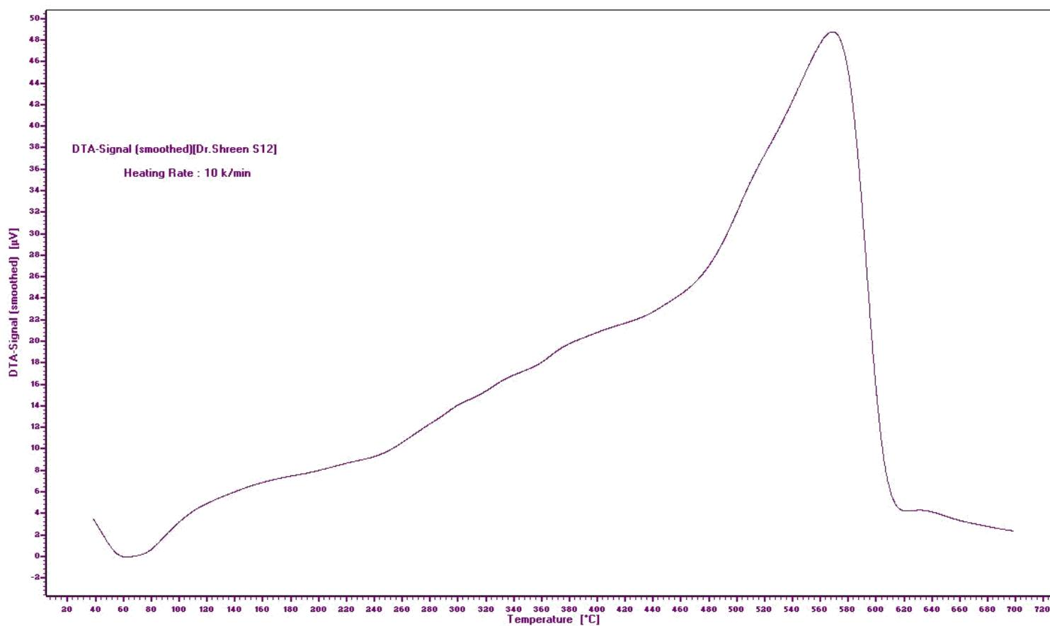
**Figure 56:** DTA of poly[2-(4-(2-(4'-aminobiphenyl-4-ylamino)-2-oxoethylthio)-6-morpholino-1,3,5-triazin-2-ylthio)acetic acid] **32**.
