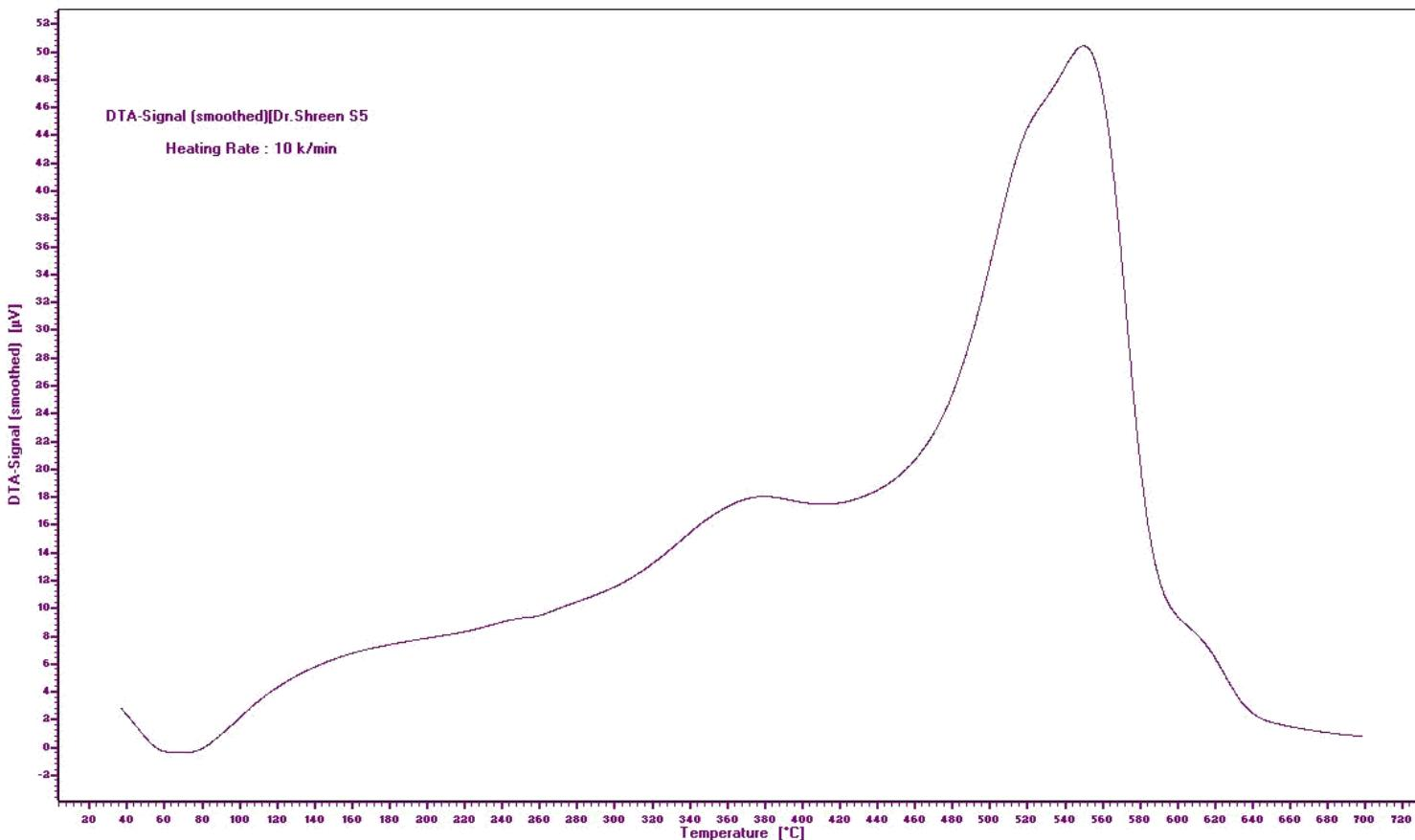
**Figure 51:** DTA of poly[2-(4-(2-(4'-aminobiphenyl-4-ylamino)-2-oxoethylamino)-6-morpholino-1,3,5-triazin-2-ylamino)acetic acid] **31.**
