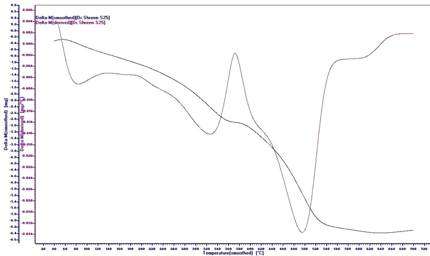
**Figure 135:** TGA/DTG of poly[2-(4-(2-(4-aminophenylamino)-2-oxoethylthio)-6-(phenylamino)-1,3,5-triazin-2-ylthio)acetic acid] **48**.
