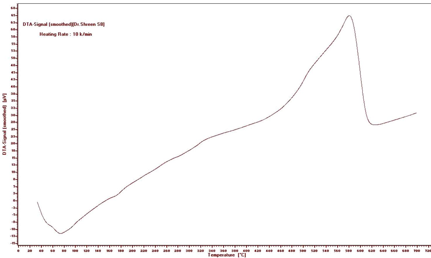
**Figure 131:** DTA of poly[2-(4-(2-(4-aminophenylamino)-2-oxoethylamino)-6-(phenylamino)-1,3,5-triazin-2-ylamino)acetic acid] **47**.
