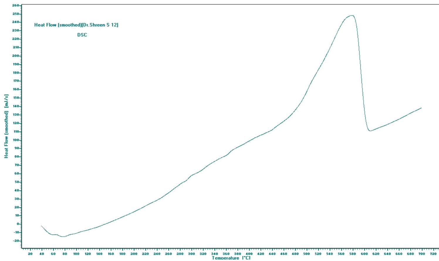
**Figure 57:** DSC of poly[2-(4-(2-(4'-aminobiphenyl-4-ylamino)-2-oxoethylthio)-6-morpholino-1,3,5-triazin-2-ylthio)acetic acid] **32**.
