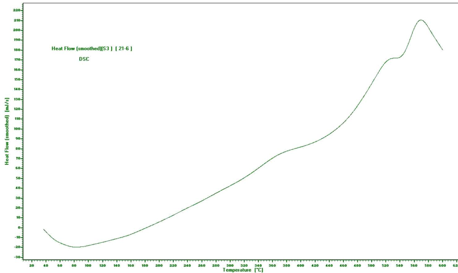
**Figure 112:** DSC of poly[2-(4-(2-(4-aminophenylamino)-2-oxoethylamino)-6-morpholino-1,3,5-triazin-2-ylamino)acetic acid] **43**.
