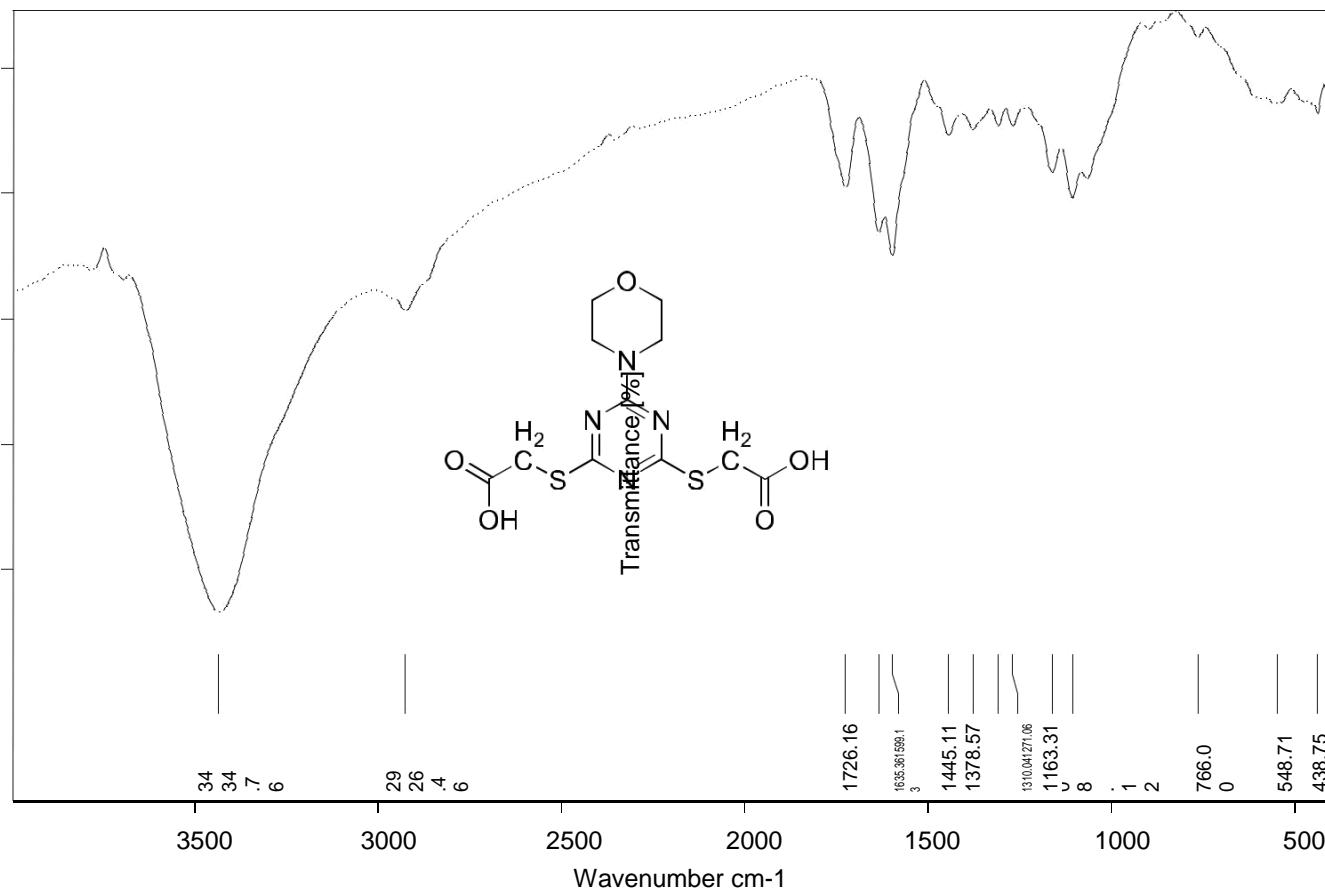
**Figure 4:** IR (KBr) of 2,2'-(6-morpholino-1,3,5-triazine-2,4-diyl)bis(sulfanediyl)diacetic acid **10**.
