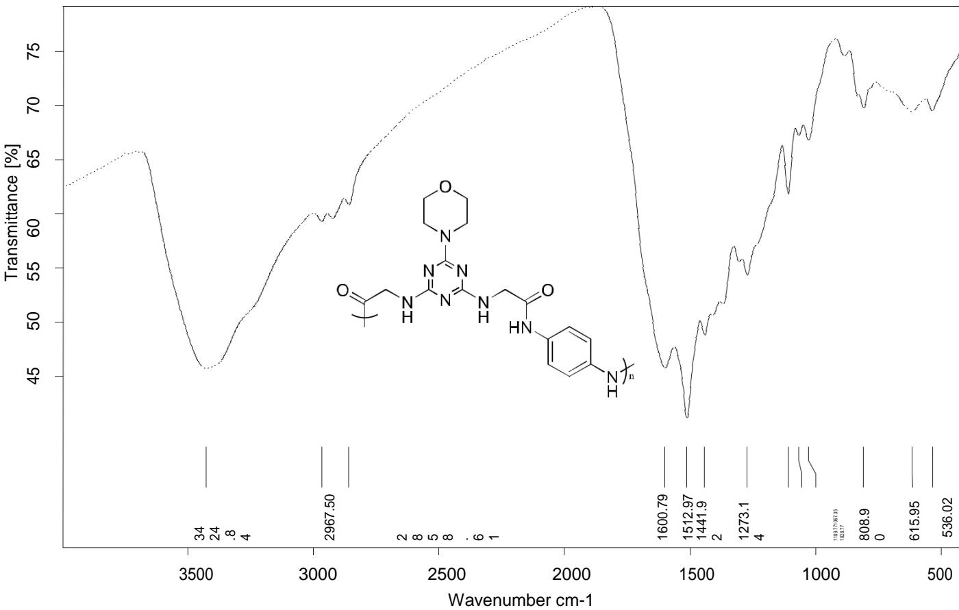
**Figure 108:** IR (KBr) of poly[2-(4-(2-(4-aminophenylamino)-2-oxoethylamino)-6-morpholino-1,3,5-triazin-2-ylamino)acetic acid] **43.**
