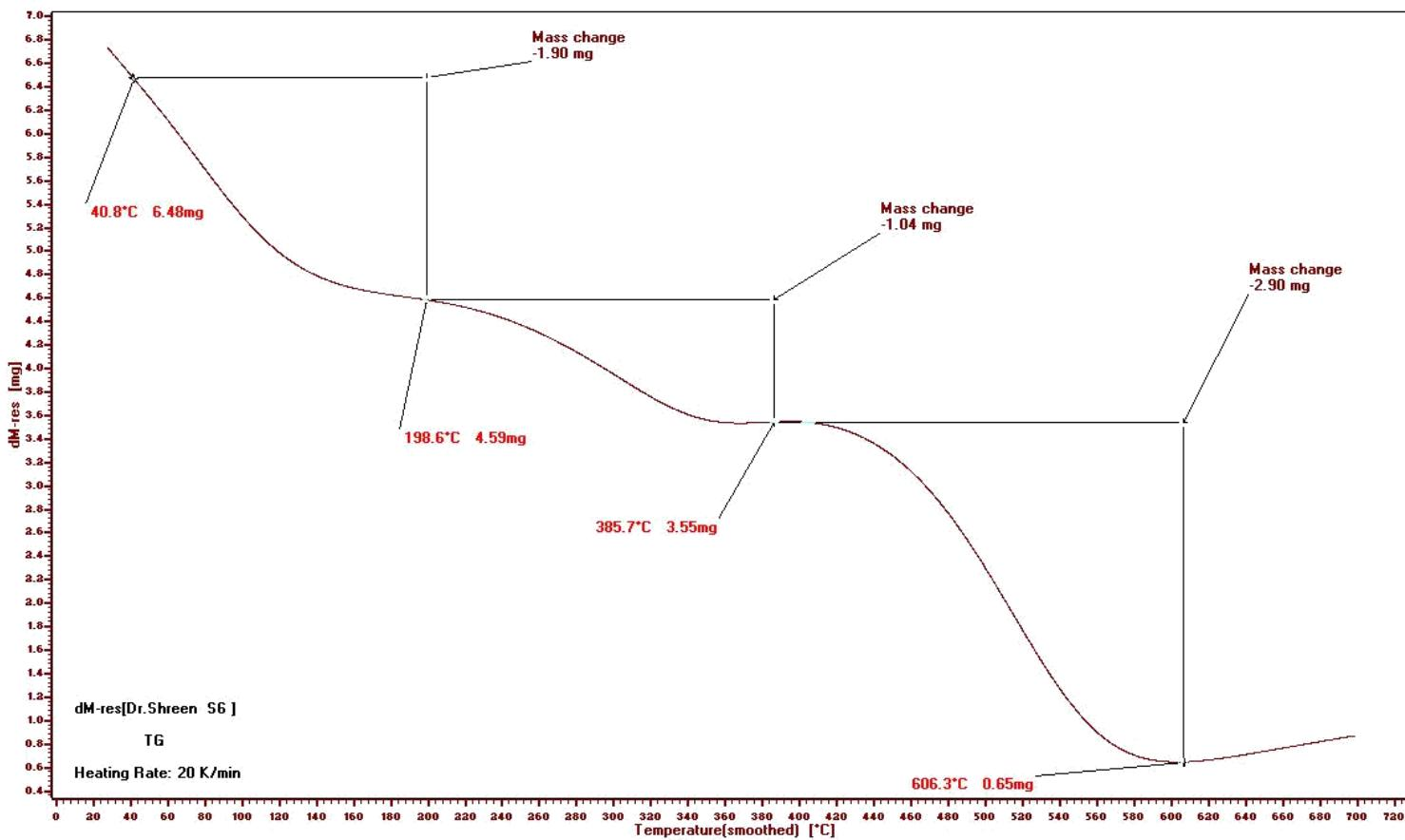
**Figure 69:** TGA of poly[2-(4-(2-(4'-aminobiphenyl-4-ylamino)-2-oxoethylamino)-6-(phenylamino)-1,3,5-triazin-2-ylamino)acetic acid]
