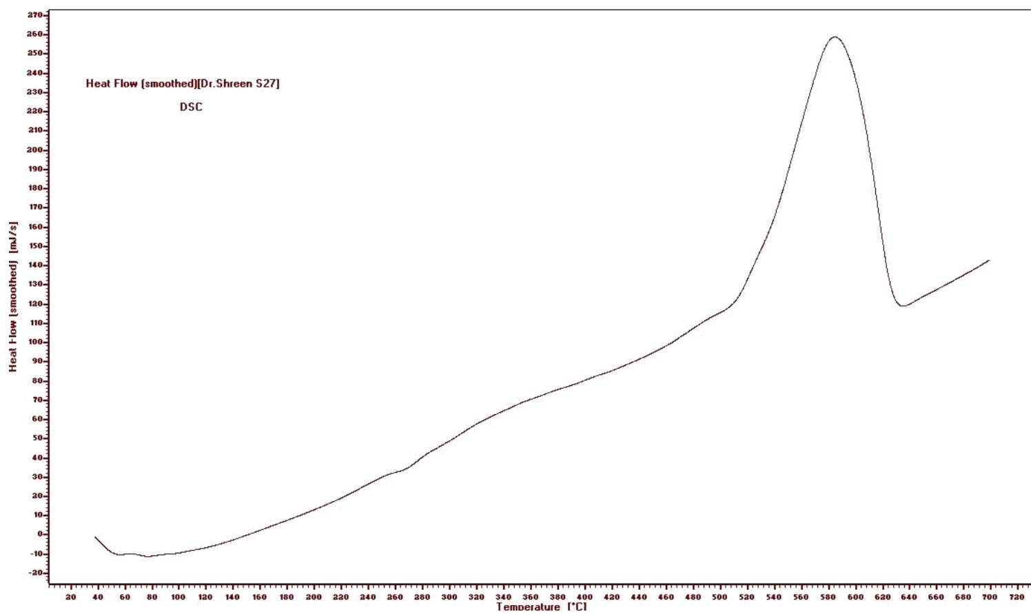
**Figure 67:** DSC of poly[2-(4-(2-(4'-aminobiphenyl-4-ylamino)-2-oxoethylthio)-6-(piperidin-1-yl)-1,3,5-triazin-2-ylthio)acetic acid] 34.
