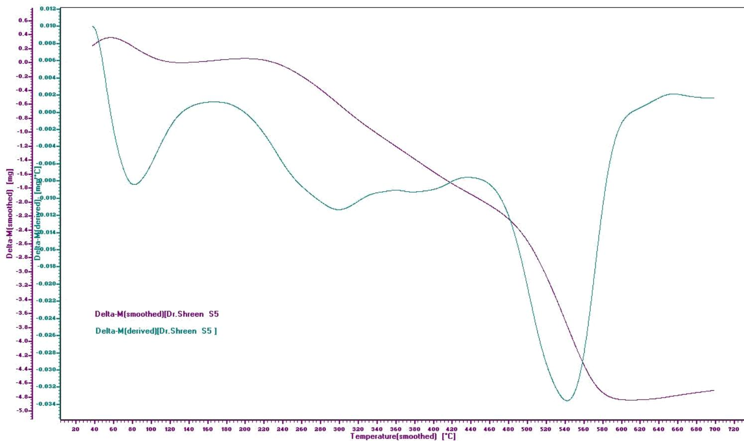
**Figure 50:** TGA/DTG of poly[2-(4-(2-(4'-aminobiphenyl-4-ylamino)-2-oxoethylamino)-6-morpholino-1,3,5-triazin-2-ylamino)acetic acid] **31**.
