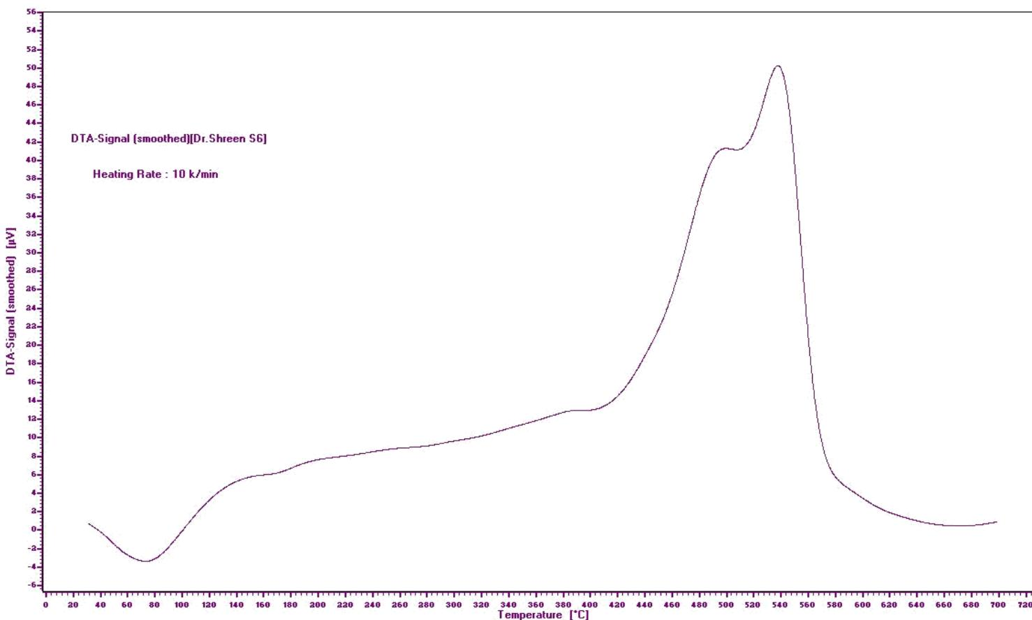
**Figure 71:** DTA of poly[2-(4-(2-(4'-aminobiphenyl-4-ylamino)-2-oxoethylamino)-6-(phenylamino)-1,3,5-triazin-2-ylamino)acetic acid]
