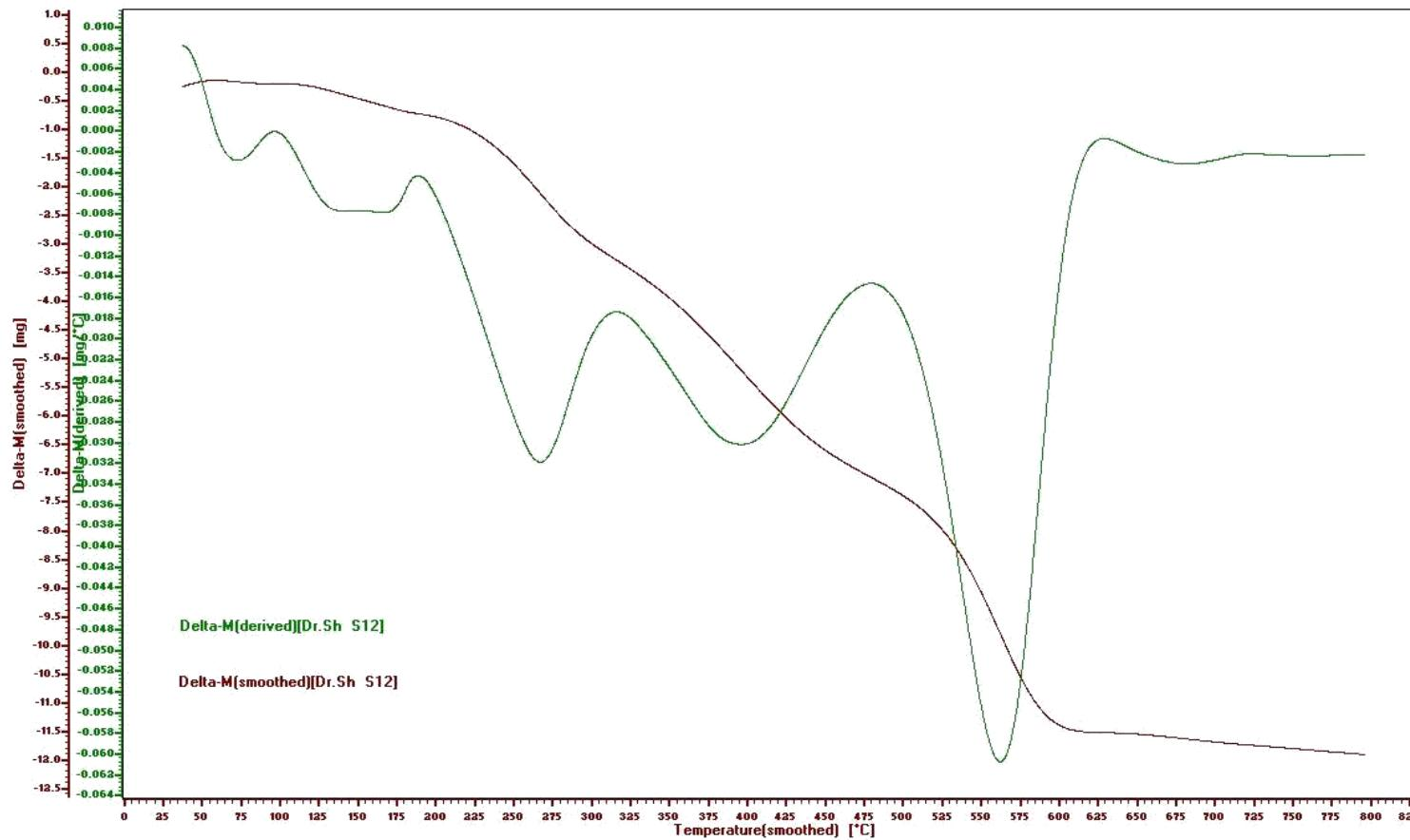
**Figure 55:** TGA/DTG of poly[2-(4-(2-(4'-aminobiphenyl-4-ylamino)-2-oxoethylthio)-6-morpholino-1,3,5-triazin-2-ylthio)acetic acid]
