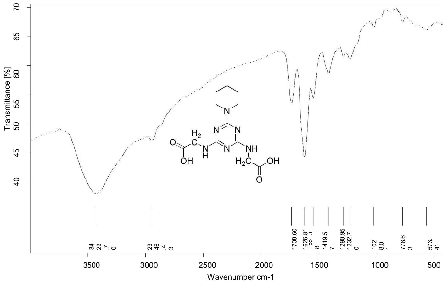
**Figure 6:** IR (KBr) of 2,2'-(6-(piperidin-1-yl)-1,3,5-triazine-2,4-diyl)bis(azanediyl)diacetic acid **11**.
