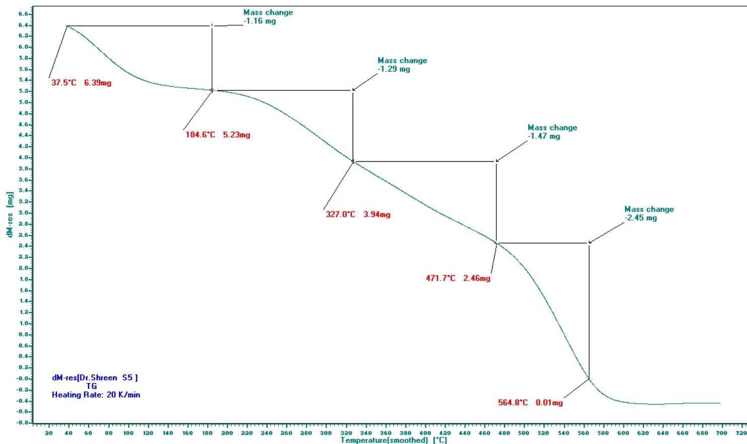
**Figure 49:** TGA of poly[2-(4-(2-(4'-aminobiphenyl-4-ylamino)-2-oxoethylamino)-6-morpholino-1,3,5-triazin-2-ylamino)acetic acid]
