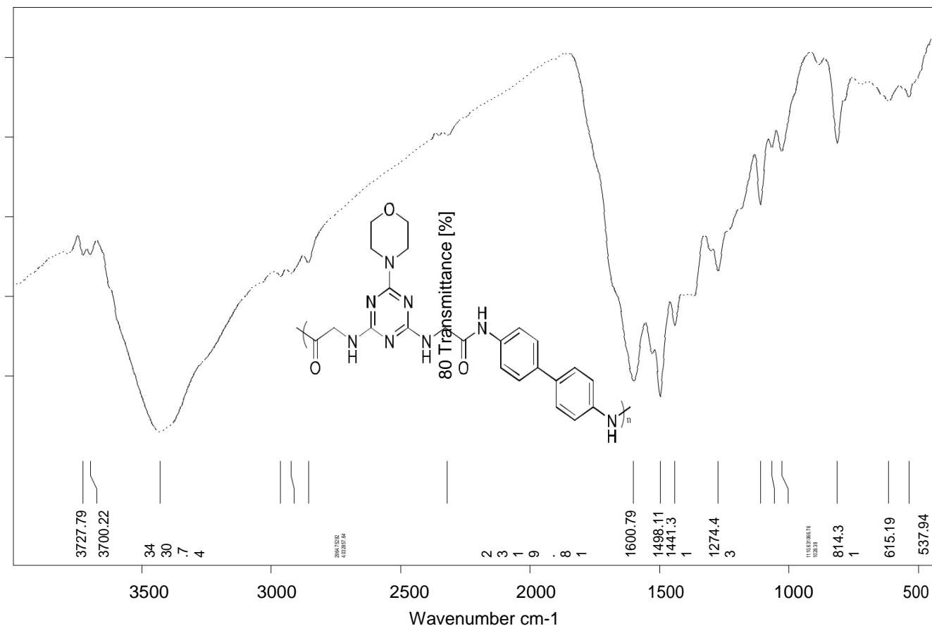
**Figure 48:** IR (KBr) of poly[2-(4-(2-(4'-aminobiphenyl-4-ylamino)-2-oxoethylamino)-6-morpholino-1,3,5-triazin-2-ylamino)acetic acid] **31.**
