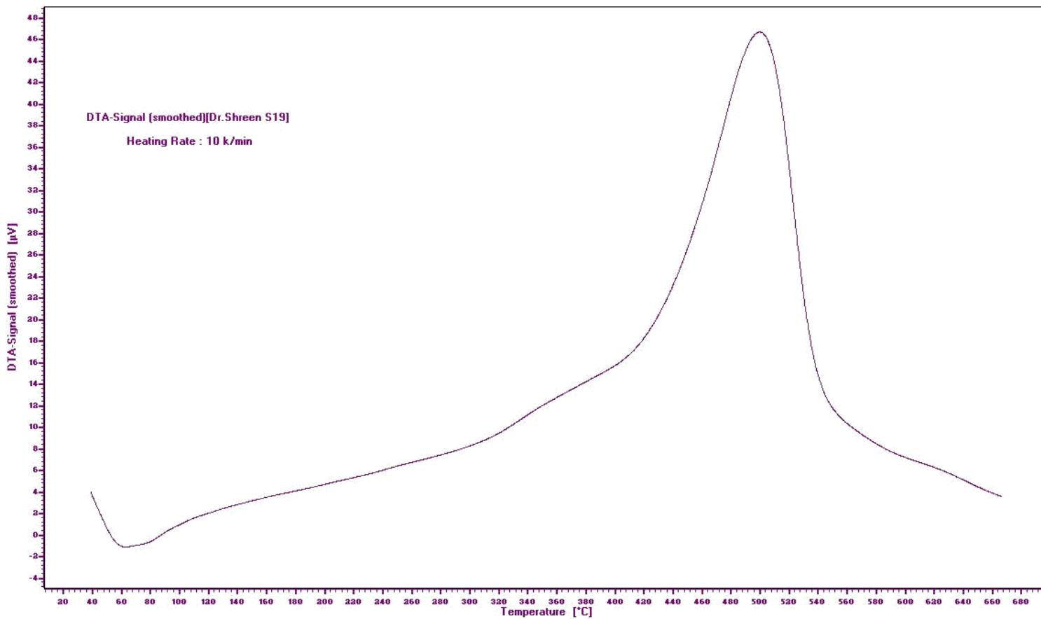
**Figure 76:** DTA of poly[2-(4-(2-(4'-aminobiphenyl-4-ylamino)-2-oxoethylthio)-6-(phenylamino)-1,3,5-triazin-2-ylthio)acetic acid] **36**.
