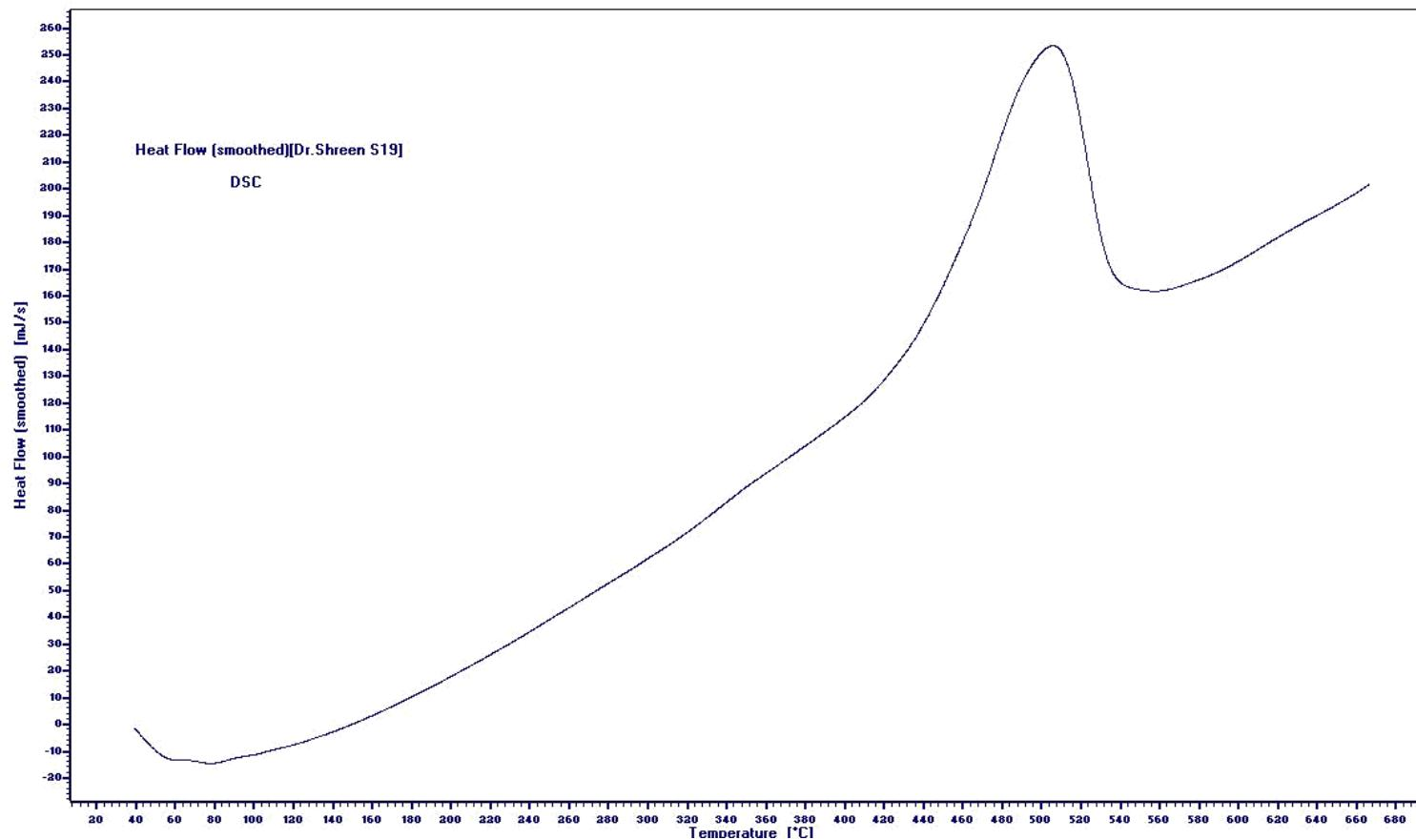
**Figure 77:** DSC of poly[2-(4-(2-(4'-aminobiphenyl-4-ylamino)-2-oxoethylthio)-6-(phenylamino)-1,3,5-triazin-2-ylthio)acetic acid] **36**.
