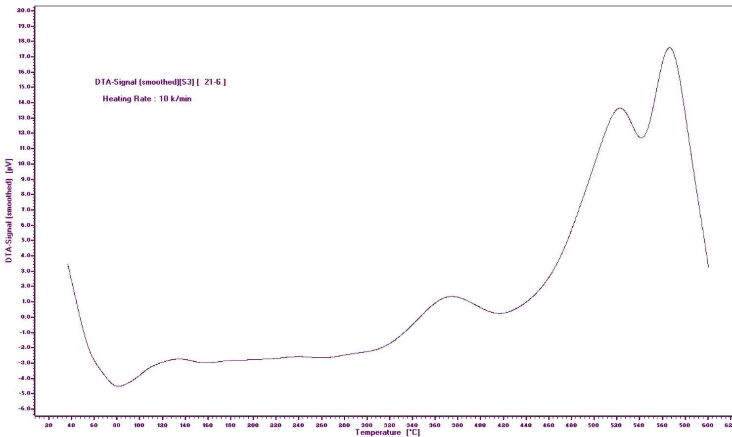
**Figure 111:** DTA of poly[2-(4-(2-(4-aminophenylamino)-2-oxoethylamino)-6-morpholino-1,3,5-triazin-2-ylamino)acetic acid] 43.
