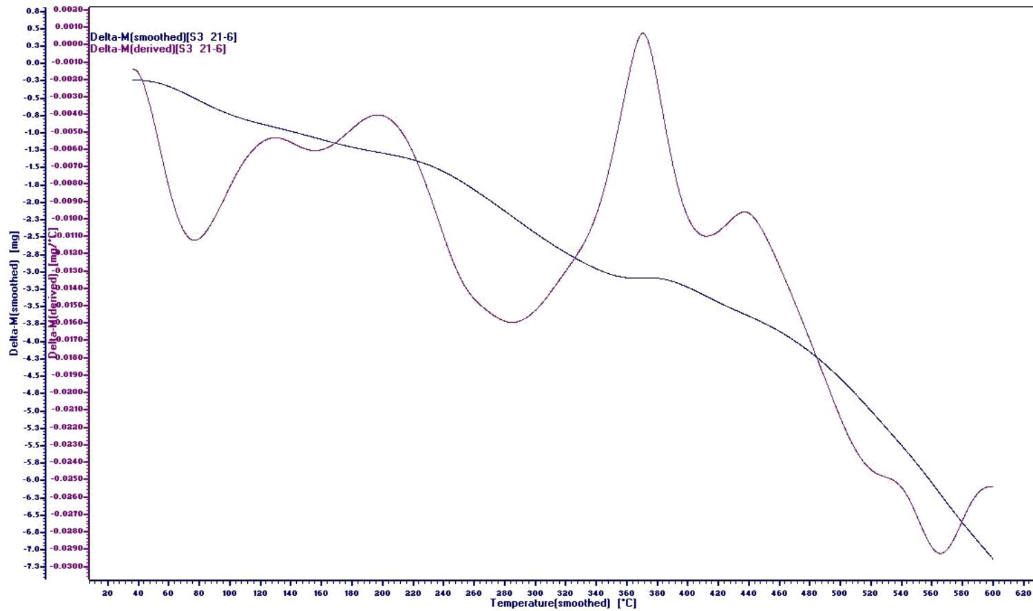
**Figure 110:** TGA/DTG of poly[2-(4-(2-(4-aminophenylamino)-2-oxoethylamino)-6-morpholino-1,3,5-triazin-2-ylamino)acetic acid]
