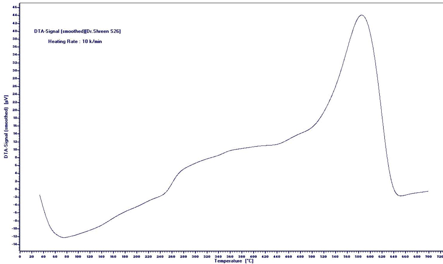
**Figure 126:** DTA of poly[2-(4-(2-(4-aminophenylamino)-2-oxoethylthio)-6-(piperidin-1-yl)-1,3,5-triazin-2-ylthio)acetic acid] **46**.
