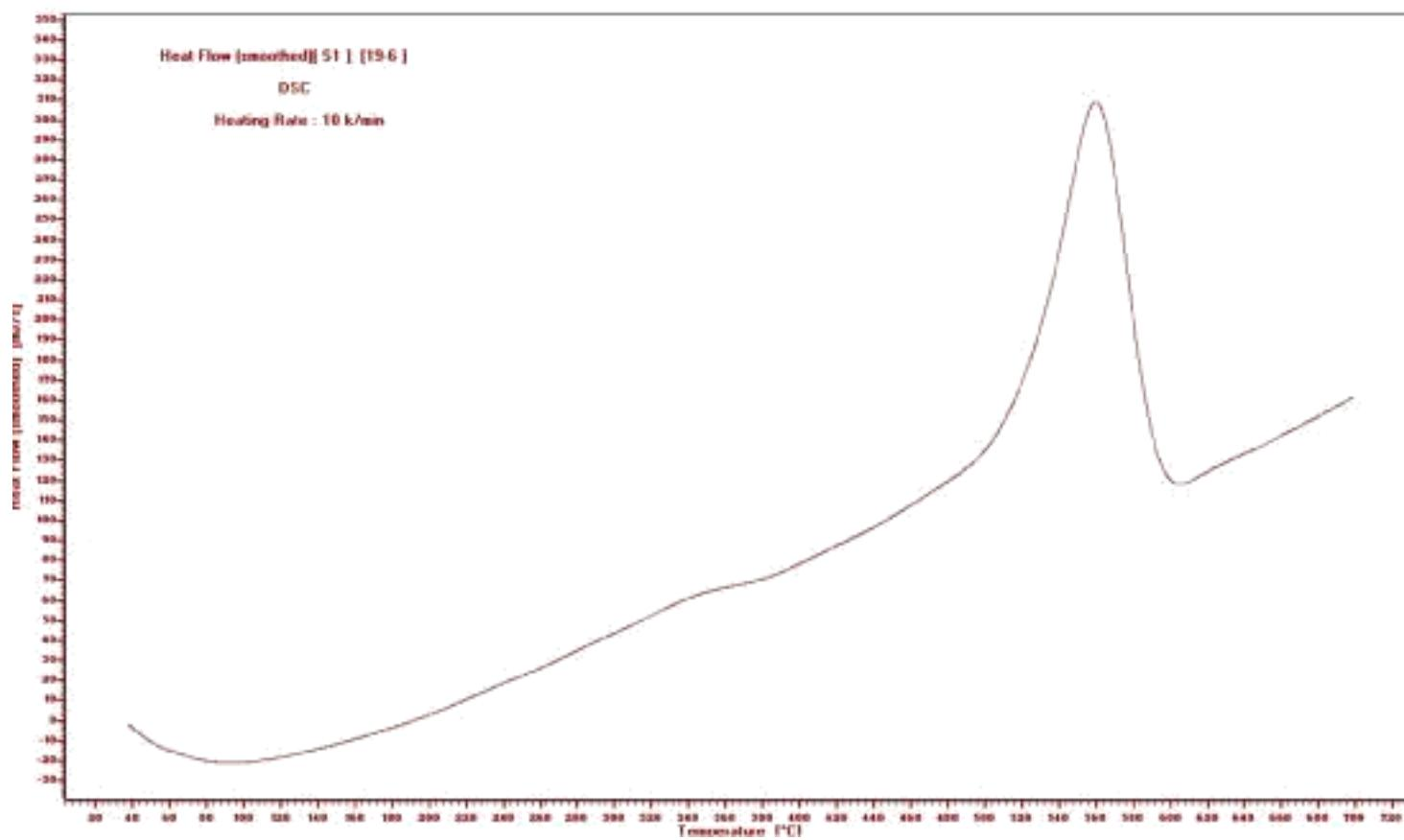
**Figure 122:** DSC of poly[2-(4-(2-(4-aminophenylamino)-2-oxoethylamino)-6-(piperidin-1-yl)-1,3,5-triazin-2-ylamino)acetic acid] **45**.
