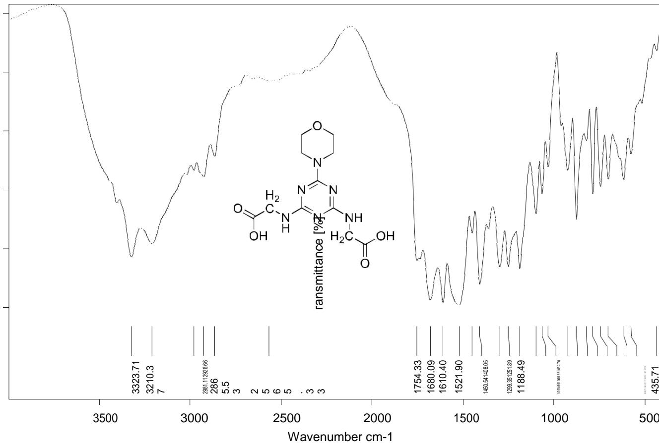
**Figure 1:** IR (KBr) of 2,2'-(6-morpholino-1,3,5-triazine-2,4-diyl)bis(azanediyl)diacetic acid
