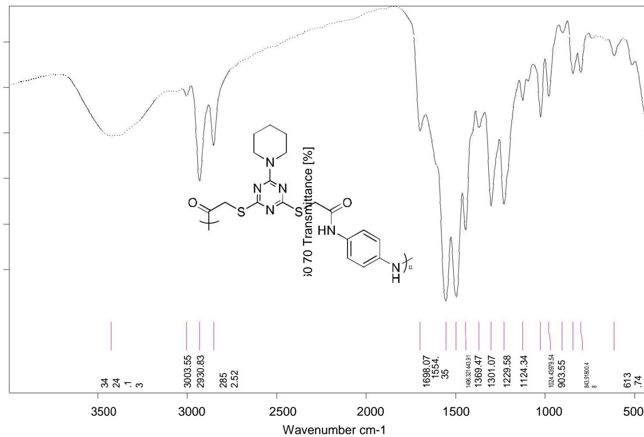
**Figure 123:** IR (KBr) of poly[2-(4-(2-(4-aminophenylamino)-2-oxoethylthio)-6-(piperidin-1-yl)-1,3,5-triazin-2-ylthio)acetic acid] 46.
