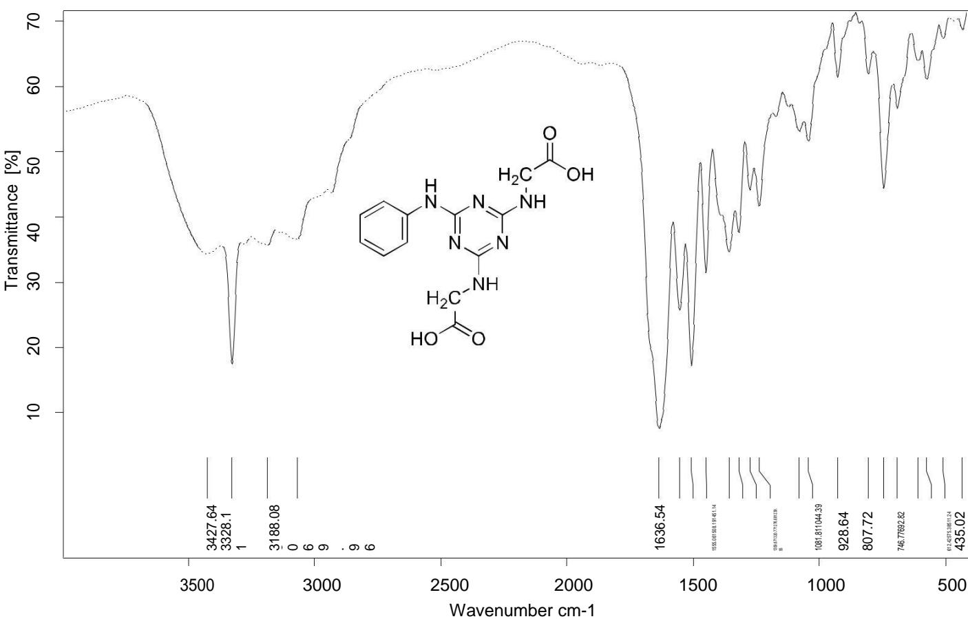
**Figure 13:** IR (KBr) of 2,2'-(6-(phenylamino)-1,3,5-triazine-2,4-diyl)bis(azanediyl)diacetic acid **13**.
