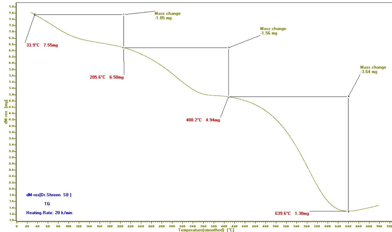
**Figure 129:** TGA of poly[2-(4-(2-(4-aminophenylamino)-2-oxoethylamino)-6-(phenylamino)-1,3,5-triazin-2-ylamino)acetic acid] **47**.
