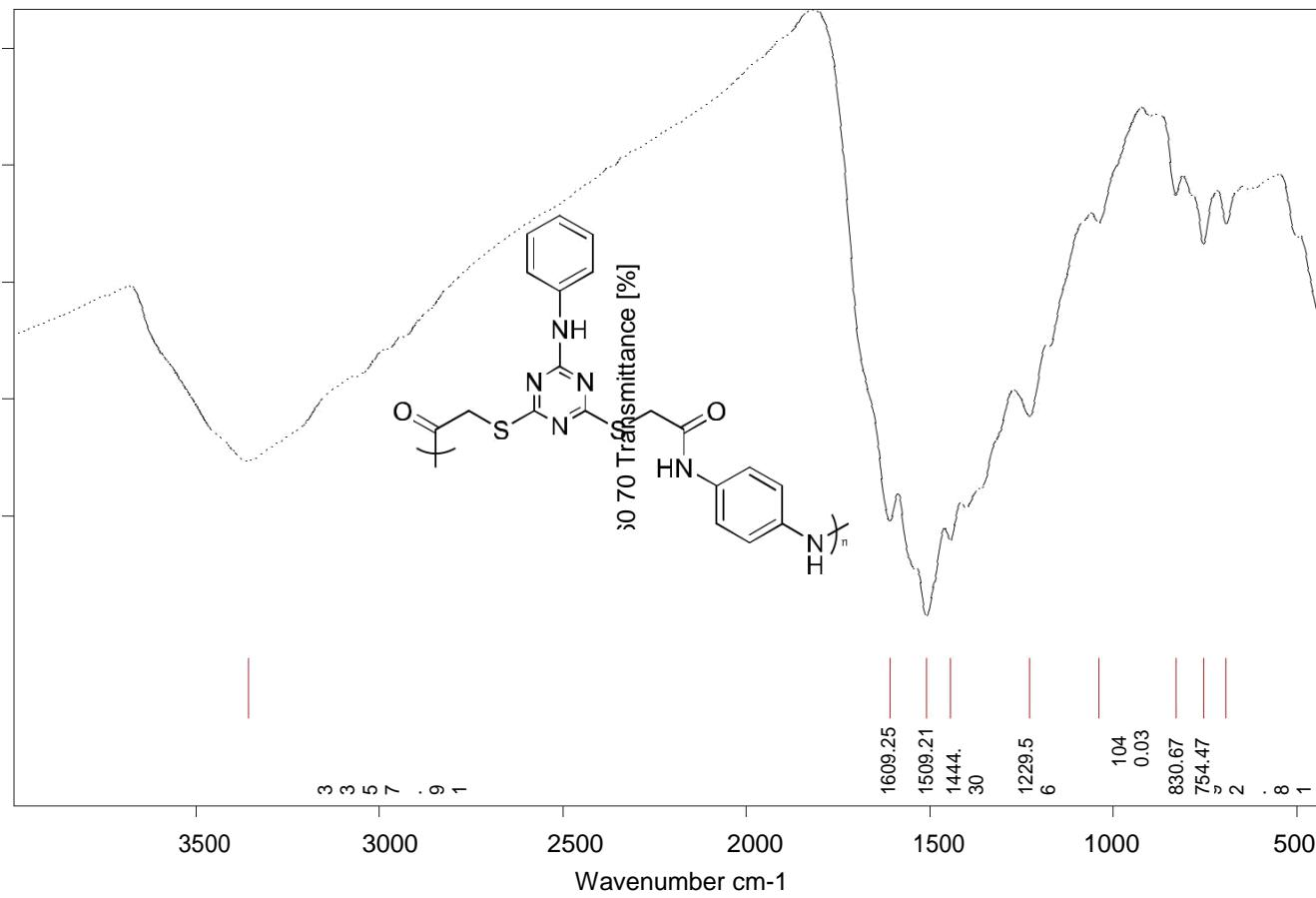
**Figure 133:** IR (KBr) of poly[2-(4-(2-(4-aminophenylamino)-2-oxoethylthio)-6-(phenylamino)-1,3,5-triazin-2-ylthio)acetic acid] **48.**
