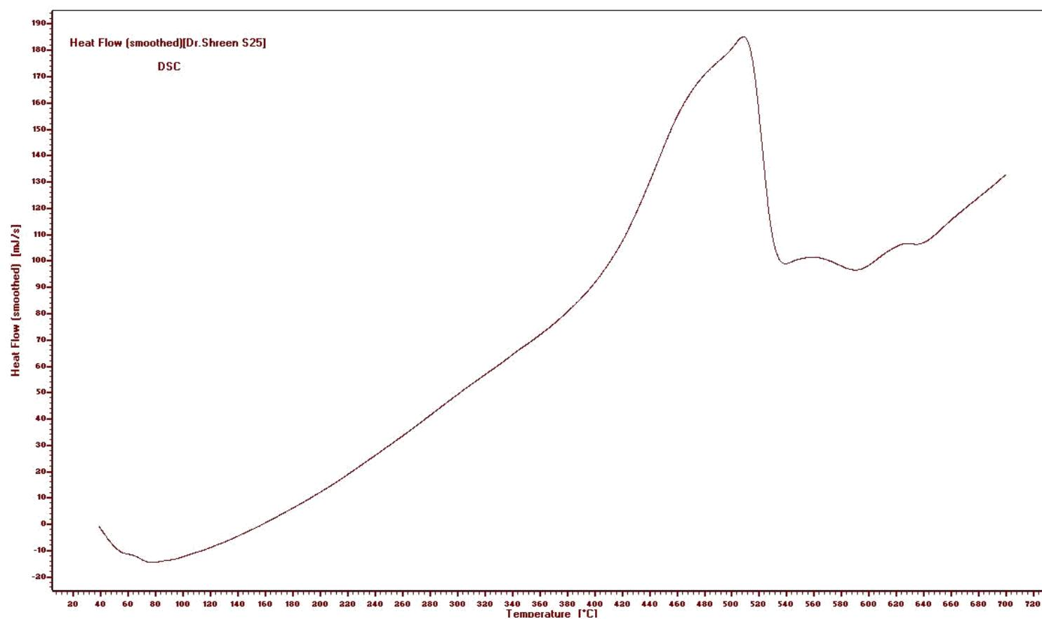
**Figure 137:** DSC of poly[2-(4-(2-(4-aminophenylamino)-2-oxoethylthio)-6-(phenylamino)-1,3,5-triazin-2-ylthio)acetic acid] **48**.
