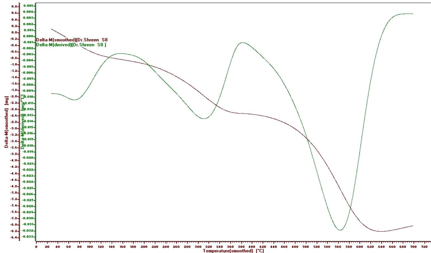
**Figure 130:** TGA/DTG of poly[2-(4-(2-(4-aminophenylamino)-2-oxoethylamino)-6-(phenylamino)-1,3,5-triazin-2-ylamino)acetic acid]
