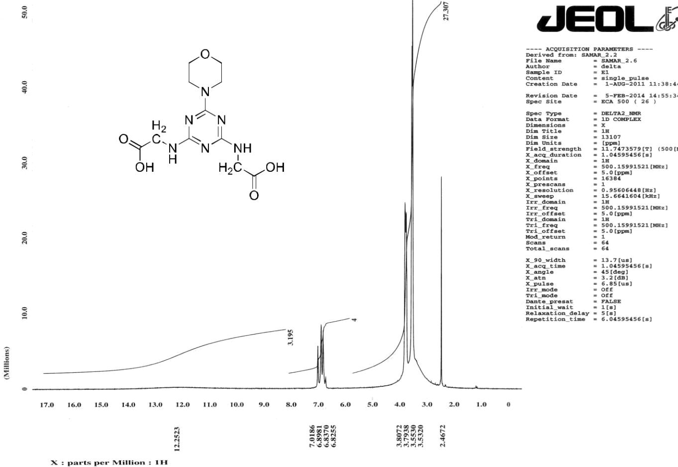
**Figure 2:**  $^1\text{H}$ -NMR (DMSO-d<sub>6</sub>) of 2,2'-(6-morpholino-1,3,5-triazine-2,4-diyl)bis(azanediyl)diacetic acid **9**.
