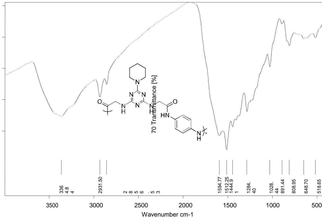
**Figure 118:** IR (KBr) of poly[2-(4-(2-(4-aminophenylamino)-2-oxoethylamino)-6-(piperidin-1-yl)-1,3,5-triazin-2-ylamino)acetic acid]
