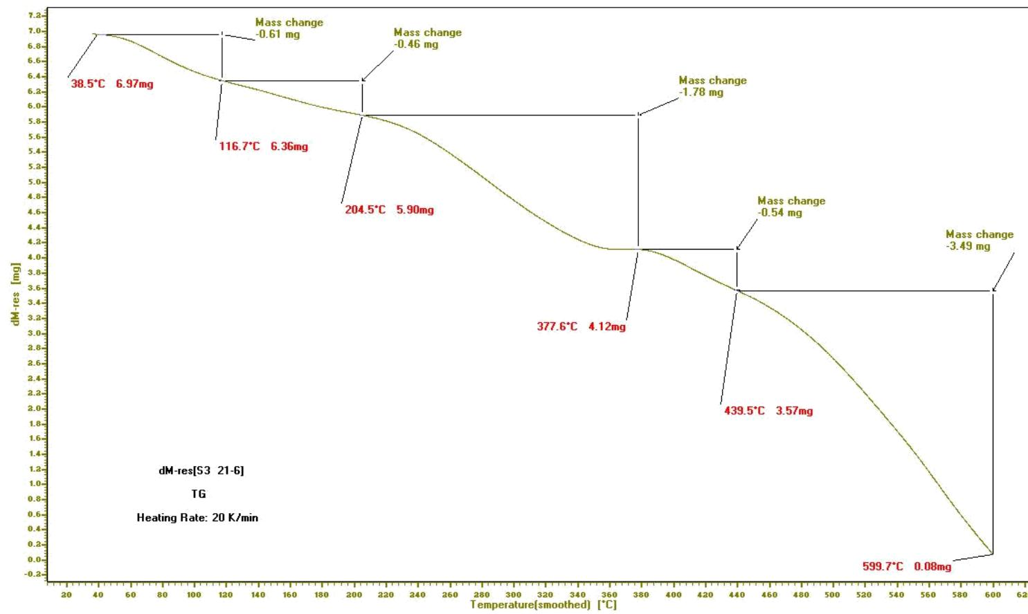
**Figure 109:** TGA of poly[2-(4-(2-(4-aminophenylamino)-2-oxoethylamino)-6-morpholino-1,3,5-triazin-2-ylamino)acetic acid] 43.
