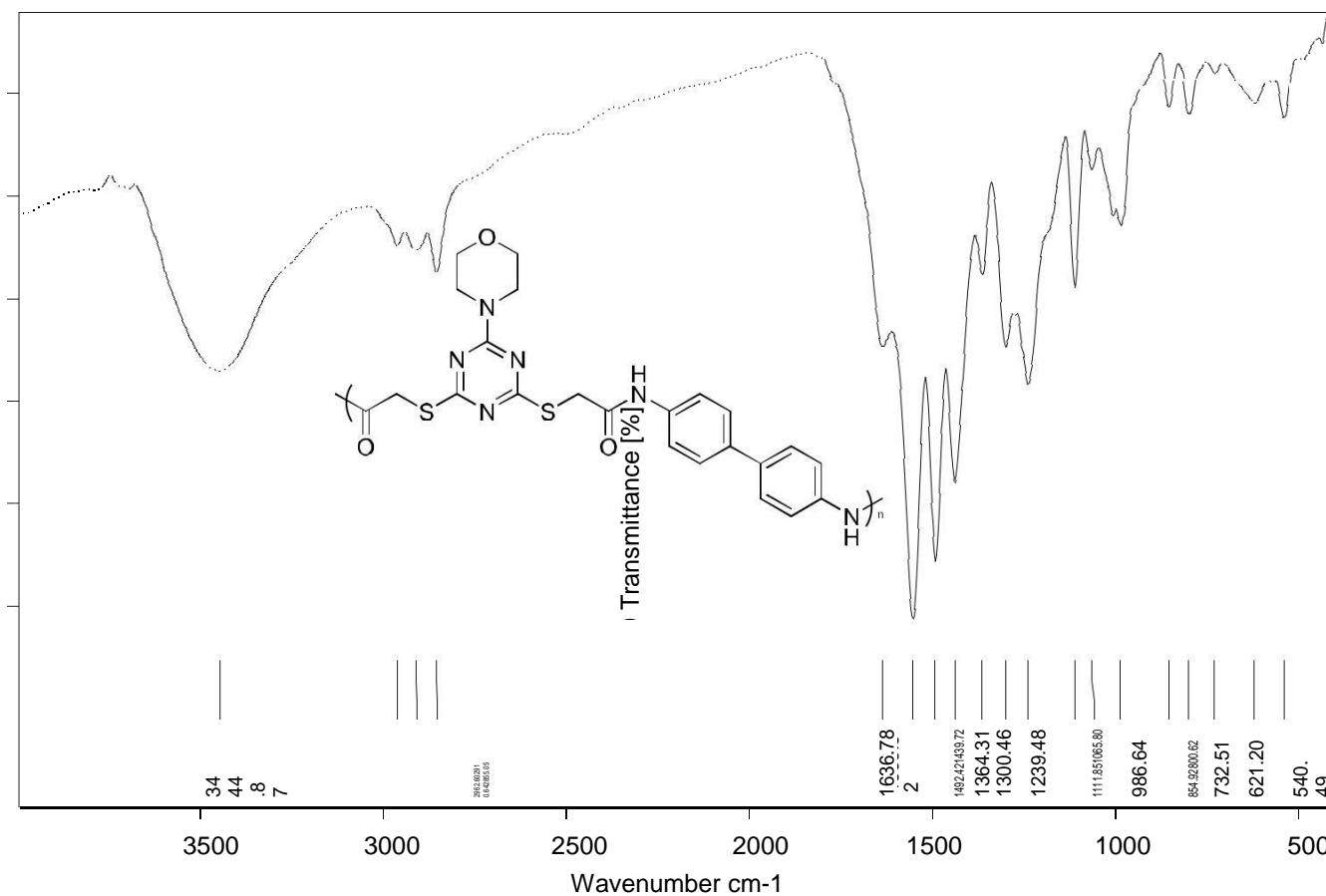
**Figure 53:** IR (KBr) of poly[2-(4-(2-(4'-aminobiphenyl-4-ylamino)-2-oxoethylthio)-6-morpholino-1,3,5-triazin-2-ylthio)acetic acid] **32.**
