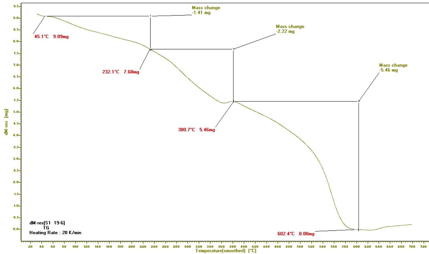
**Figure 119:** TGA of poly[2-(4-(2-(4-aminophenylamino)-2-oxoethylamino)-6-(piperidin-1-yl)-1,3,5-triazin-2-ylamino)acetic acid] **45**.
