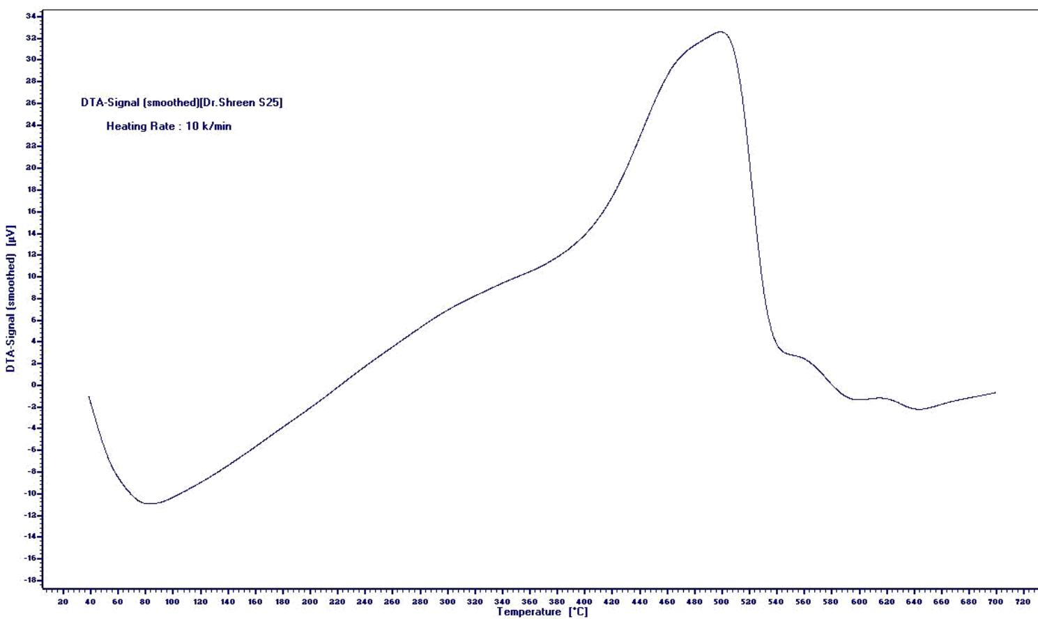
**Figure 136:** DTA of poly[2-(4-(2-(4-aminophenylamino)-2-oxoethylthio)-6-(phenylamino)-1,3,5-triazin-2-ylthio)acetic acid] 48.
