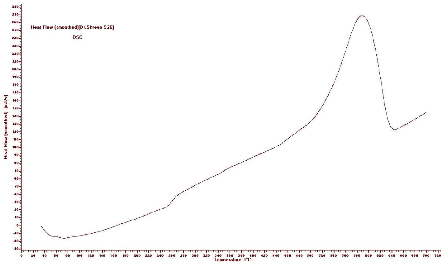
**Figure 127:** DSC of poly[2-(4-(2-(4-aminophenylamino)-2-oxoethylthio)-6-(piperidin-1-yl)-1,3,5-triazin-2-ylthio)acetic acid] **46**.
