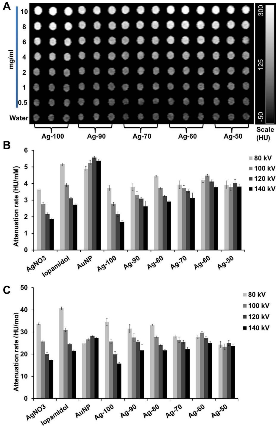
Figure S3: CT phantom images of GSAN (Ag-100, Ag-90, Ag-70, Ag-60 and Ag-50) scanned at 80 kV (A); CT attenuation rates HU/mM (B) and HU/mg (C) of different agents.
