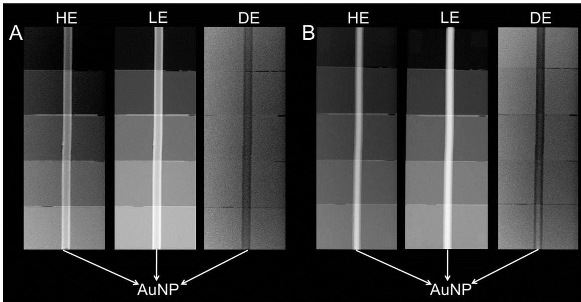
Figure S2. Dual energy mammography phantom images of AuNP at concentrations of 16 mg/ml (A) and 50 mg/ml (B). HE: high energy image; LE: low energy image and DE: dual energy subtraction image.
