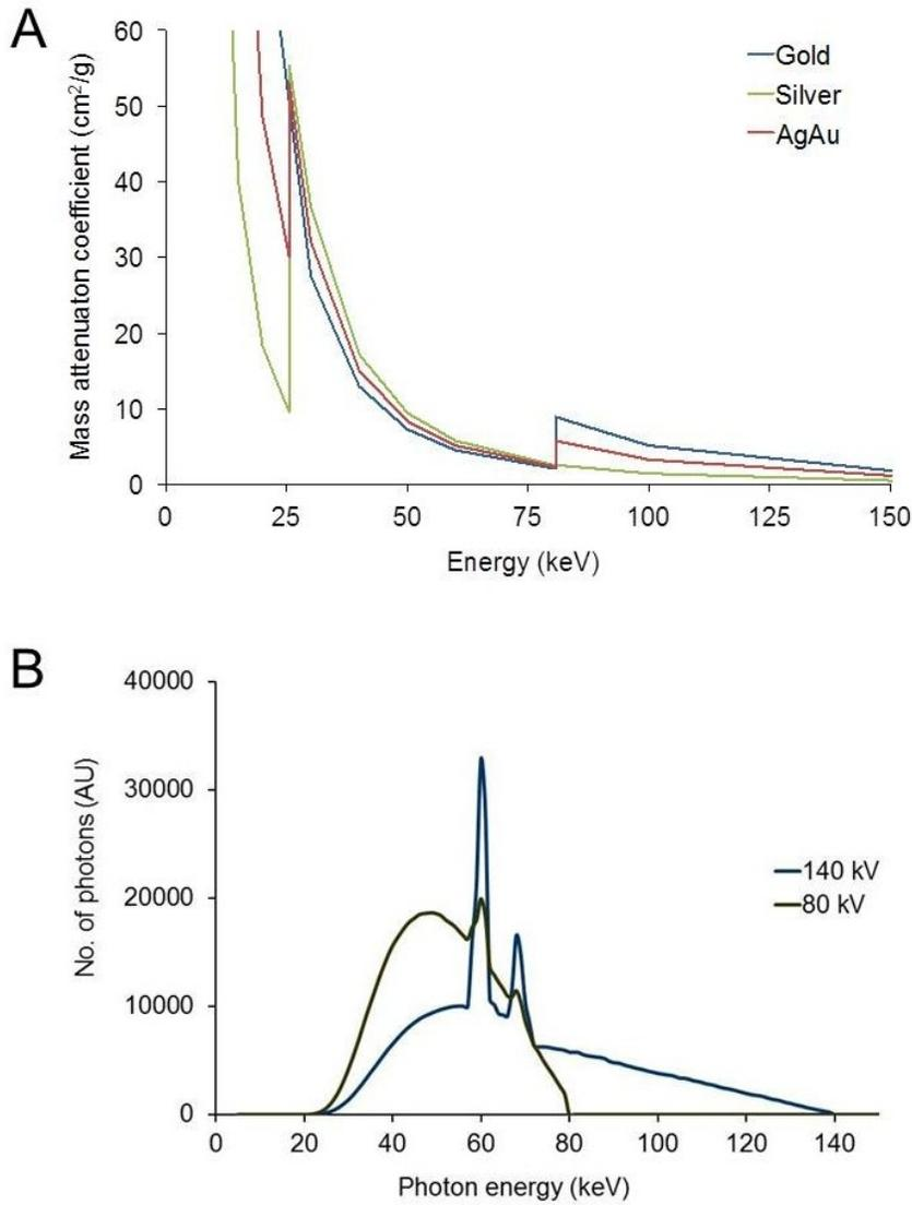
Figure S4: (A) Mass attenuation coefficients of gold, silver and 1:1 mixture of gold and silver. The data was obtained from the NIST website. (B) Photon energy distribution generated from the X-ray tube of a CT scanner run at 80 or 140 kV.
