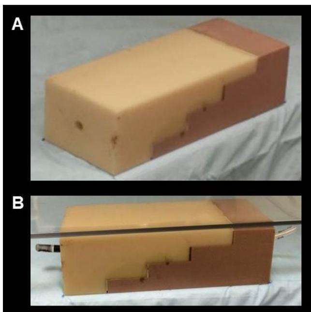
Figure S5. DE Mammography step phantom image, A) Empty phantom; B) Tube containing GSAN inserted into the step phantom.
