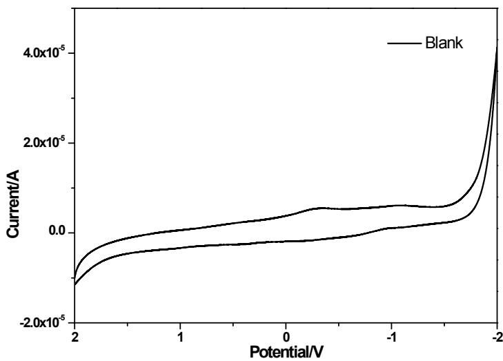
CV background was taken in chloroform solvent. Glassy carbon as working electrode, in the presence of 0.1 M tetrabutylammonium hexafluorophosphate as supporting electrolyte.
