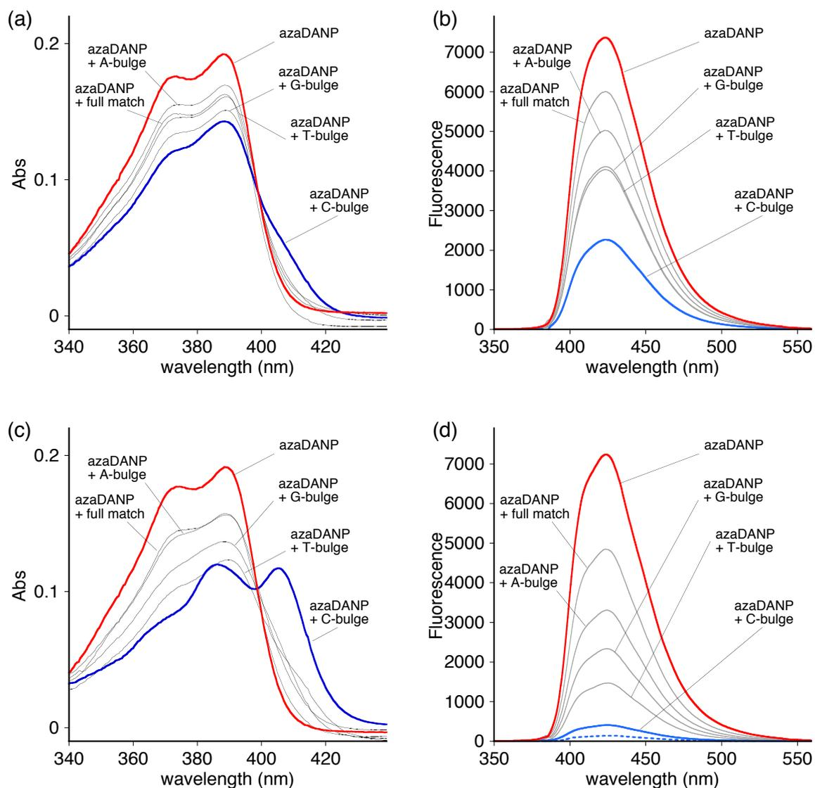
**Figure S2.** Absorption (a and c) and fluorescent (b and d) spectra of azaDANP (10  $\mu\text{M}$ ) (red line) with bulged DNA (30  $\mu\text{M}$ ) 5'-d(GTTGCNCTGGA)-3'/3'-d(CAACGGACCT)-5', where N is A, T, G, C (blue line), or full match at pH 7.0 (a and b) or 5.5 (c and d) (10 mM sodium cacodylate, 100 mM NaCl). Excitation wavelength was at the absorption maxima. Blue dotted line in (d) showed fluorescent spectra excited at 405 nm.
