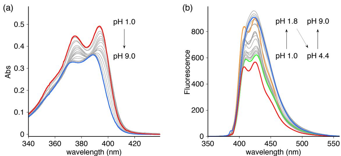
**Figure S1.** (a) Absorption and (b) fluorescent spectra of azaDANP (20  $\mu$ M) at various pHs in the solutions of buffer (20 mM) and NaCl (100 mM). Excitation wavelength was at the absorption maxima. Fluorescent spectra at 1.0 (red line), 1.8 (orange line), 4.4 (green line), and 9.0 (blue line) were shown colored.
