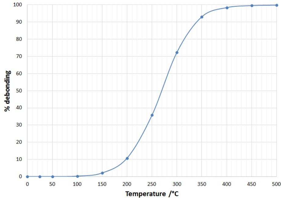
$$T_{20\% \text{ debonding}} = 225 \text{ }^{\circ}\text{C}$$
