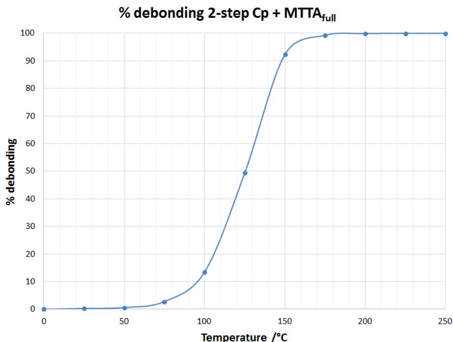
$T_{20\% \text{ debonding}} = 105^\circ\text{C}$
