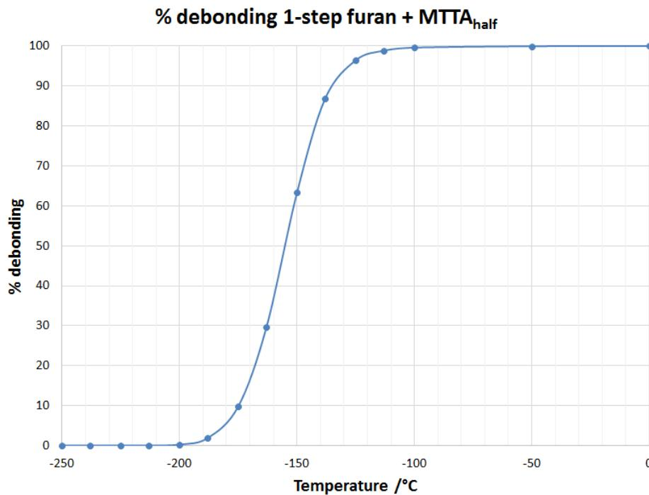
$$T_{20\% \text{ debonding}} = -169 \text{ }^{\circ}\text{C}$$
