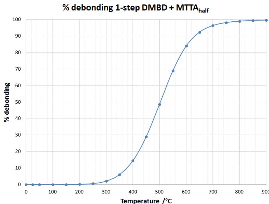
$$T_{20\% \text{ debonding}} = 427 \text{ }^{\circ}\text{C}$$
