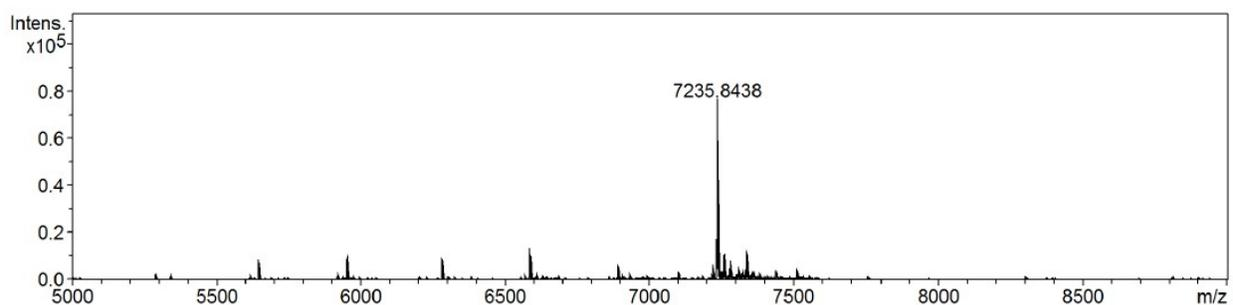
**Figure SF6:** LC/MS data for RNA with 3'end N[PFC] modification. The data was processed and deconvoluted using the Bruker DataAnalysis software version 4.1. Calculated exact mass: 7235.94, Obtained: 7235.84.
