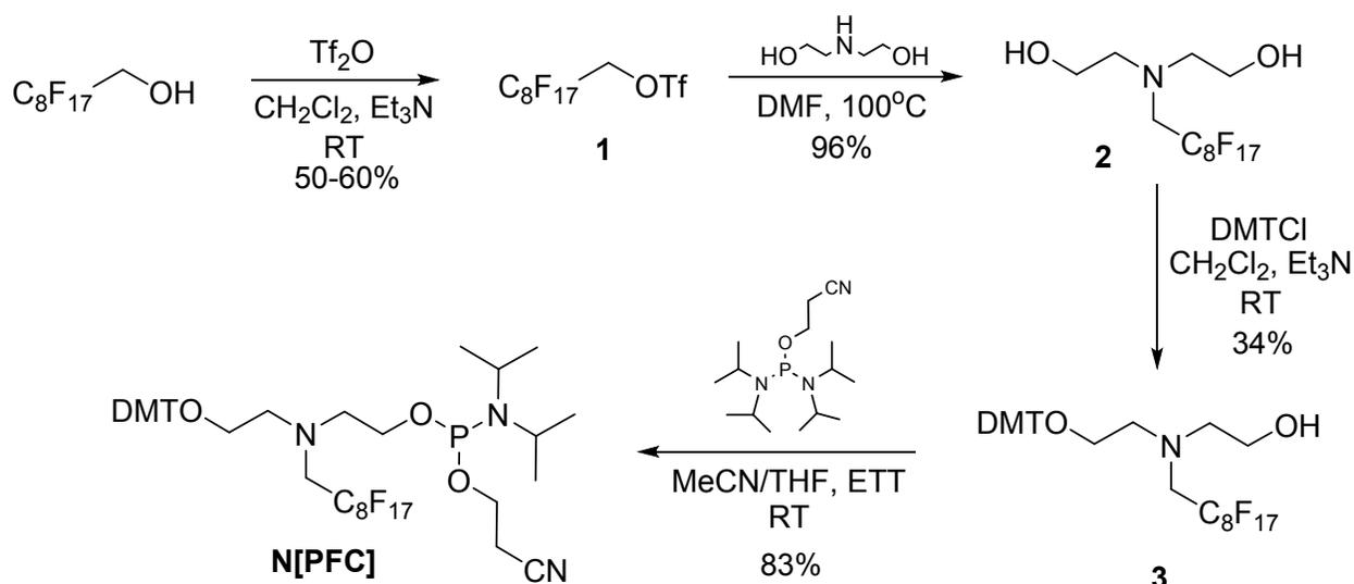
**Supporting Scheme SS1:** Synthetic pathway for the preparation of N[PFC] phosphoramidite.
