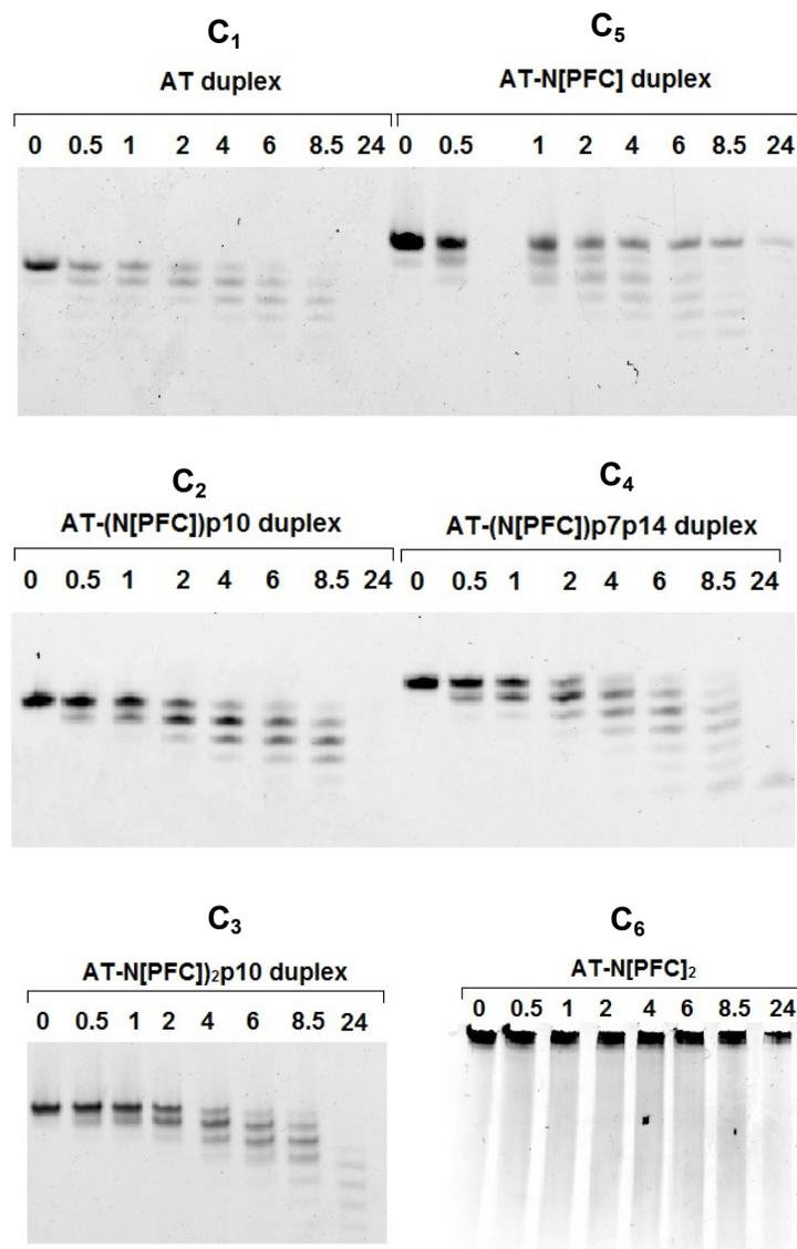
**Figure SF16A.** Representative gels after FBS degradation assays. The name of the analyzed strand is on top of each gel and numbers correspond to the time the aliquot were taken (h). One would notice that  $C_6$  leads to non-penetrating bands only. This is probably due to self-assembly in DMEM+10%FBS (presence of mono/divalent cations).
