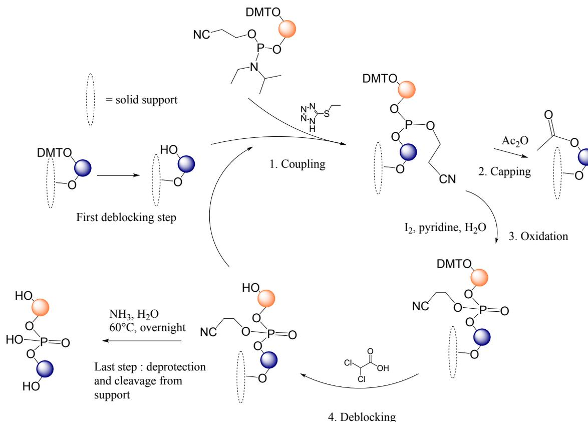
**Supporting Figure SF1:** Synthetic cycle performed by the automated synthesizer. Orange and blue spheres represent the monomers used.
