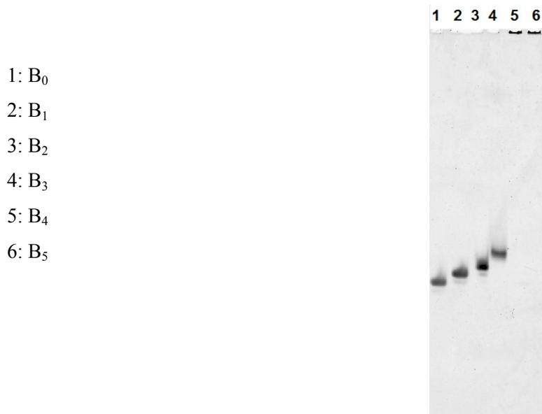
**Figure SF7:** 15% denaturing PAGE analysis of DNA-Teflon polymers. The DNA sequence is the AT one and the length of the PFC tail vary from 0 to 5 PFC units ( $B_n$  polymers). From  $n=4$ , self-assembly occurs and the material does not seem able to penetrate in the gel (non-penetrating band).
