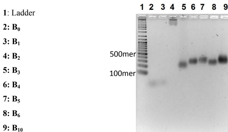
**Figure SF9:** 2.5% AGE analysis of the different AT-(N[PFC]<sub>n</sub>) strands in TAMg. Aggregation seems to occur from n=2 but clean assembled products appear from n=3. According to the ladder used, their hydrodynamic volume is greater than that of a 400mer. Mobility difference between each band of the ladder corresponds to a 100nucleotide difference.
