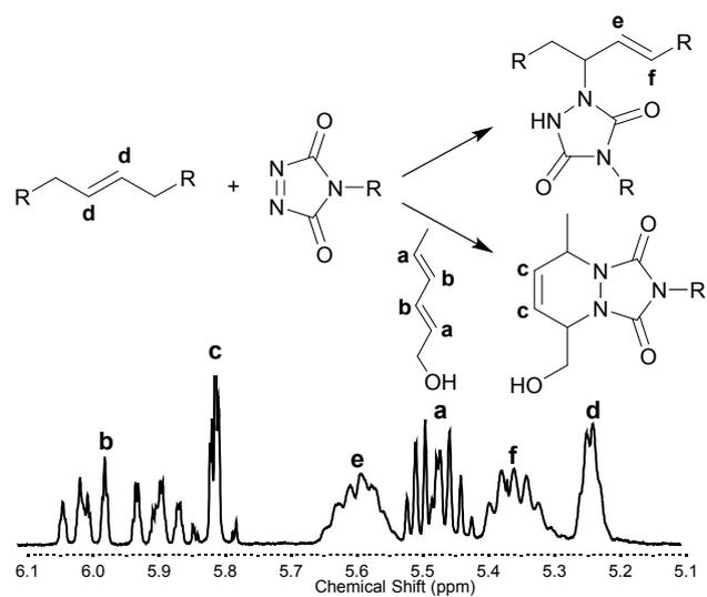
Figure S 1 – Modification kinetics: Quenching with HDEO makes analysis via  $^1\text{H-NMR}$  possible; Conversions were obtained by comparison of the signals at 5.50 ppm (e, 1 olefinic proton after modification) and 5.25 ppm (d, 2 olefinic protons before modification) as these signals show no interference with the HDEO signals (a, b, c).
