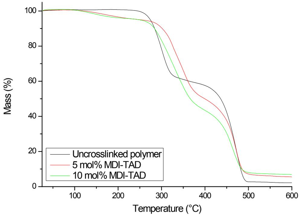
Figure S 23 - Example of crosslinking of 50 mol% PhTAD modified P1 with 5 and 10 mol% MDI-TAD - TGA data.
