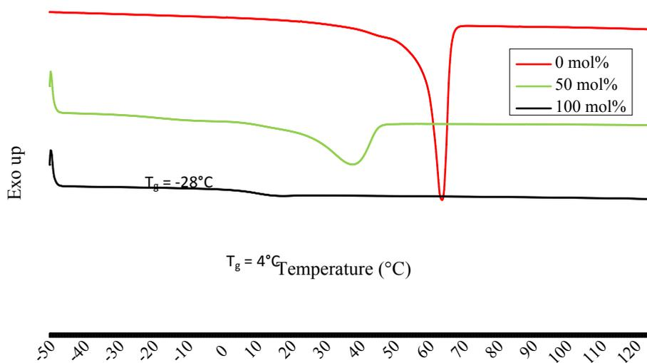
Figure S 15 - Modification of P2 with PhTAD – DSC data.
