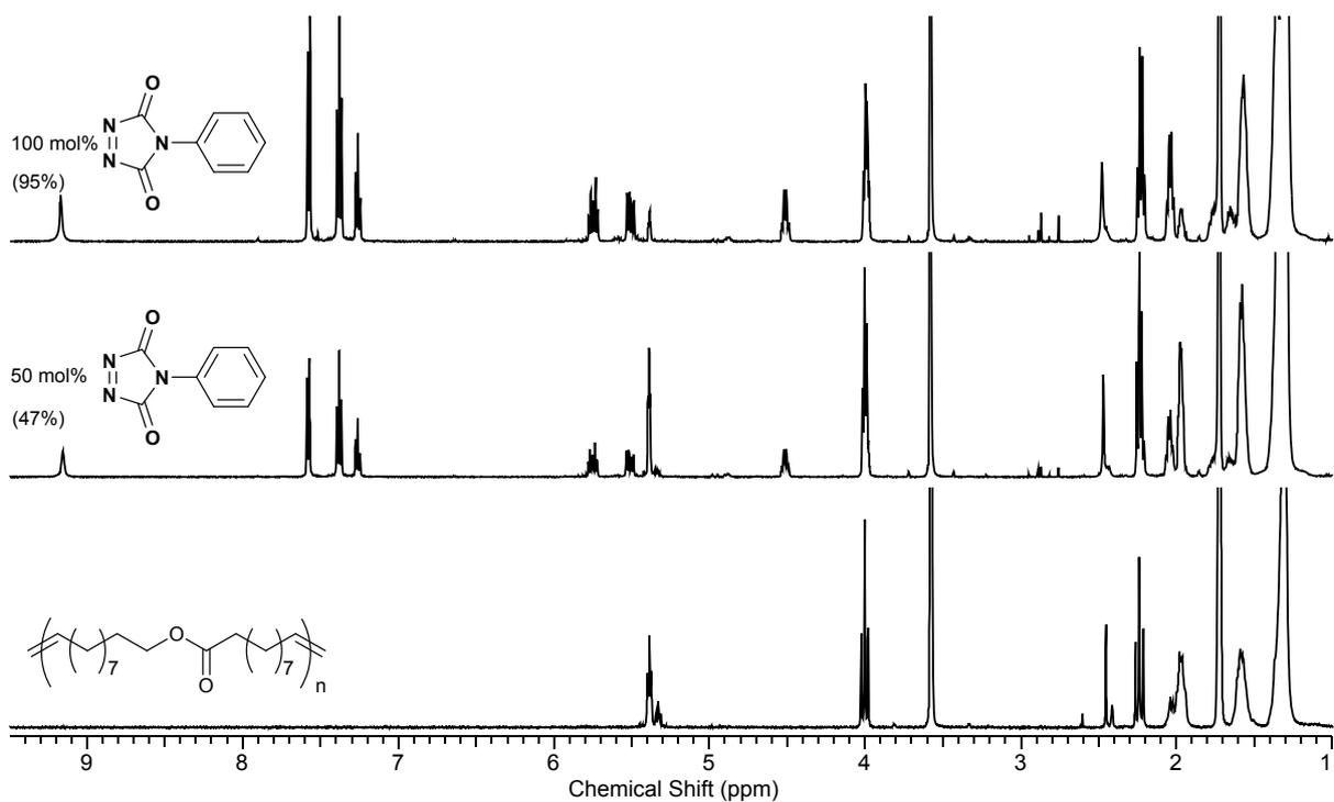
Figure S 10 - Modification of P3 with PhTAD – NMR spectra in THF- $d_8$  with targeted and experimentally observed (between brackets) functionalisation degree.
