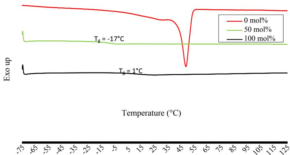
Figure S 8 - Modification of P1 with BuTAD - DSC data.
