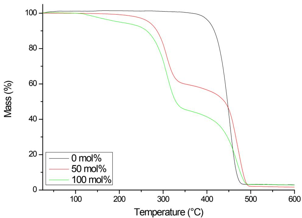
Figure S 7 - Modification of P1 with BuTAD - TGA thermograms.
