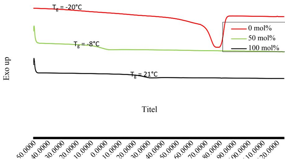
Figure S 17 - Modification of P4 with PhTAD – DSC data.
