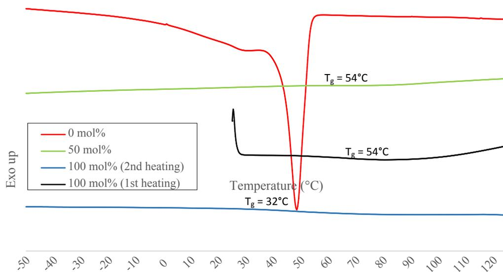
Figure S 22 - Functionalisation of P1 with  $\text{COOH}$ -PhTAD - DSC data.
