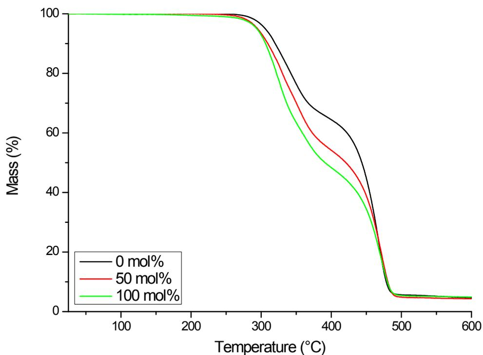
Figure S 14 - Modification of P4 with PhTAD – TGA thermograms.
