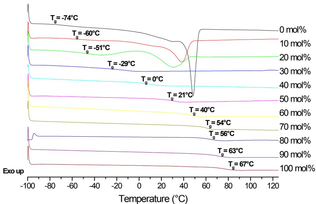
Figure S 5 - Raw DSC data of the systematically modified polymers with modification degrees ranging from 0 mol% PhTAD to 100 mol% PhTAD. An increasing  $T_g$  and decreasing crystallinity with increasing degree of modification are observed.
