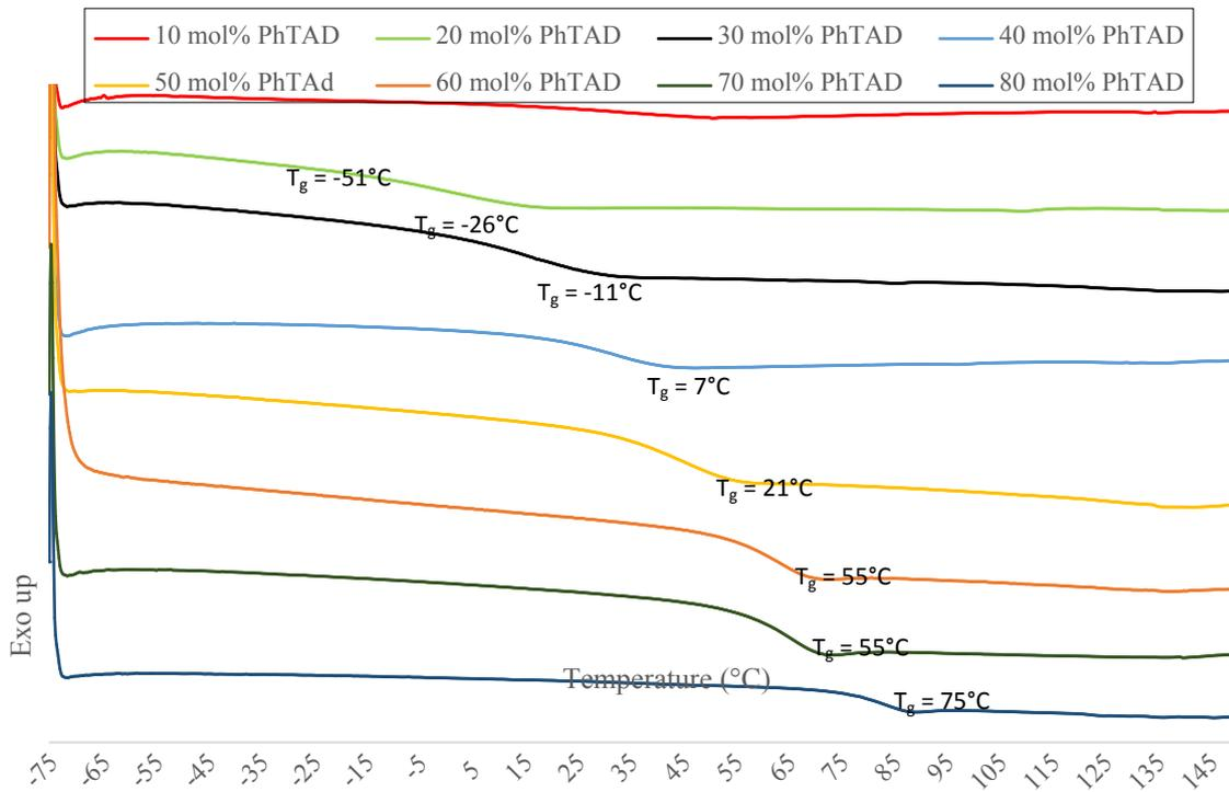
Figure S 24 – DSC analysis of PhTAD modified P1 crosslinked with 5 mol% MDI-TAD.
