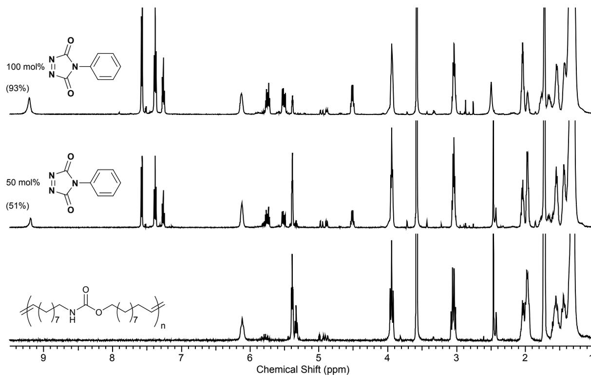
Figure S 11 - Modification of P4 with PhTAD – NMR spectra in THF- $d_8$  with targeted and experimentally observed (between brackets) functionalisation degree.
