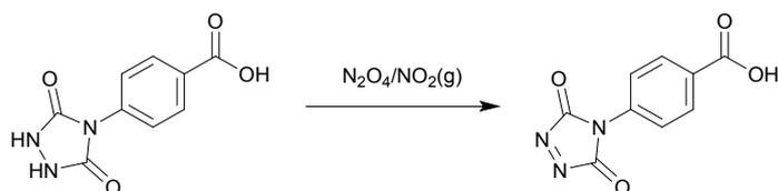
In a 250 mL flask, 4-(3,5-dioxo-1,2,4-triazolidin-4-yl)benzoic acid (0.7 g, 3.2 mmol, 1 eq.) was suspended in 100 mL of dried ethyl acetate. 5 g (excess) Na<sub>2</sub>SO<sub>4</sub> was added, the mixture was cooled to 0°C and gaseous NO<sub>2</sub> was bubbled through the solution for 15 minutes, until no further change in colour was observed. Excess of NO<sub>2</sub> was removed by a stream of argon. The
