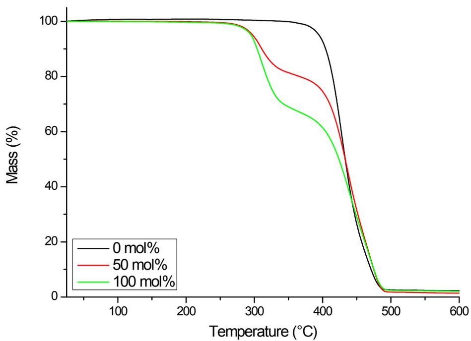
Figure S 13 - Modification of P3 with PhTAD – TGA thermograms.
