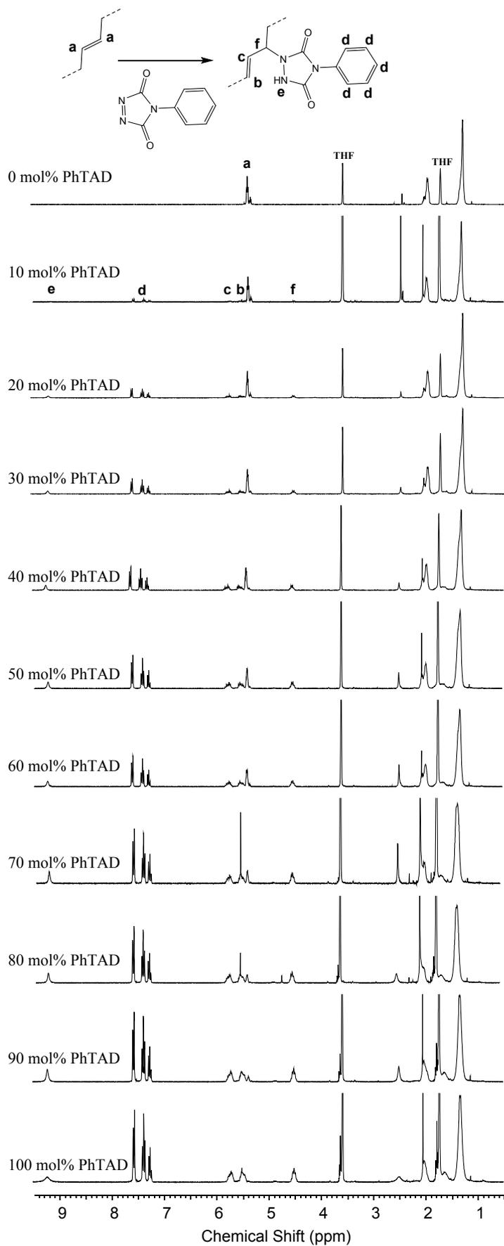
Figure S 2 - Full spectra of the systematic modification of P1 with PhTAD (THF-d<sub>8</sub>).
