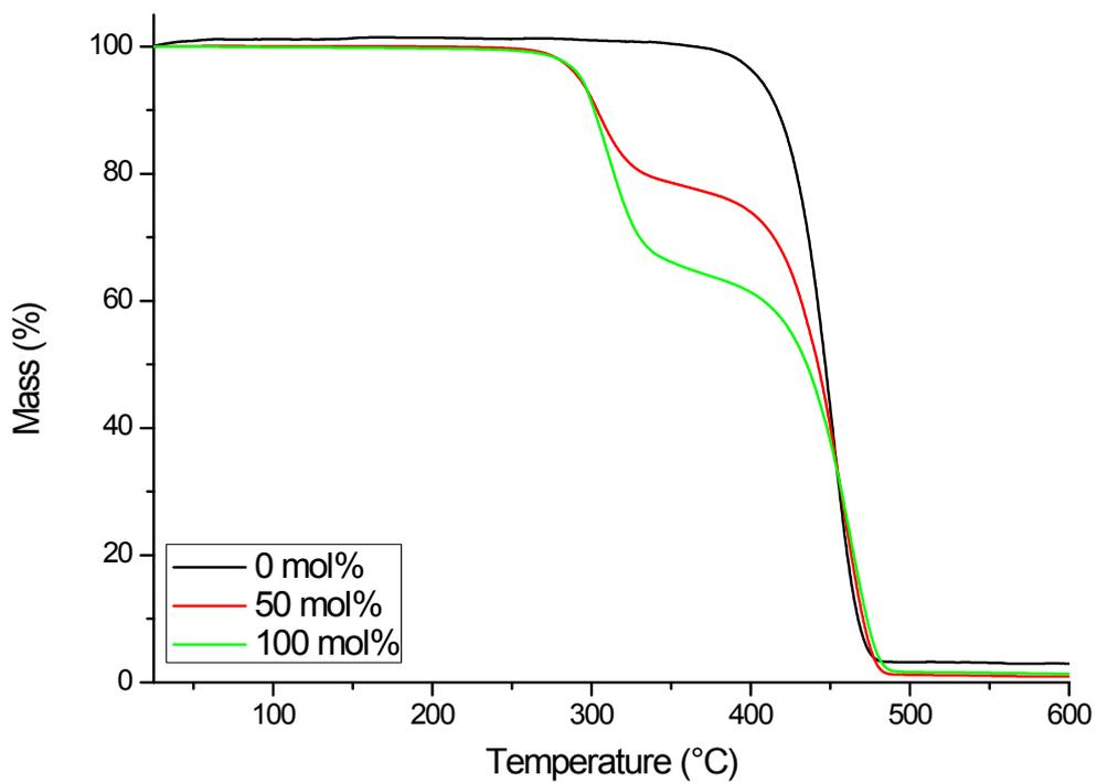
Figure S 12 - Modification of P2 with PhTAD – TGA thermograms.
