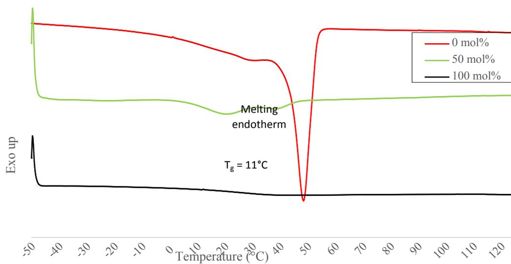
Figure S 21 - Functionalisation of P1 with  $\text{NO}_2$ -PhTAD – DSC data.
