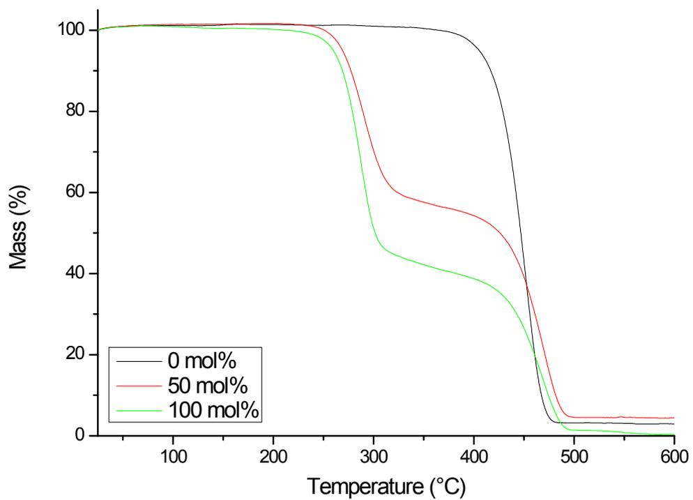
Figure S 19 - Functionalisation of P1 with NO<sub>2</sub>-PhTAD - TGA thermograms.
