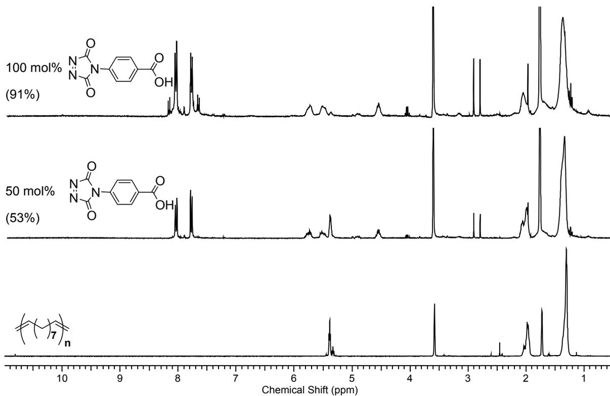
Figure S 18 - Functionalisation of P1 with COOH-PhTAD - NMR data (THF- $d_8$ ). The COOH and urazole protons can only be seen upon zooming.
