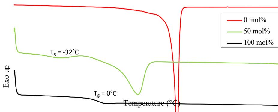
Figure S 16 - Modification of P3 with PhTAD – DSC data.
