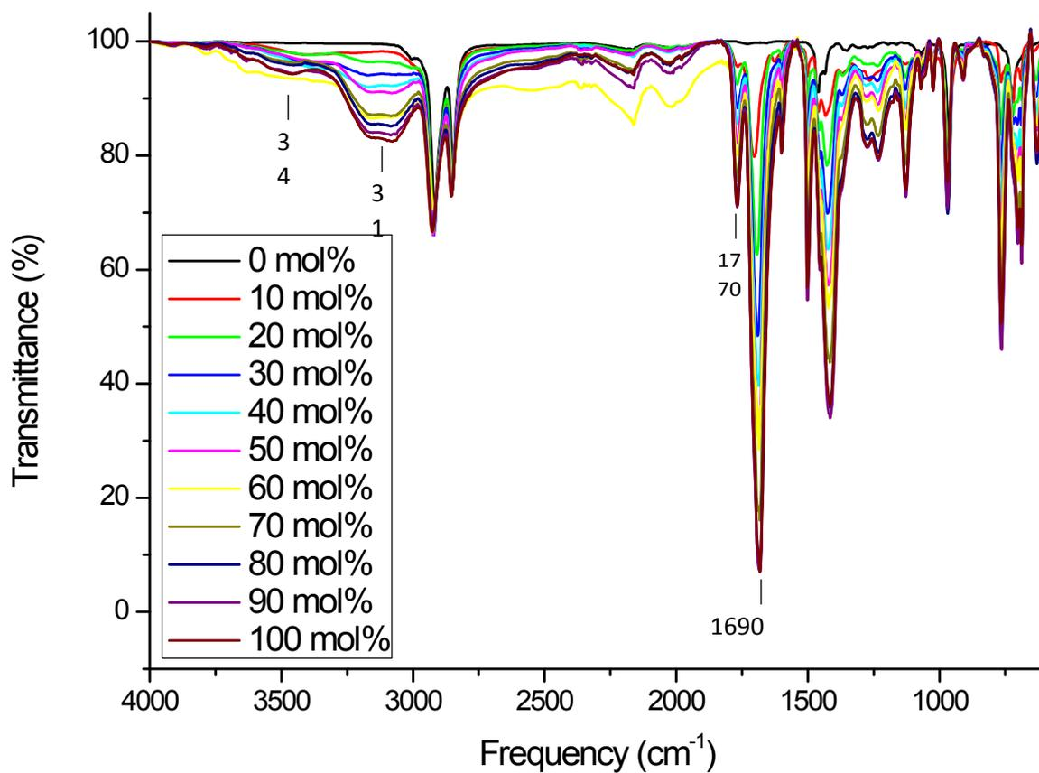
Figure S 3 - IR-spectra of the systematic modification of P1 with PhTAD with varying degrees of modification. Increasing modification leads to the increase of C=O stretches (1690 cm<sup>-1</sup> and 1770 cm<sup>-1</sup>) and N-H stretches (3400 cm<sup>-1</sup> and 3140 cm<sup>-1</sup>).
