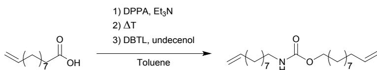
15.9 g 10-undecenoic acid (0.087 mol, 1 eq.) was solubilized in 250 mL toluene and mixed with triethylamine (24.1 mL, 0.173 mol, 2 eq.) in a 500 mL flask. Diphenylphosphoryl azide (25
