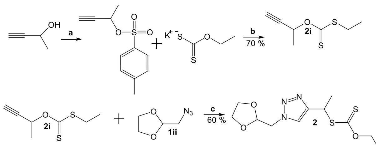
**Scheme S2. Synthesis of RAFT agent **2**;** (a) *p*-Tosyl chloride, KOH, diethyl ether, 0 °C to r.t.; (b) THF, r.t.; (c) CuSO<sub>4</sub>·5H<sub>2</sub>O, sodium ascorbate, DMF, r.t
