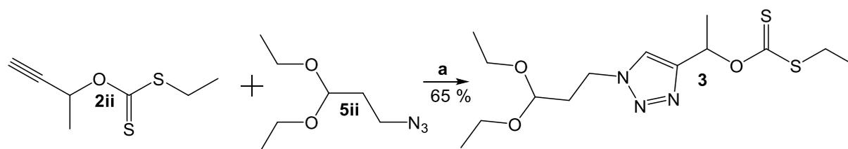
**Scheme S5. Synthesis of RAFT agent X;** (a) CuSO<sub>4</sub>·5H<sub>2</sub>O, sodium ascorbate, DMF, r.t.
