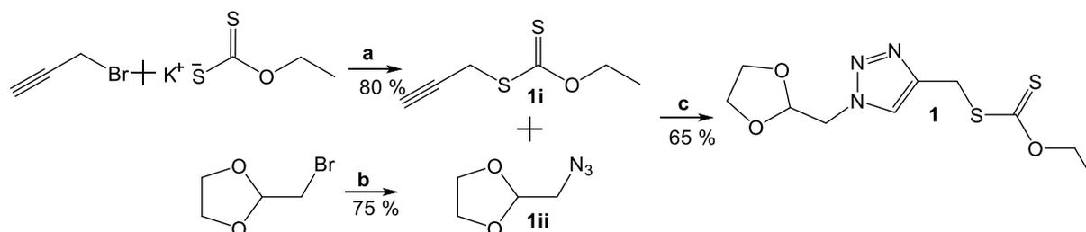
**Scheme S1. Synthesis of RAFT agent 1;** (a) THF, r.t.; (b) NaN<sub>3</sub>, DMSO, 100 °C; (c) CuSO<sub>4</sub>·5H<sub>2</sub>O, sodium ascorbate, DMF, r.t
