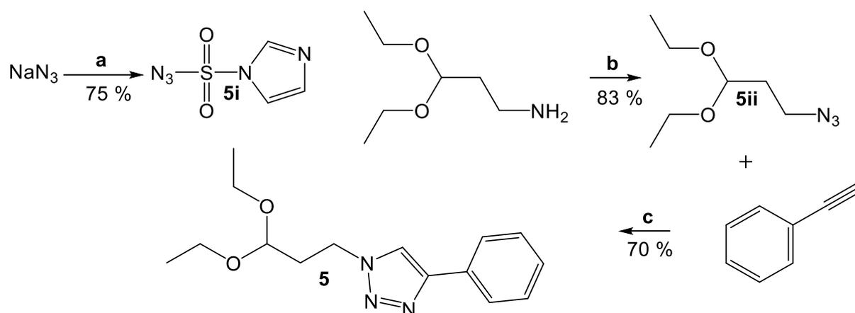
**Scheme S4. Synthesis of model acetal 5;** (a) (i)  $\text{SO}_2\text{Cl}_2$ , MeCN, r.t. (ii) imidazole 0  $^\circ\text{C}$  to r.t., (b)  $\text{K}_2\text{CO}_3$ ,  $\text{CuSO}_4 \cdot 5\text{H}_2\text{O}$ , **5i**, MeOH, r.t. (c)  $\text{CuSO}_4 \cdot 5\text{H}_2\text{O}$ , sodium ascorbate, DMF, r.t.
