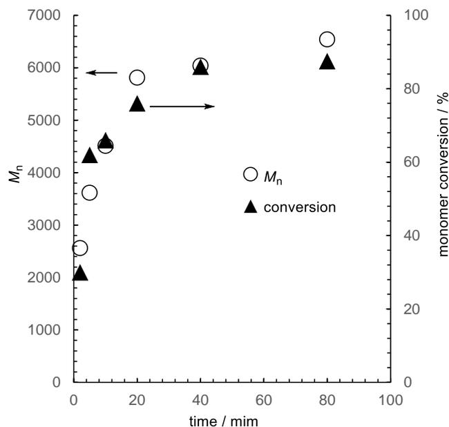
**Fig. S1** Plots of time vs  $M_n$  and monomer conversion in the polymerization of **1b**.
