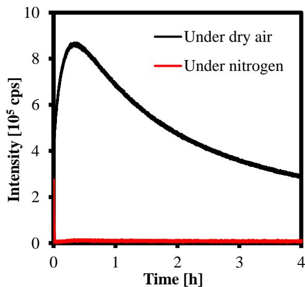
**Figure S2.** Chemiluminescence profiles of silkworm silk powder at 200 °C under dry air and nitrogen.
