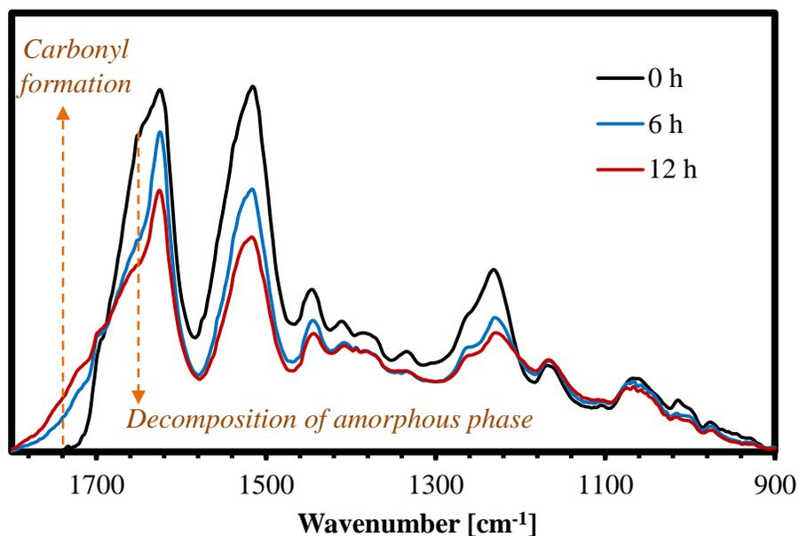
**Figure S3.** ATR-IR spectra for silkworm silk before and after degraded at 200 °C under dry air for 6 and 12 hours.
