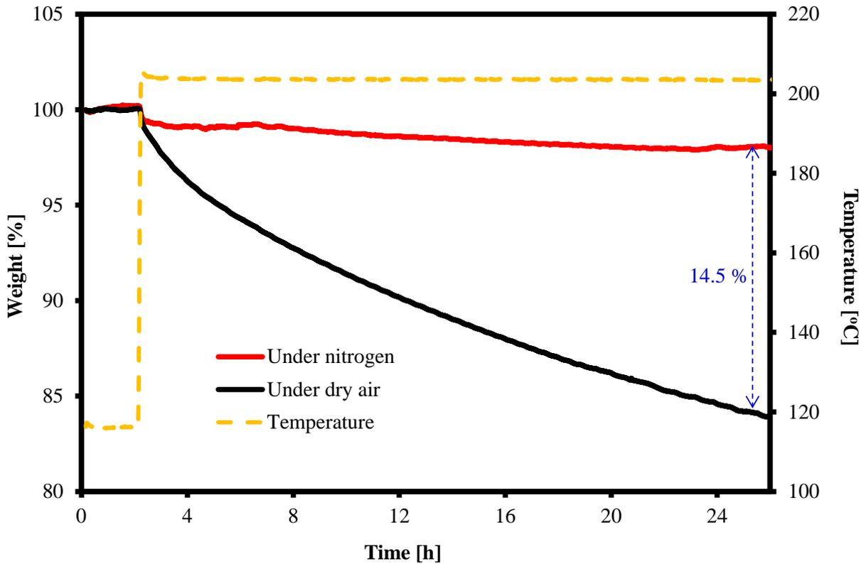
**Figure S1.** TGA curves of silkworm silk powder in an isothermal mode at 110 °C for 2 hours to remove free water and at 200 °C for 24 hours to promote the degradation.
