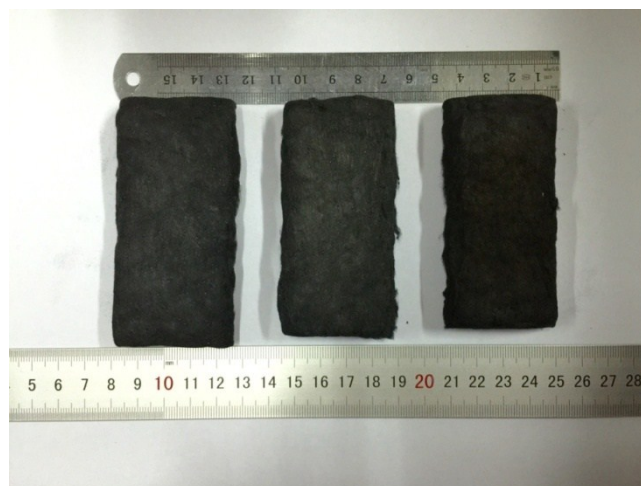
Fig. S1 Digital photo of HCFSs prepared under 500, 700 and 900 °C from left to right.
