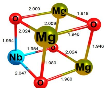
$\text{Mg}_3\text{NbO}_4-1\text{H}_2$  ( $\text{H}_2$  towards Nb)
