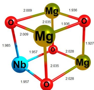
$\text{Mg}_3\text{NbO}_4-1\text{H}_2$  ( $\text{H}_2$  towards Mg)
