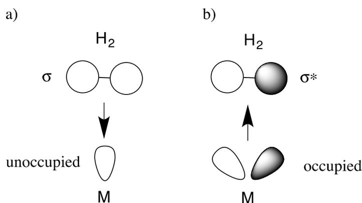
Fig. S2. (a) Electron donation from and (b) back-donation to the hydrogen molecule.
