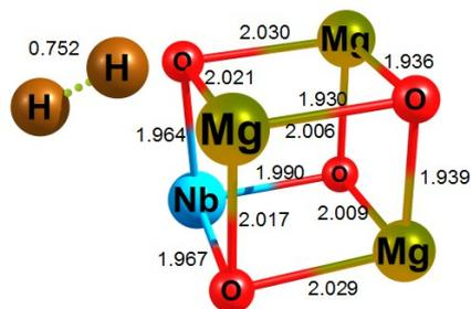
$\text{Mg}_3\text{NbO}_4-3\text{H}_2$  (one  $\text{H}_2$  towards Mg)
