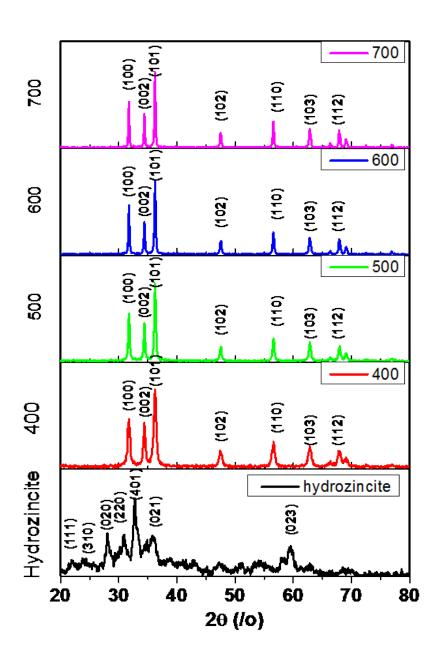
The average crystalline size calculated by Scherrer equation using the (101) peak is 16.1, 25.1, 31.0, and 35.9 nm, respectively.
