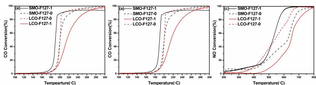
Fig. S3 (a) CO, (b) C<sub>3</sub>H<sub>8</sub>, (c) NO conversion of the oxides as a function of temperature under the simulated exhaust gas. (CO/NO/C<sub>3</sub>H<sub>8</sub>/O<sub>2</sub>/N<sub>2</sub> = 2.0/0.2/0.05/1.0/96.75)
