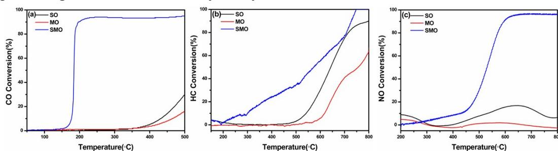
Fig. S4 (a) CO, (b) C<sub>3</sub>H<sub>8</sub>, (c) NO conversion for SO, MO and SMO oxides as a function of temperature under the simulated exhaust gas. (CO/NO/C<sub>3</sub>H<sub>8</sub>/O<sub>2</sub>/N<sub>2</sub> = 2.0/0.2/0.05/1.0/96.75)
