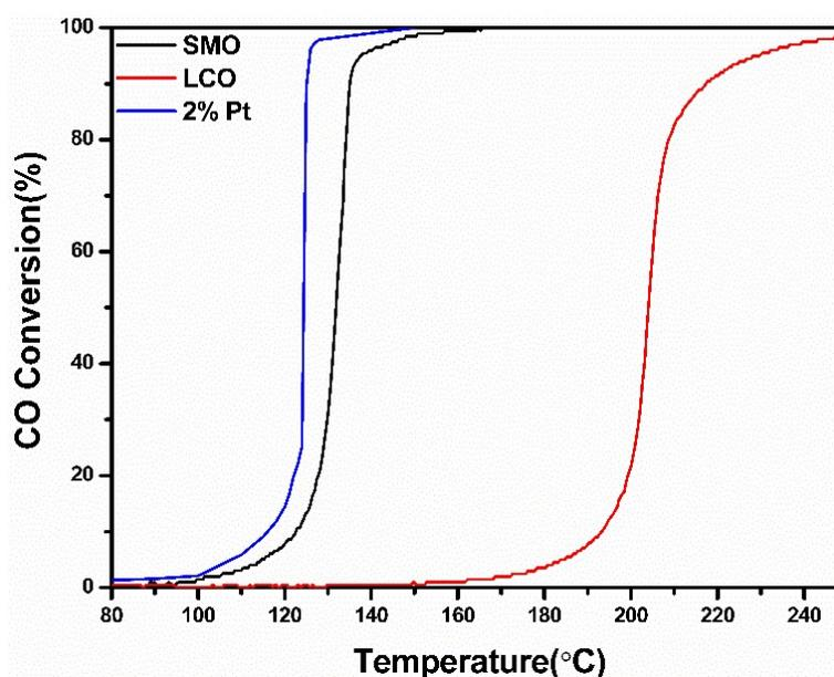
Fig. S2 The CO conversion as a function of temperature for the prepared samples.
