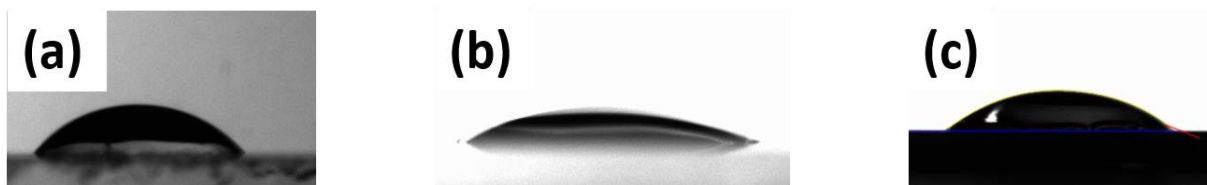
Fig. S3 Contact angle measurements for: (a) bare glass, (b) pSBMA-H and (c) pSBVI-H.
