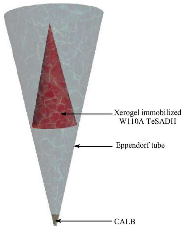
**Figure S2.** Reaction set-up for dual enzymatic DKR of phenyl-ring-containing secondary alcohols.
