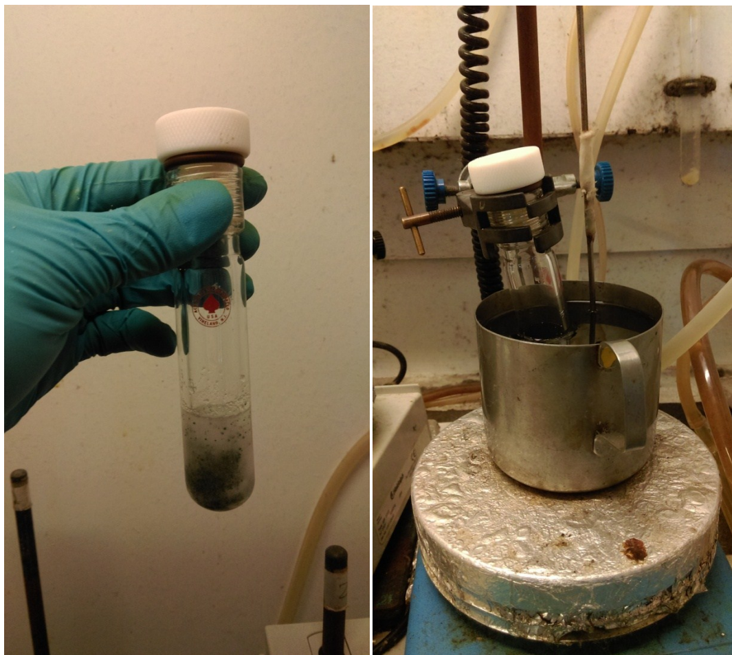
Figure S4. 15 mL, Aldrich Z181064 glass pressure reactor charged with the reaction mixture and experiment set up.
