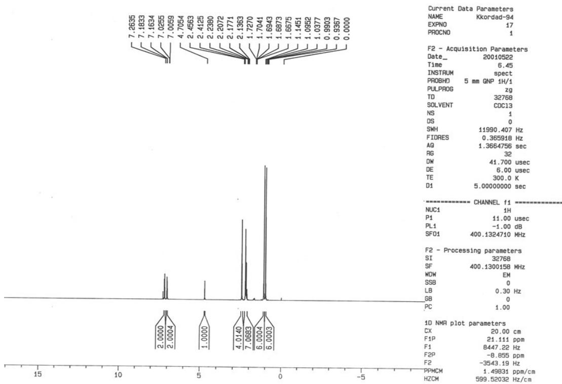
Fig.28. <sup>1</sup>H-NMR spectrum of 3,3,6,6-tetramethyl-9-(p-tolyl)-3,4,5,6,7,9-hexahydro-1H-xanthene-1,8(2H)-dione in DMSO (Table 5, entry 14).
