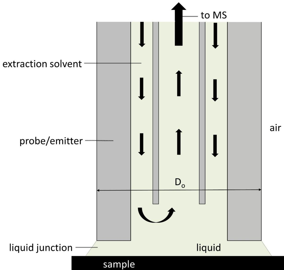
**Fig. S1.** Schematic illustration of a junction region from a flowprobe™-MS experimental setup with  $D_o = 630 \mu\text{m}$  ( $D_o$ : probe outer diameter).
