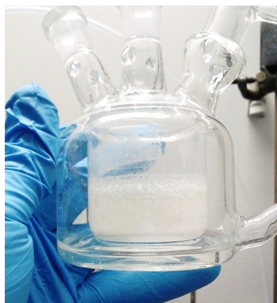
Figure S2. K_2CO_3 precipitation on the inner wall of the reactor after an experiment
