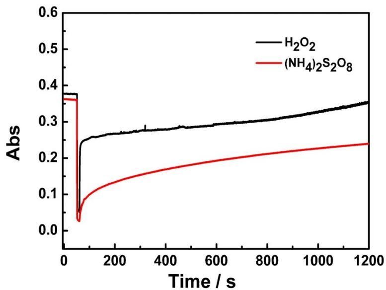
Fig. S3 In situ absorbance measurement of the Mg/PB battery connected at 50 s and then disconnected at 60 s. The red curve referred to the electrolyte containing 0.025 M (NH<sub>4</sub>)<sub>2</sub>S<sub>2</sub>O<sub>8</sub>, 1 M KCl and 0.1 M phosphate buffer (pH 6), and the black curve referred to the electrolyte containing 0.025 M H<sub>2</sub>O<sub>2</sub>, 1 M KCl and 0.1 M phosphate buffer (pH 6).
