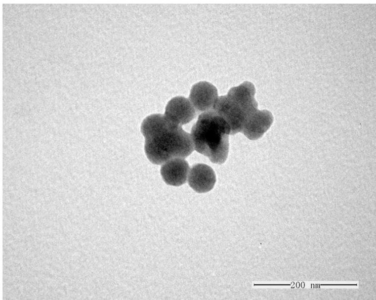
Fig. S5. TEM of the Ru@SiO<sub>2</sub> nanoparticle.
