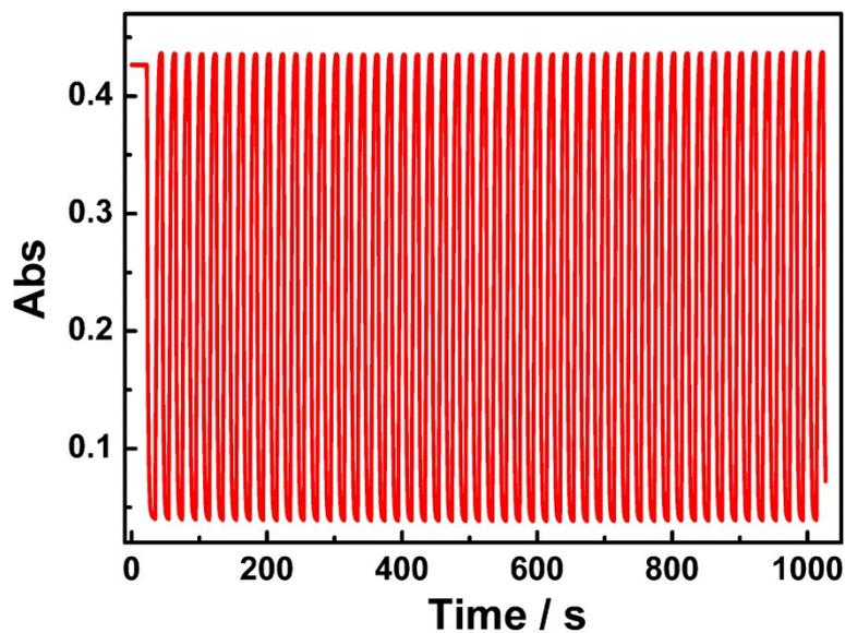
Fig. S2. Absorption (700 nm) response of the PB film versus time during consecutive switch cycles (0 V/0.4 V, 10 s) in 1 M KCl and 0.1 M phosphate buffer (pH 6) electrolyte solution.
