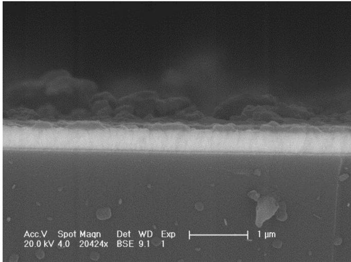
Fig. S8. The SEM of the section of the PB/Ru@SiO<sub>2</sub>/Nafion film.
