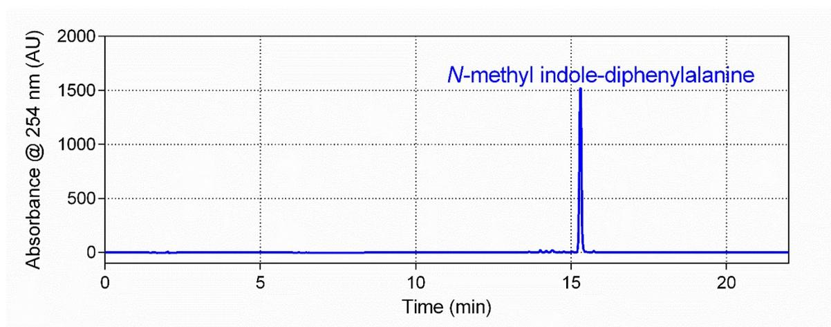
**Figure S1** – HPLC trace of *N*-methylindole-diphenylalanine, **2**.
