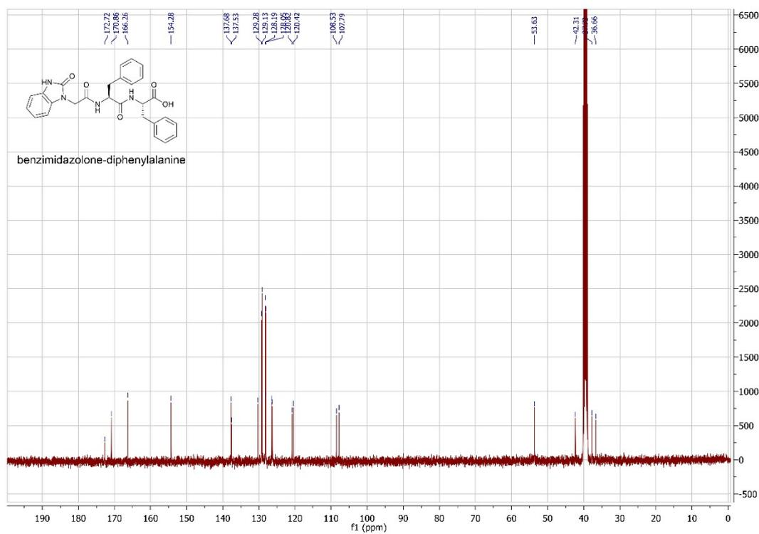
Figure S4 – <sup>13</sup>C NMR Spectra of benzimidazolone-diphenylalanine, 3.
