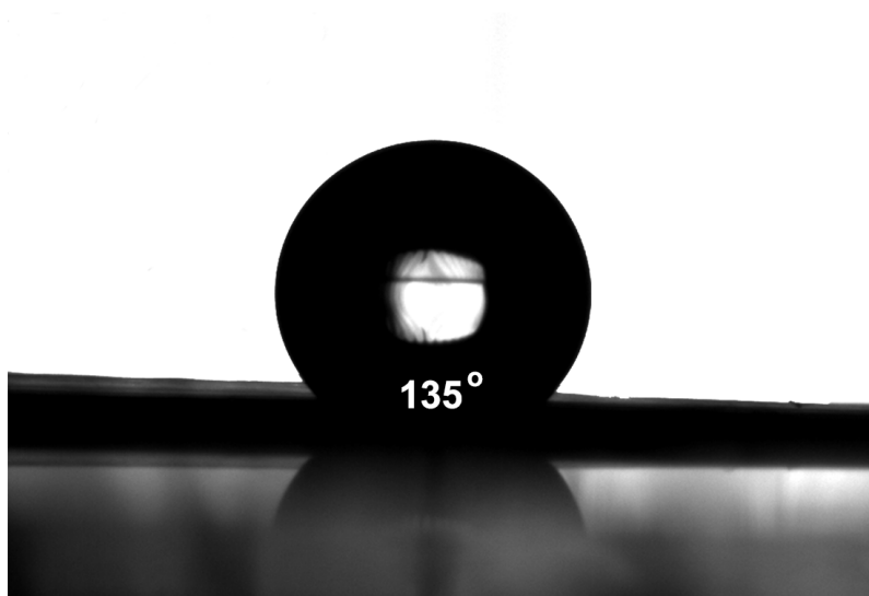
Figure S10. A water droplet on an aligned CNT sheet.
