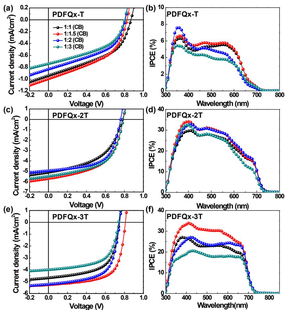
**Fig. S5** a), c), e) J-V characteristics and b), d), f) IPCE curves for PDFQx-T:PC<sub>71</sub>BM, PDFQx-2T:PC<sub>71</sub>BM, and PDFQx-3T:PC<sub>71</sub>BM devices with changing blend ratios. The processing solvent is chlorobenzene (CB).
