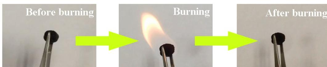
**Fig. S6** Photographs showing the generation of oPP-33.3 carbon aerogel via combustion.
