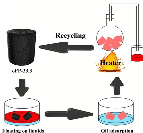
**Fig. S7** The recycling process of oPP-33.3 carbon aerogel after its adsorption of acetone.
