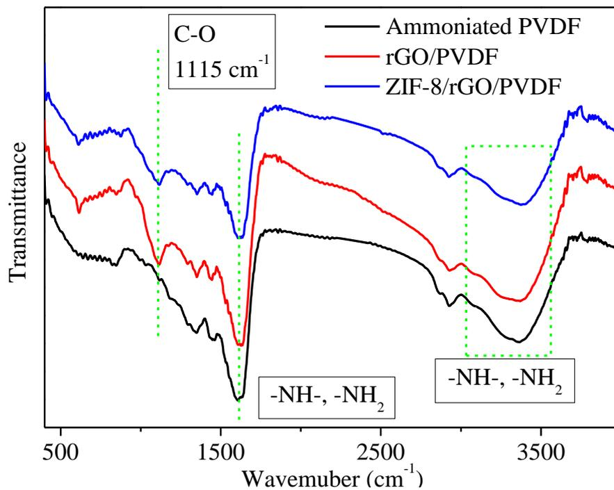
**Figure S3.** FTIR spectra of aminated PVDF hollow fiber, rGO membrane and ZIF-8/rGO membrane.
