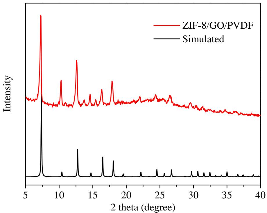
**Figure S5.** XRD patterns of simulated ZIF-8 and ZIF-8/rGO membranes. The characteristic peaks in XRD pattern demonstrate that the prepared membrane contains the ZIF-8 materials.
