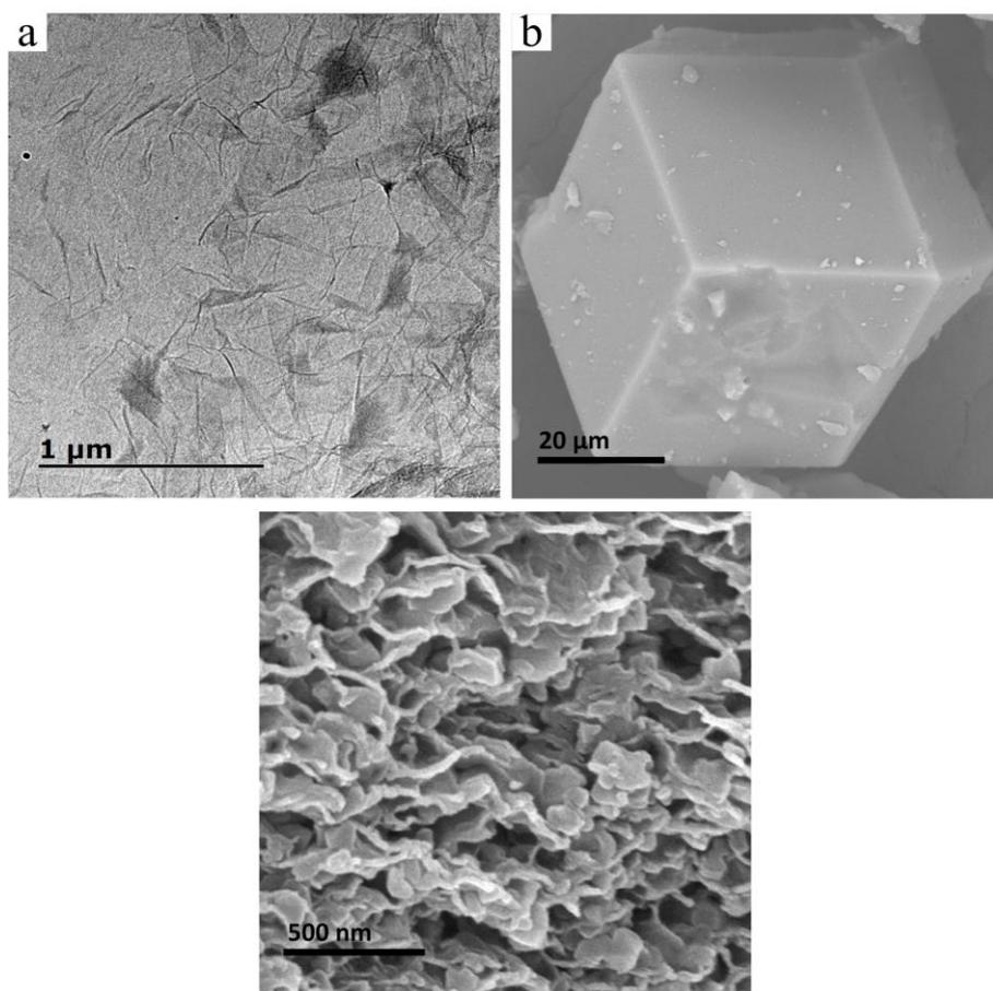
**Figure S1.** (a) TEM image of GO sheets synthesized by Hummer's method. (b) SEM image of ZIF-8 synthesized by solvothermal method. (c) SEM image of ZIF-8/rGO composite.
