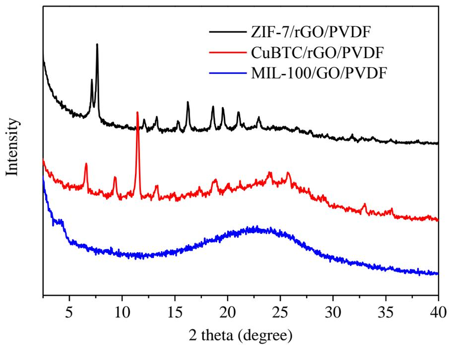
**Figure S10.** XRD patterns of ZIF-7/rGO, CuBTC/rGO and MIL-100/rGO membranes.
