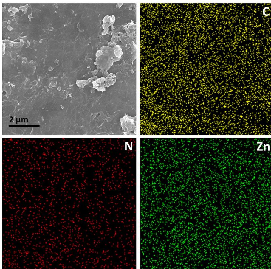
**Figure S7.** EDS mapping images of inner ZIF-8/rGO membrane. It indicates that ZIF-8 is dispersed in the whole membrane uniformly.
