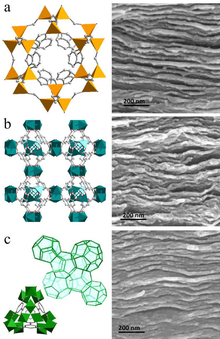
**Figure S9.** Cross-sectional SEM images and crystalline structure of (a) ZIF-7/rGO, (b) CuBTC/rGO and (c) MIL-100/rGO membranes
