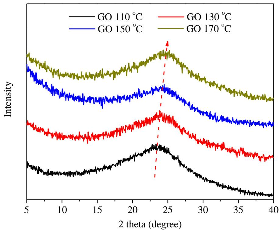
**Figure S4.** XRD patterns of rGO membranes synthesized at different temperature.
