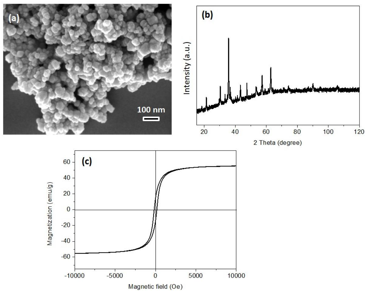
**Figure S1.** SEM image (a), powder X-ray diffraction pattern (b), and magnetic hysteresis loop of HP-passivated  $\text{Fe}_3\text{O}_4$  nanoparticles.
