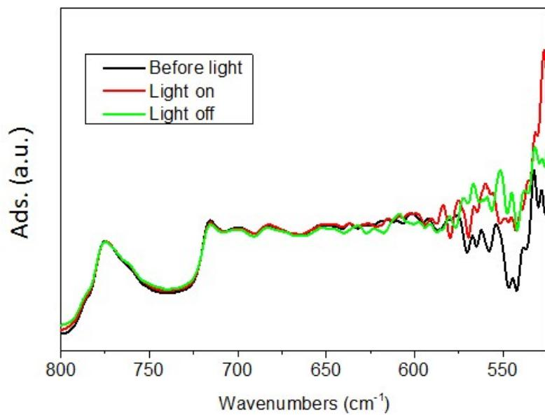
**Figure S3.** Time resolved FT-IR spectra of mPCN-M before and after irradiation with 365 nm of UV light.
