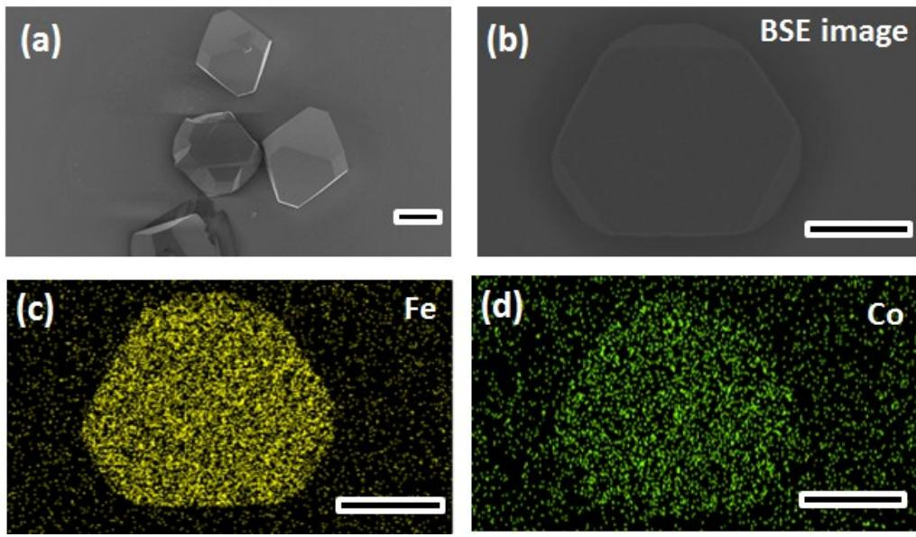
**Figure S2.** SEM images of bare PCN-250 crystals (a); BSE image (b), Fe (b) and Co (c) elemental mapping of a selective PCN-250 crystal. The scale bars are 100  $\mu\text{m}$ .
