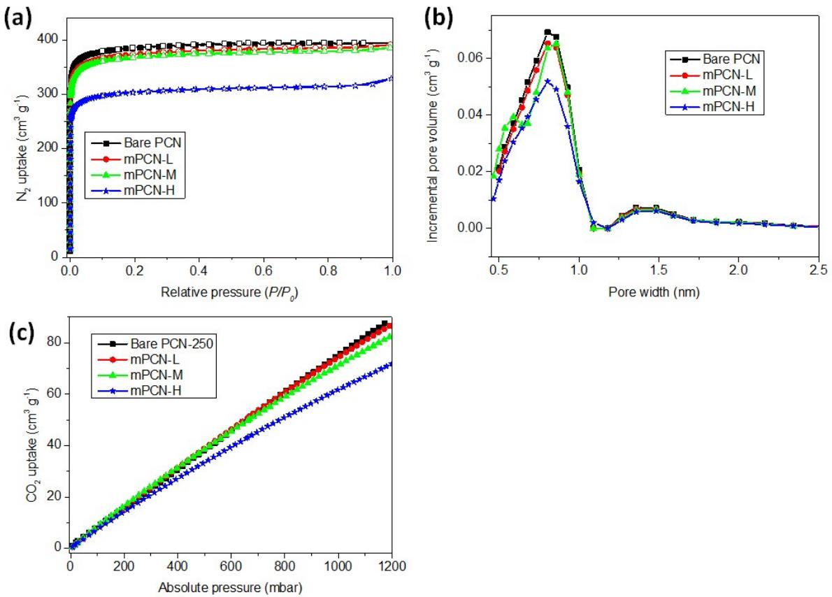
**Figure S4.** N<sub>2</sub> adsorption isotherms at 77.3 K (a), pore size distributions (b), and CO<sub>2</sub> adsorption isotherms at 298 K of bare PCN-250 and mPCNs with different magnetic nanoparticle content (c).
