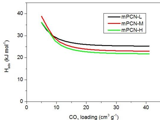
**Figure S5:** Isosteric heat of adsorption as a function of  $\text{CO}_2$  uptake of mPCN.
