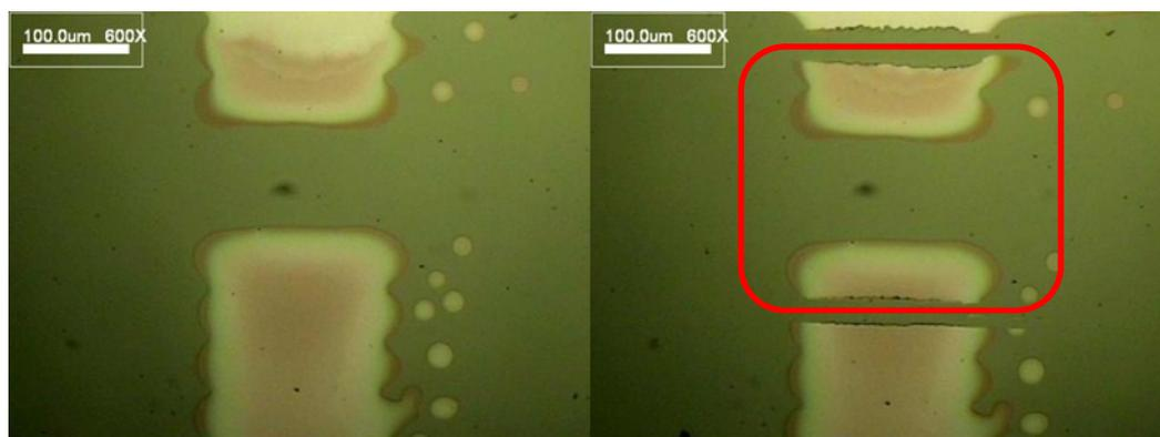
Fig. S1. Microscopic images of the fabricated SWCNT-TFT. The channel area of the TFT was mechanically patterned using a sharp tip. (left: before the patterning process, right: after the patterning process)
