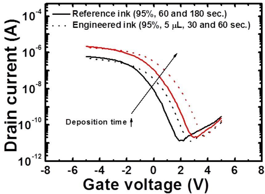
Fig. S3 Transfer characteristics of the solution-processed SWCNT-TFTs fabricated by using the reference ink (95%-purified, deposition times of 60 and 180 seconds: solid line) and 4M nitric acid (5  $\mu$ L)-added ink (95%-purified, deposition times of 30 and 60 seconds: dotted line)
