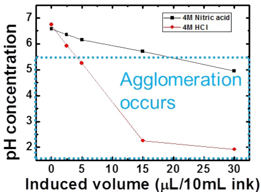
Fig. S2. pH concentration variations of the engineered inks as a function of induced acid volume in commercial SWCNT ink (10 mL). When pH concentration of the engineered ink is 5.0~5.5, large SWCNT agglomeration occurs.
