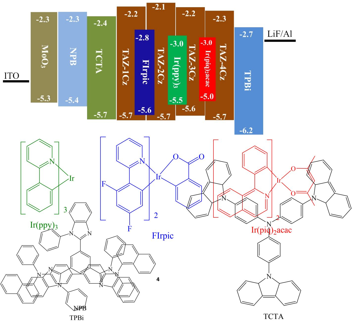
Fig. S4 The energy level and chemical structures of the all materials
