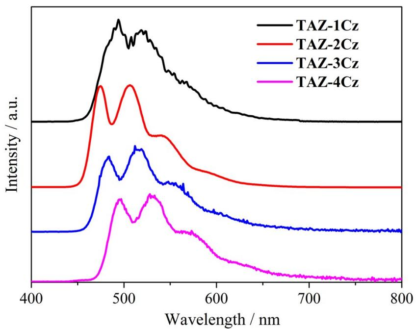
Fig. S2 Phosphorescent spectra in a frozen 2-methyltetrahydrofuran matrix at 77 K
