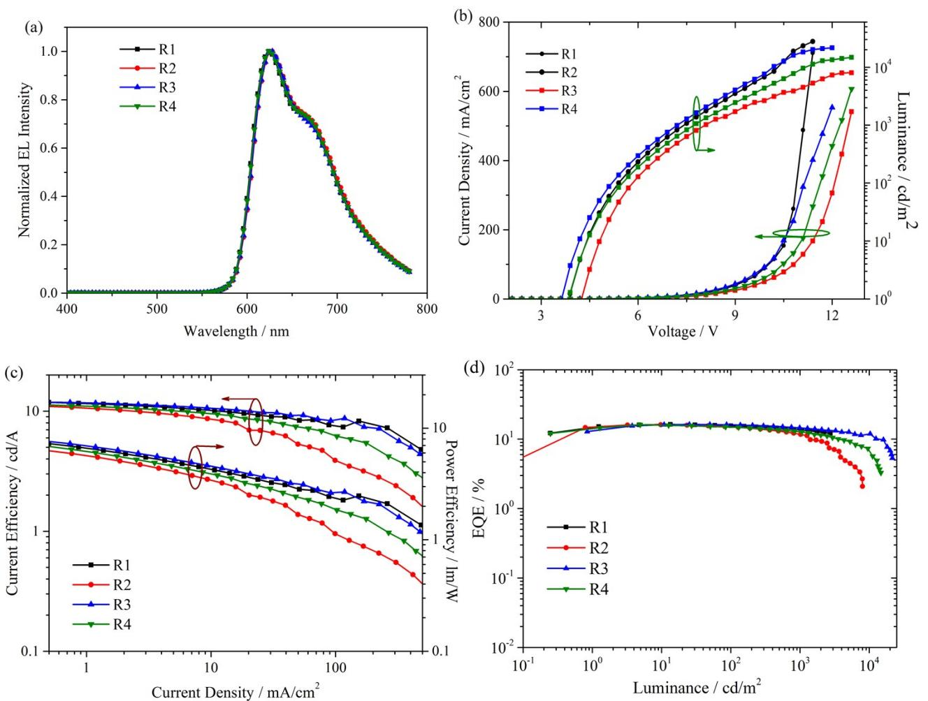
Fig. S6. (a) EL spectra of devices, (b) J-V-L characteristics, (c)  $\eta_c - \eta_p$  curves and (d) EQE
