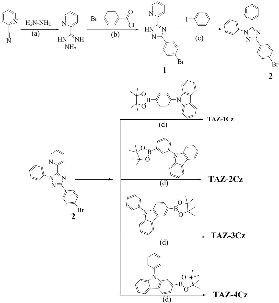
Scheme S1. Synthetic scheme of the all four bipolar materials. (a) EtOH, 8 h,  $\text{N}_2$ ; (b)  $\text{NaCO}_3$ , DMAC, Ethylene, glycol, 6 h,  $\text{N}_2$ ; (d) Phen,  $\text{CuI}$ ,  $\text{Cs}_2\text{CO}_3$ , DMF, Reflux; 24 h,  $\text{N}_2$ ; (e)  $\text{Pd}(\text{pph}_3)_4$ ,  $\text{NaCO}_3$ , THF, reflux, 24 h,  $\text{N}_2$
