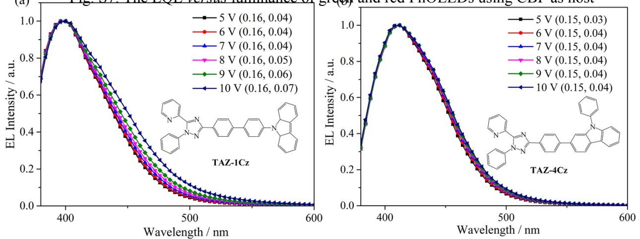
Fig. S8 The EL spectra and CIE coordination under the different voltages
