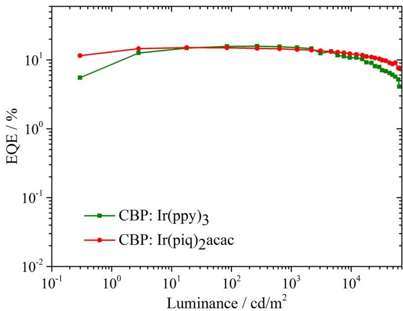
(a) Fig. S7. The EQE *versus* luminance of green and red PhOLEDs using CBP as host
