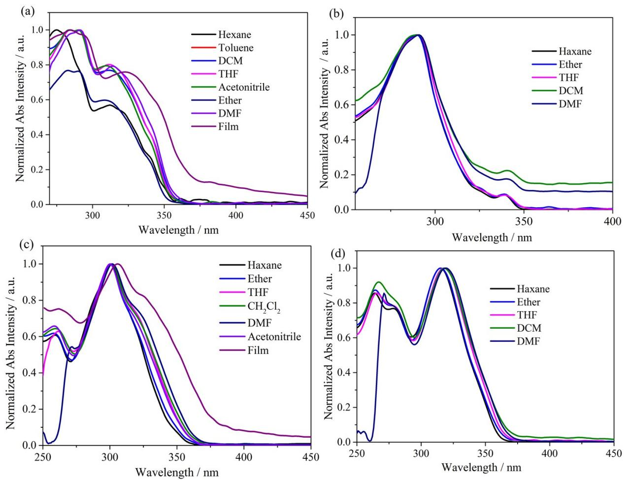
Fig. S1 Absorption spectra of host materials in different polarity solvents (a) **TAZ-1Cz**, (b) **TAZ-2Cz**, (c) **TAZ-3Cz** and (d) **TAZ-4Cz**
