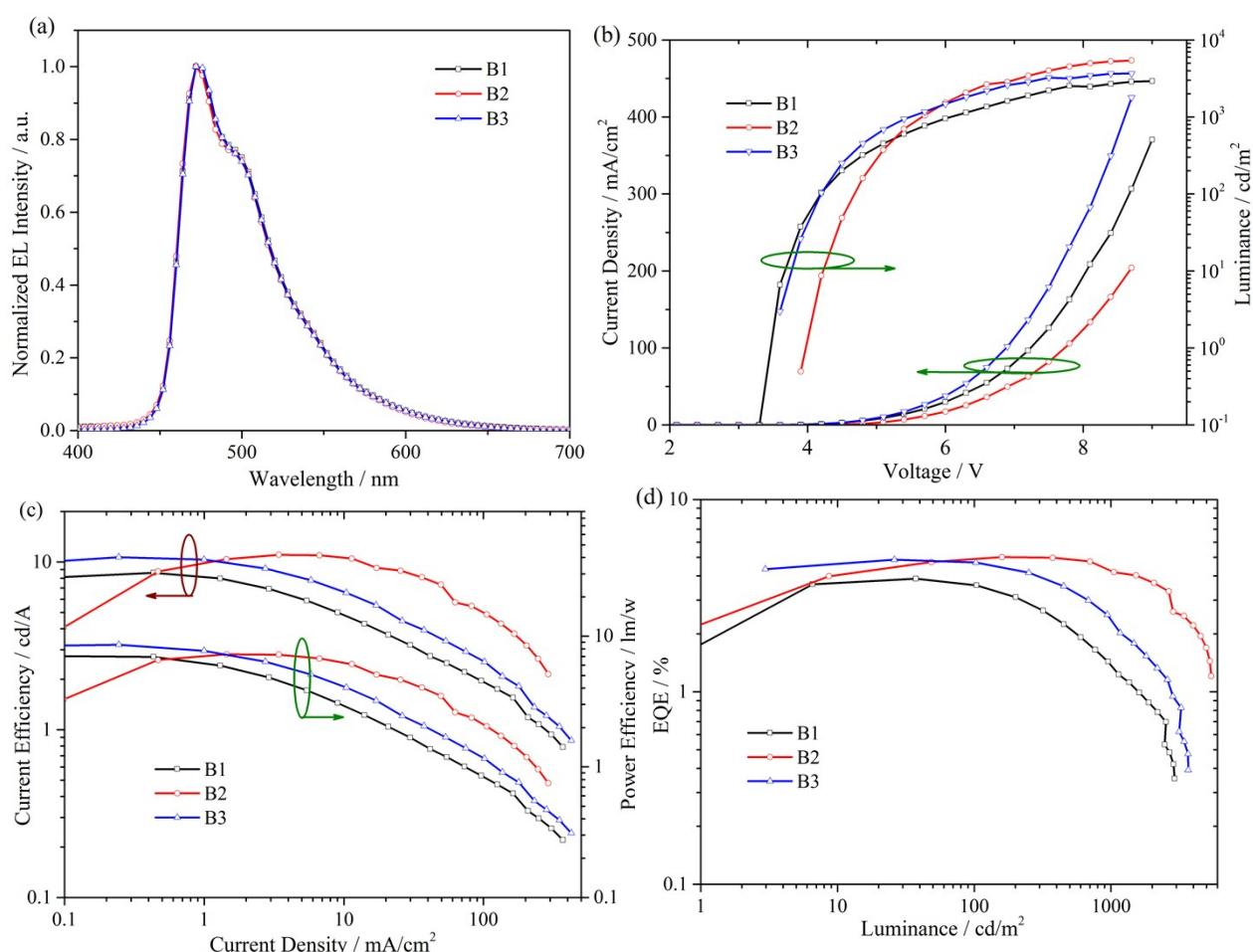
Fig. S5. (a) EL spectra of devices, (b) J-V-L characteristics, (c)  $\eta_c - J - \eta_p$  curves and (d) EQE *versus* luminance for blue devices B1-B3 with the 1, 2, 4-trizole derivatives host.
