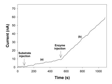
**Figure S1**. Spontaneous (a) and enzymatic (b) substrate hydrolysis. Supporting electrolyte: phosphate buffer pH 8.5, I 0.1 M. Substrate: butyrylcholine 1.75 mM. Enzyme: BChE 1 U L<sup>-1</sup>. Electrode rotation rate: 200 rpm.
