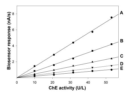
**Figure S3** Calibration curves for various ChE/substrate couples: AChE/acetylcholine (A); BChE/butyrylcholine (B); BChE/s-butyrylthiocholine (C); BChE/benzoylcholine (D); BChE/acetylcholine (E). Substrate concentration: 1 mM. Supporting electrolyte: phosphate buffer pH 7.8, I 0.1 M. Temperature: 25 °C. Electrode rotation rate: 200 rpm.
