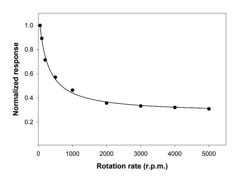
**Figure S2**. Variation of the current signal slopes as a function of the rotation rate at a Pt/PPyox/ChO biosensor upon addition of acetylcholine 1 mM and AChE 10 U L<sup>-1</sup>. Supporting electrolyte: phosphate buffer pH 7.8, I 0.1 M. Temperature: 25 °C.
