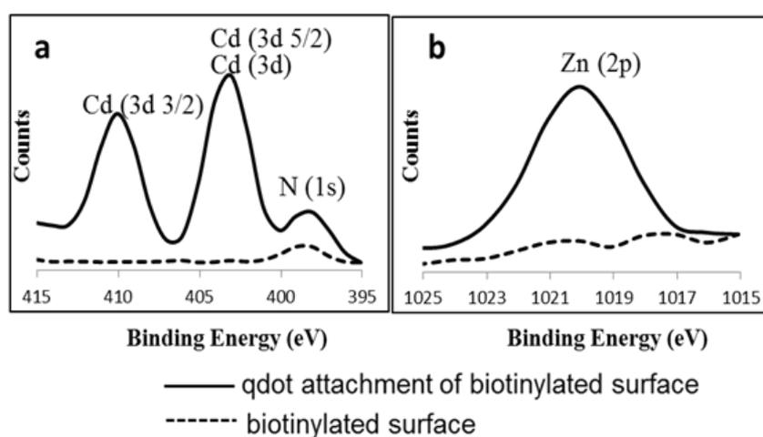
**Figure S6.** XPS Spectra of patterned hydrogel H3 (a) Binding energy of Cd and N on biotinylated surface and after attachment of streptavidin conjugated QDs. (b) Binding
