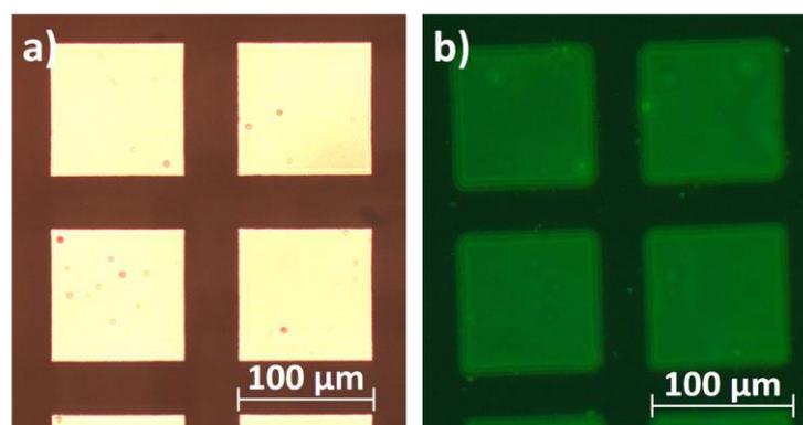
**Figure S4.** a) Optical microscope image of photomask and b) fluorescence microscope image of dye immobilized patterns.
