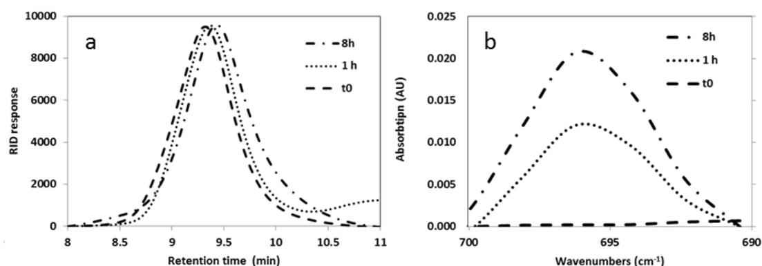
**Figure S5.** a) GPC Spectrum of polymers  $t_0$ : before retro, after 1 h of r-DA, and after 8 h of r-DA. b) C-H (Double bond) stretching of polymers in IR spectra,  $t_0$ : before retro, after 1 h of r-DA, and after 8 h of r-DA.
