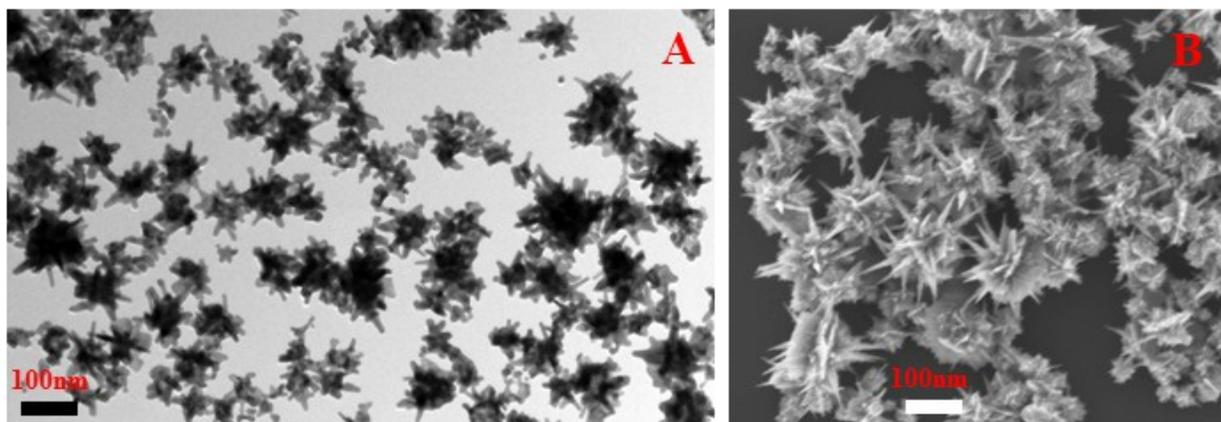
**Figure S2:** (A) Large area TEM and (B) SEM image of HHogGNPs synthesized by using 10mM NaCl in the mother solution.
