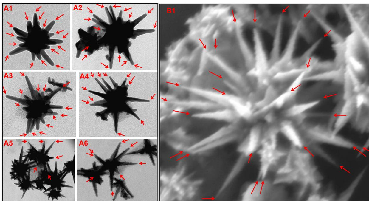
**Figure S6:** (A<sub>1</sub>-A<sub>6</sub>) are TEM images of HHogGNPs synthesized at different NaCl concentration: A<sub>1</sub> – 170 $\mu$ M, A<sub>2</sub> – 340 $\mu$ M, A<sub>3</sub> – 1.7mM, A<sub>4</sub> – 3.4mM, A<sub>5</sub> – 10mM, A<sub>6</sub> - 20mM and B1 is the SEM image of a HHogGNP synthesized in presence of 10mM NaCl.
