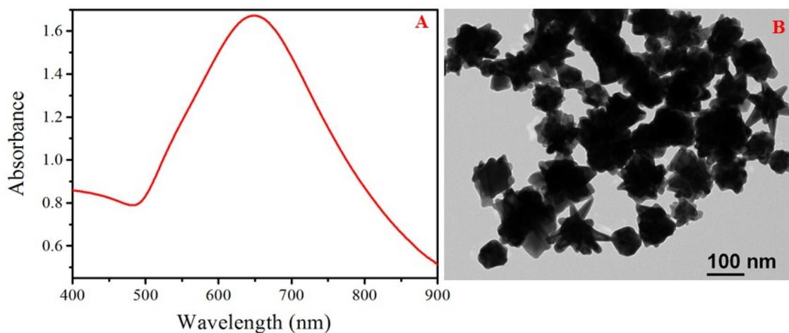
**Figure S1:** (A) Absorption spectra of gold nanostars synthesized by reducing Au(III) with ascorbic acid only (in the absence of TSC, AgNO<sub>3</sub> and NaCl) as a control, and (B) corresponding TEM image of the obtained gold nanostars.
