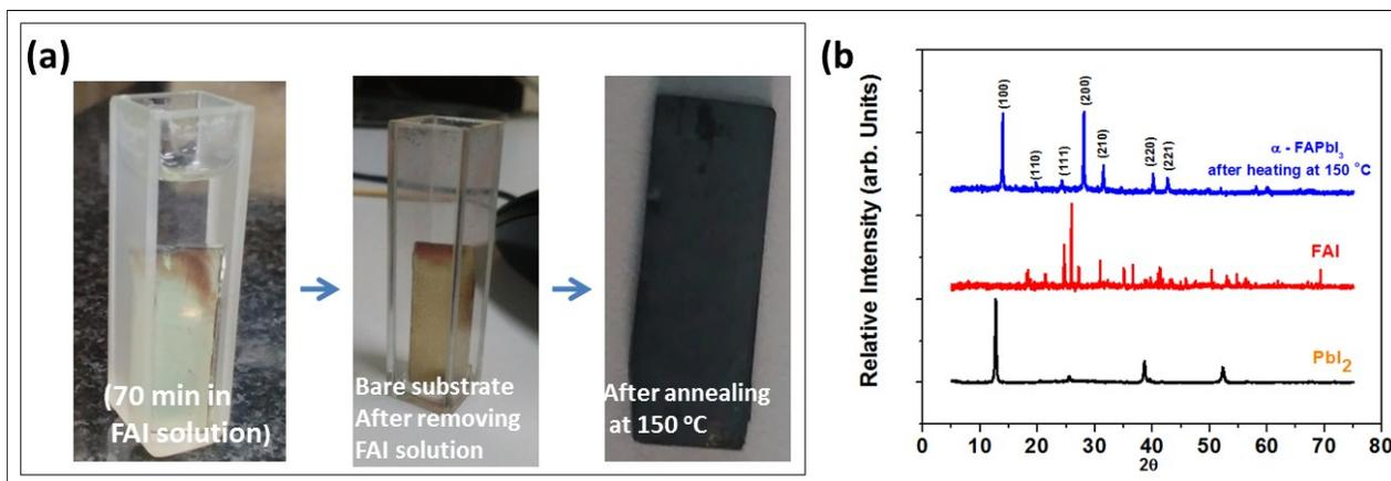
Figure S2 (a) conversion of yellow FAPbI<sub>3</sub> into black FAPbI<sub>3</sub> (b) XRD patterns of PbI<sub>2</sub>, FAPbI<sub>3</sub> and heated FAPbI<sub>3</sub> at 150 °C forming  $\alpha$ -phase.
