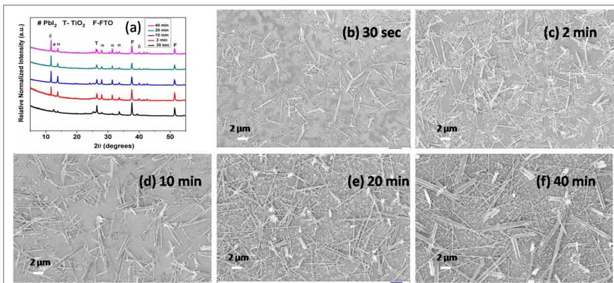
Figure S3. Phase and microstructure information of PbI<sub>2</sub> substrates dipped in FAPbI<sub>3</sub> solution (formula, F2 where antisolvent toluene is replaced with chlorobenzene) (a) XRD of FAPbI<sub>3</sub> formation with dipping time, (b-f) FEG-SEM images of PbI<sub>2</sub> converted into FAPbI<sub>3</sub> with different dipping durations of 30 sec (b), 2 min (c), 10 min (d), 20 min (e) and 40 min (f).
