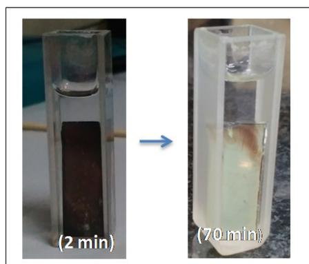
Figure S1. PbI<sub>2</sub> film dipped in FAI solution for 2 min and for 70 min dipping
