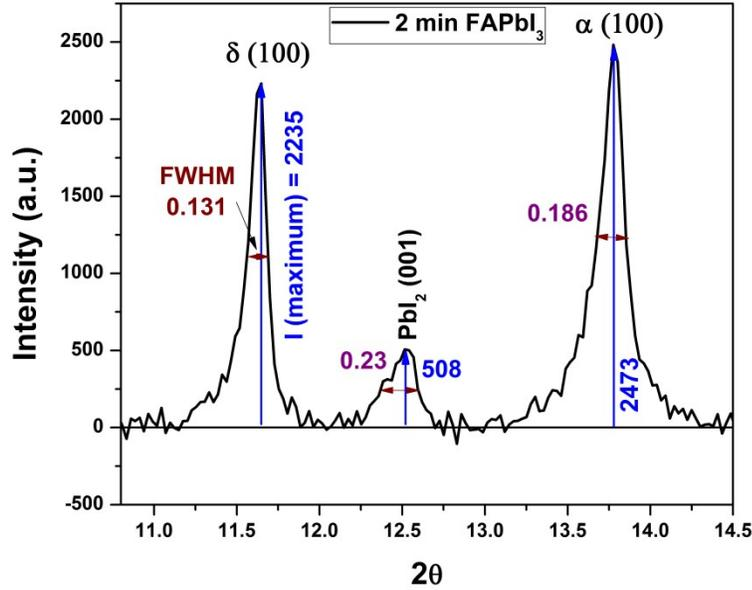
Fig 1 XRD pattern showing characteristic peaks of  $\alpha$  and  $\delta$  of  $\text{FAPbI}_3$  and  $\text{PbI}_2$  for the sample  $\text{PbI}_2$  film dipped in FAI solution for 2 min.
