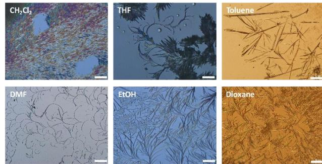
**Figure S3.** Representative bright-field micrographs of **PBDK1** crystals grown from drop-cast solutions of various solvents (5 mg/mL). Scale bar: 100 µm.
