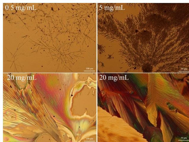
**Figure S6.** Representative bright-field micrographs of **PBDK4** crystals grown from drop-cast acetone solutions of various concentrations at room temperature.
