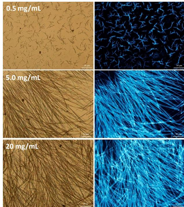
**Figure S5.** Representative bright-field (left) and fluorescence (right) micrographs of **PBDK3** crystals grown from drop-cast acetone solutions of various concentrations at room temperature. Scale bar: 50  $\mu\text{m}$ .
