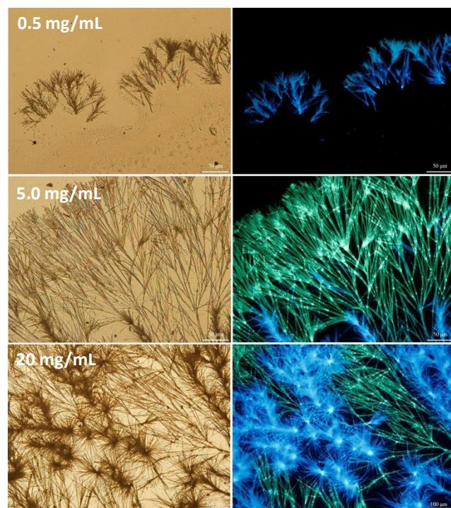
**Figure S4.** Representative bright-field (left) and fluorescence (right) micrographs of **PBDK2** crystals grown from drop-cast acetone solutions of various concentrations at room temperature. Scale bar: 50 µm.
