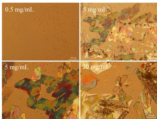
**Figure S7.** Representative bright-field micrographs of **BDK1** crystals grown from drop-cast acetone solutions of various concentrations at room temperature.
