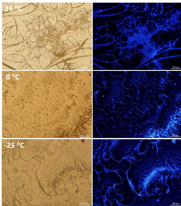
**Figure S2.** Crystal morphologies (left panel: bright field; right panel: fluorescence mode) of **PBDK1** grown from drop-cast acetone solution at 25, 0 and -20 °C (5 mg/mL). Scale bar: 100 µm.
