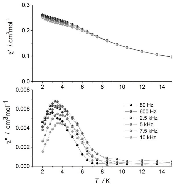
Fig. S21. Temperature dependences of real  $\chi'$  and imaginary  $\chi''$  components of the susceptibility for sample **1** at selected frequencies (measured in zero external *dc* field for exciting field of 3 Oe).
