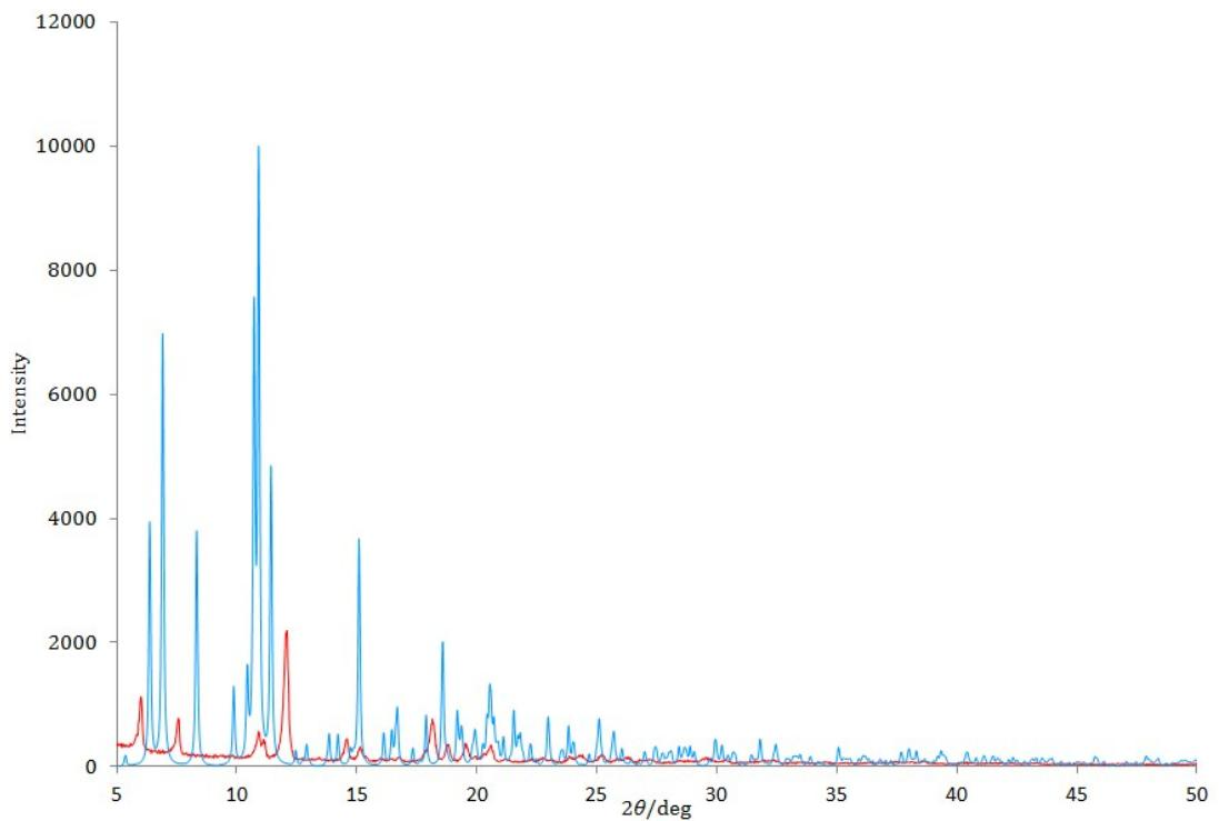
Fig. S11. The powder X-ray pattern of complex 2: measured – red line; the simulated pattern of complex 2 derived from single crystal data – blue line.
