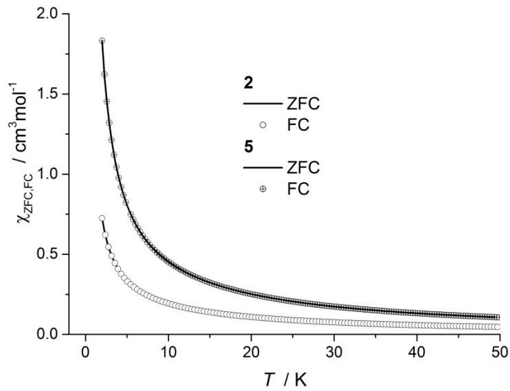
Fig. S22. Temperature dependences of  $\chi_{ZFC}$  and  $\chi_{FC}$  magnetic susceptibility measured in  $H = 1$  kOe for **2** and **5**.
