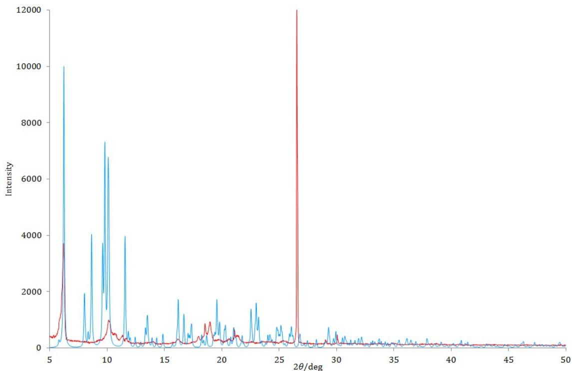
Fig. S13. The powder X-ray pattern of complex 4: measured – red line; the simulated pattern of complex 4 derived from single crystal data – blue line.
