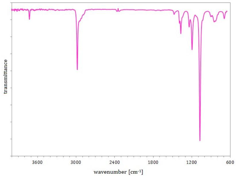
Fig. S24. FTIR spectrum of the volatiles evolving during TG analysis of **5** recorded at  $240\text{ }^{\circ}\text{C}$ .
