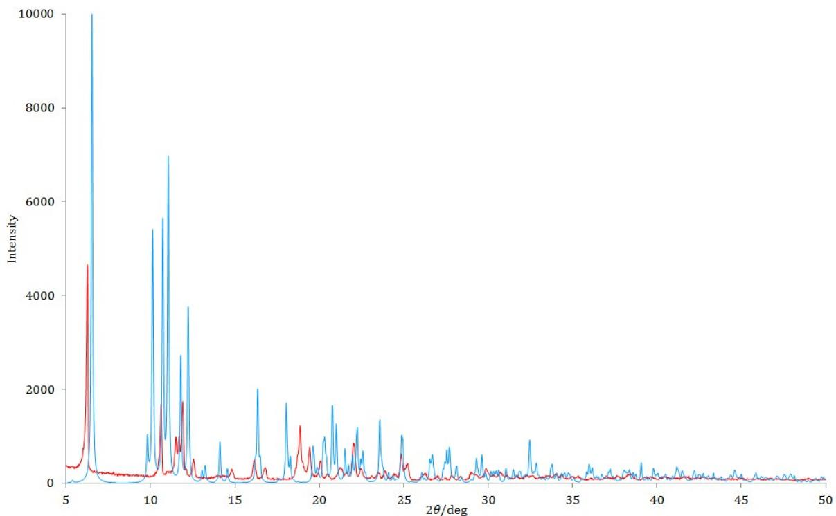
Fig. S12. The powder X-ray pattern of complex 3: measured – red line; the simulated pattern of complex 3 derived from single crystal data – blue line.
