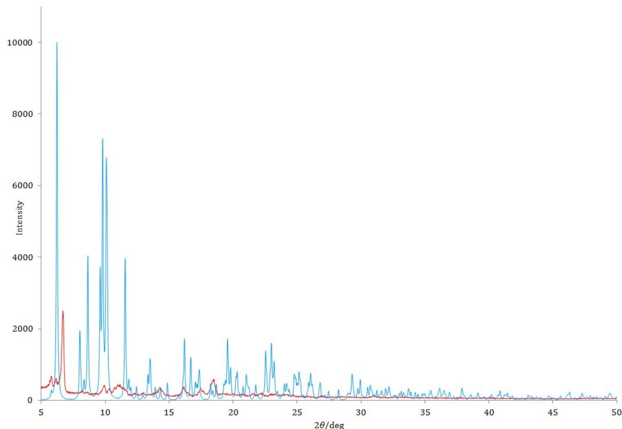
Fig. S14. The powder X-ray pattern of complex 5: measured – red line; the simulated pattern of complex 5 derived from single crystal data – blue line.
