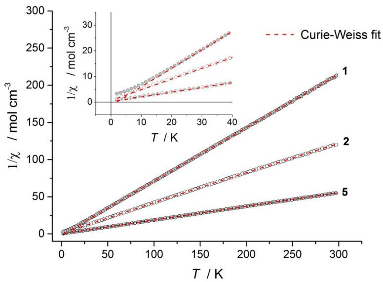
Fig. S17. Reciprocal molar susceptibility ( $1/\chi$ ) versus temperature for **1**, **2** and **5**. Dashed lines are the best Curie-Weiss fit to the data (see text); the inset shows a magnification of the low temperature range.
