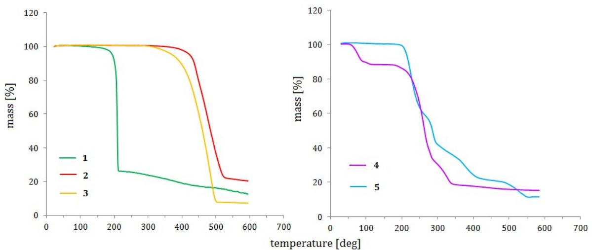
Fig. S23. Thermogravimetric curves of 1-5 obtained at a heating rate of  $10\text{ K min}^{-1}$ .
