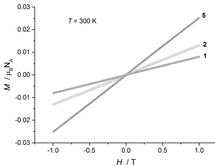
Fig. S18. Magnetization curves for samples **1**, **2** and **5** measured at 300 K.
