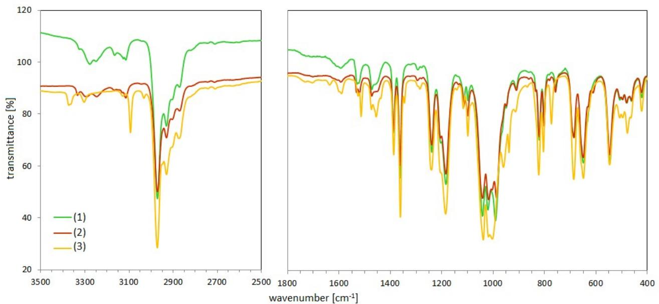
Fig. S15. FTIR spectrum of complex **1-3** in the range of 4000-400 cm<sup>-1</sup>.
