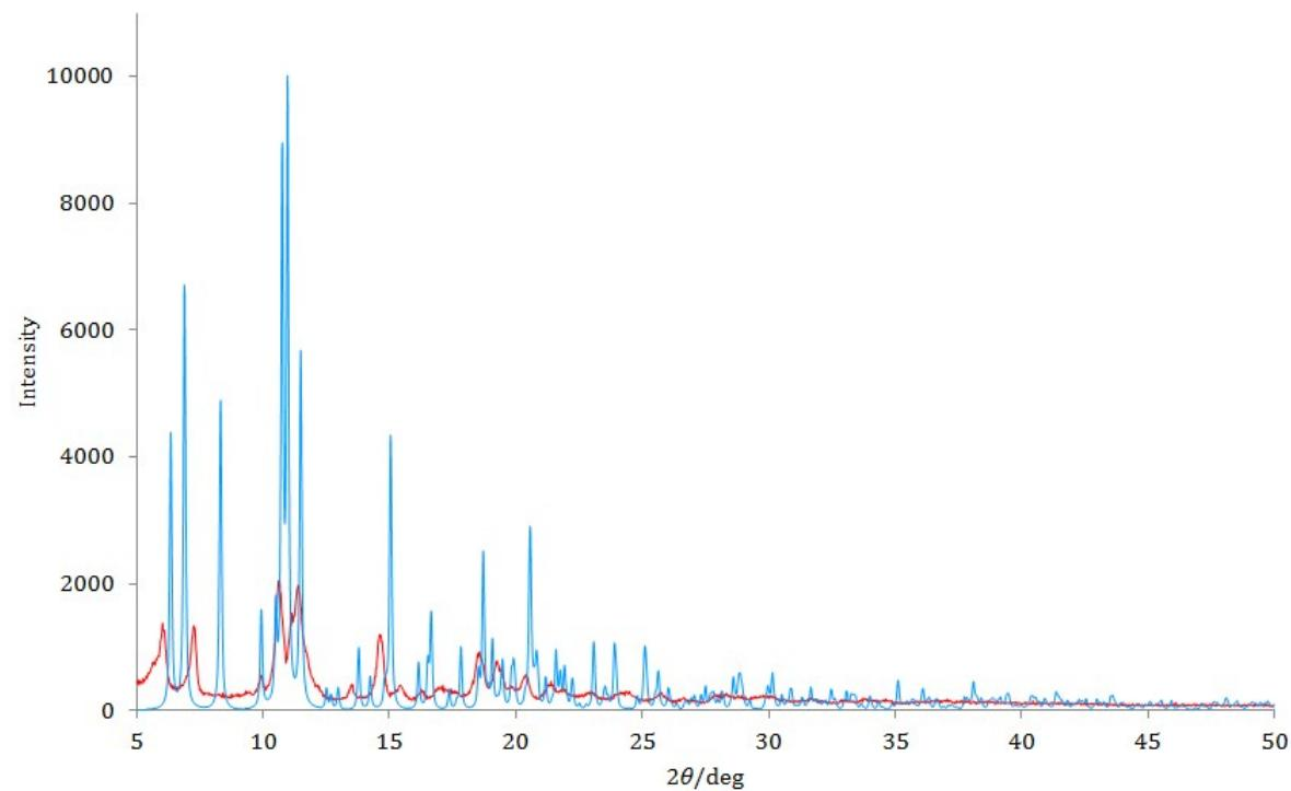
Fig. S10. The powder X-ray pattern of complex **1**: measured – red line; the simulated pattern of complex **1** derived from single crystal data – blue line.
