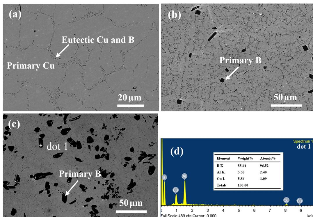
Figure S1. Typical microstructure and of Cu-B alloys cooled at a cooling rate of about 20K/s. (a) Cu-1wt.%B; (b) Cu-2.5wt.%B; (c) Cu-4wt.%B; (d) EDX analysis of dot 1 in Fig.2(c);
